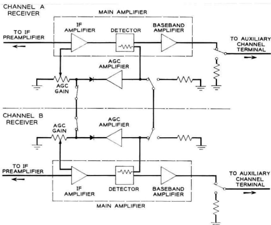
Fig. 7 — Block diagram showing interconnection of AGC circuits.
