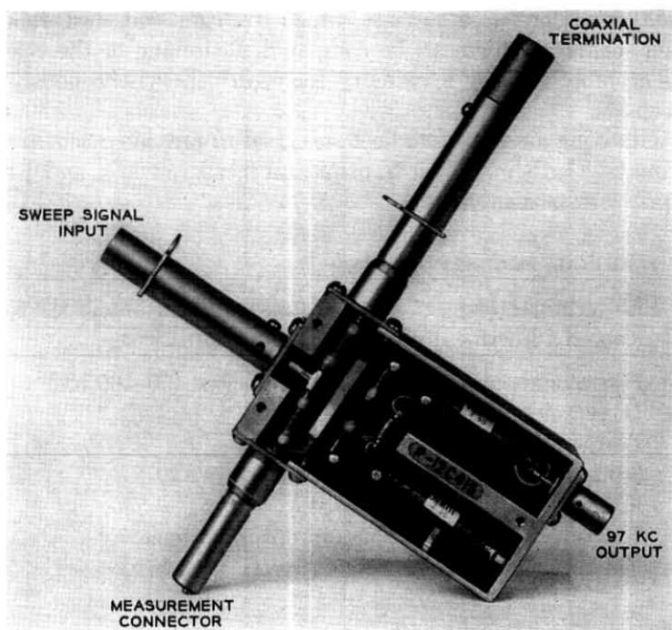
Fig. 8 — The IF reflectometer.
