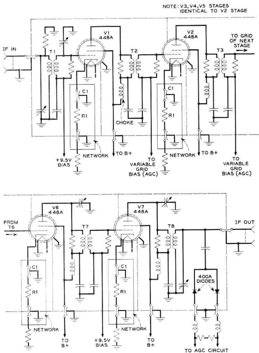
Fig. 10 — Simplified schematic of the IF main amplifier.
