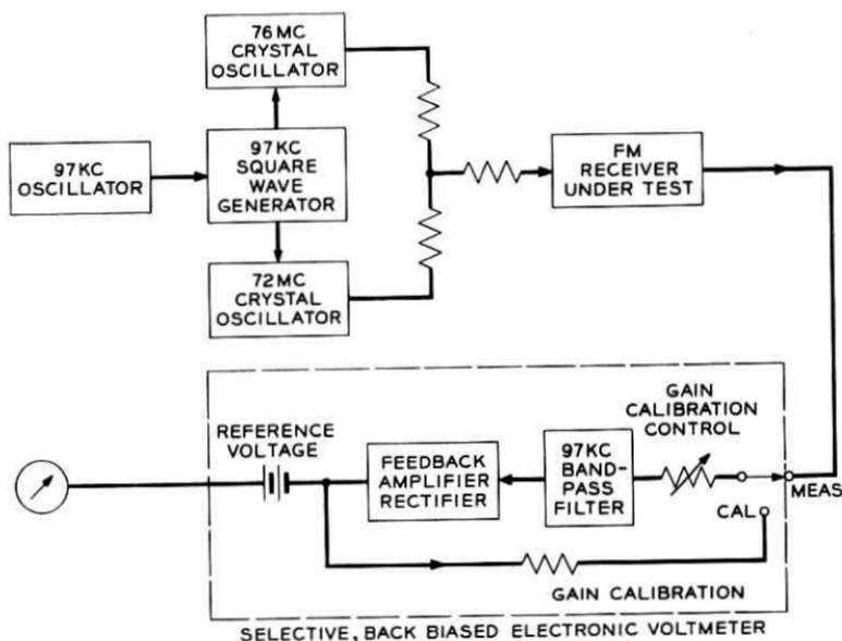
Fig. 12 — Block diagram for FM deviation sensitivity measurement.
