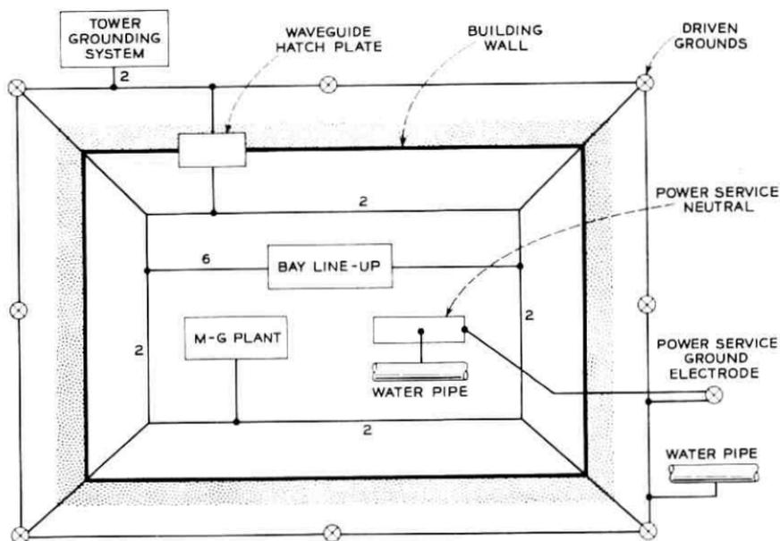
Fig. 12 — Arrangement of the basic building grounding system.
