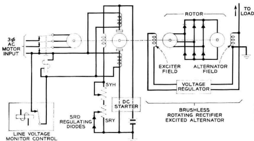
Fig. 2 — Circuit of the two-motor alternator set.
