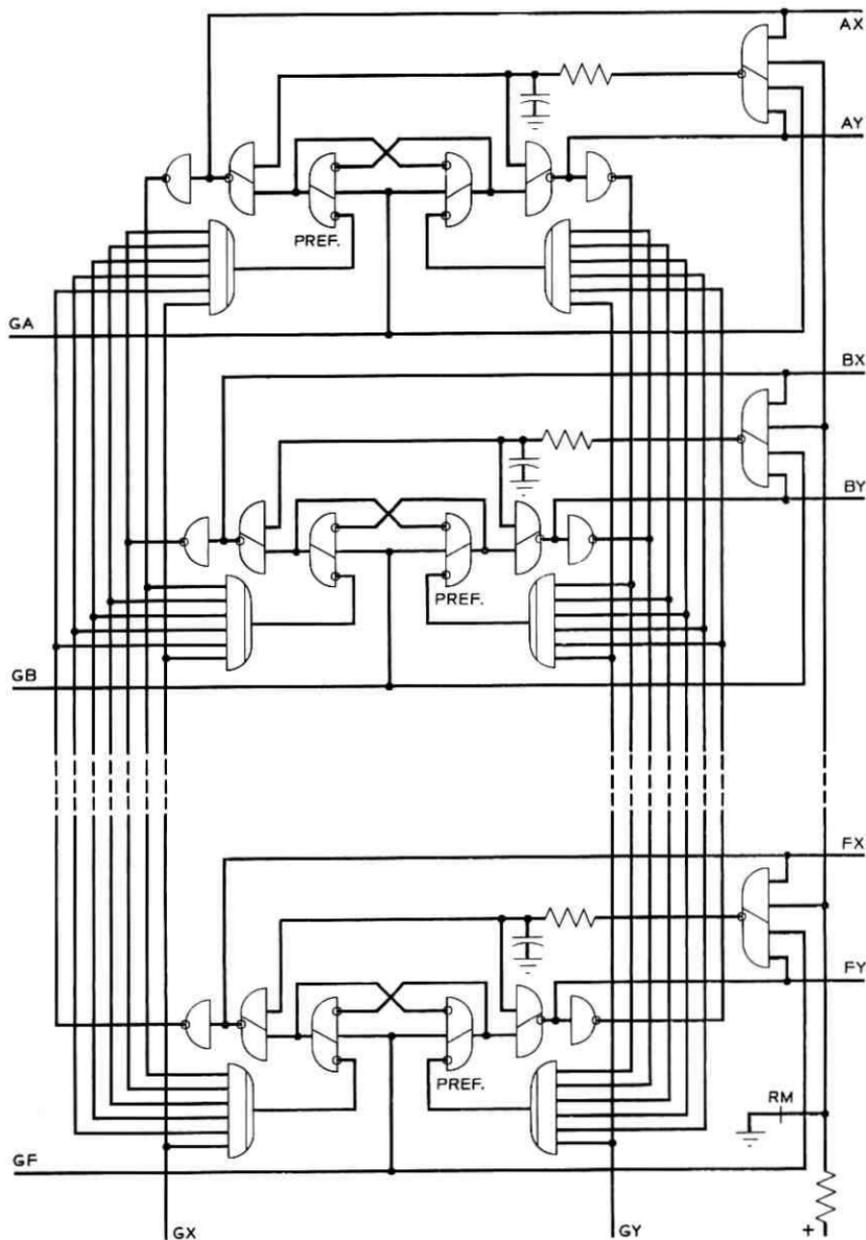
Fig. 24 — Logic diagram of the assignment circuit.
