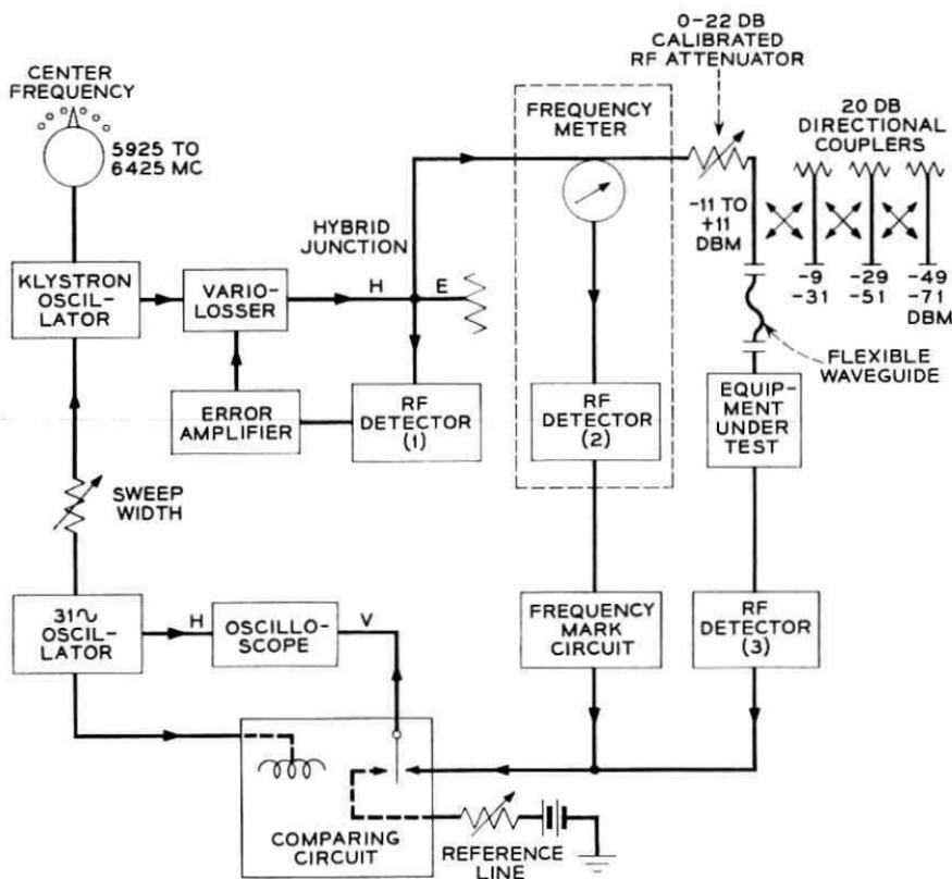
Fig. 1 — Block diagram for RF transmission measurements.
