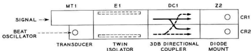
Fig. 4 — Simplified block schematic of the receiver modulator.
