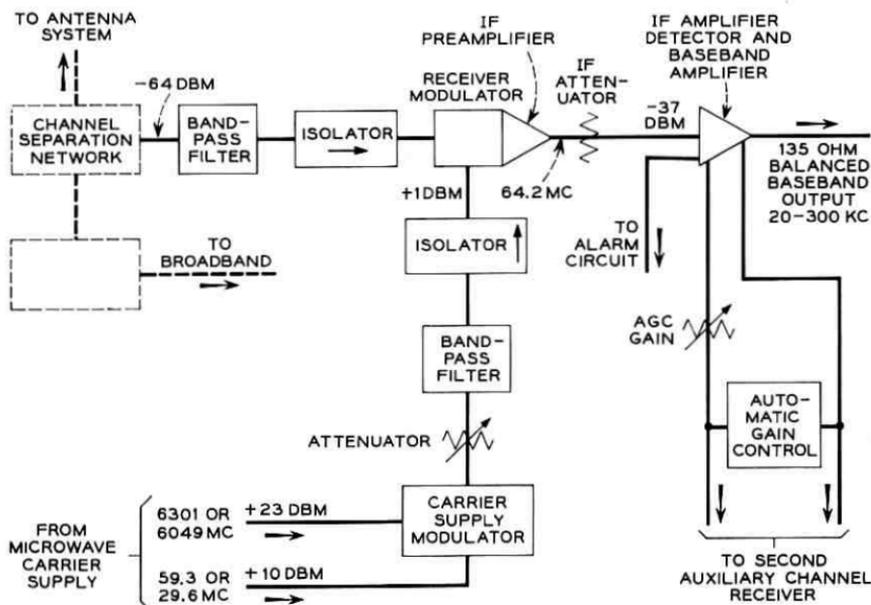
Fig. 6 — Block diagram of the auxiliary channel receiver.
