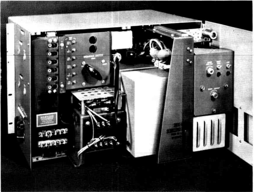
Fig. 10 — High-voltage power supply with various equipment units partially removed.
