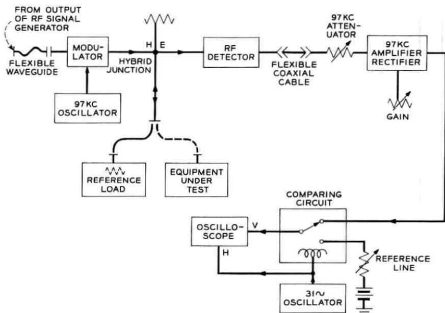
Fig. 2 — Block diagram for RF reflection coefficient measurements.
