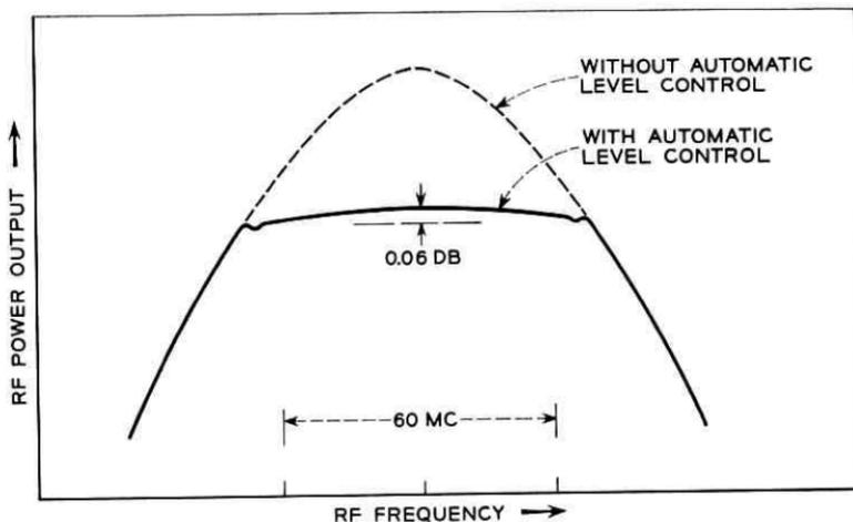
Fig. 4 — Action of the automatic level control.
