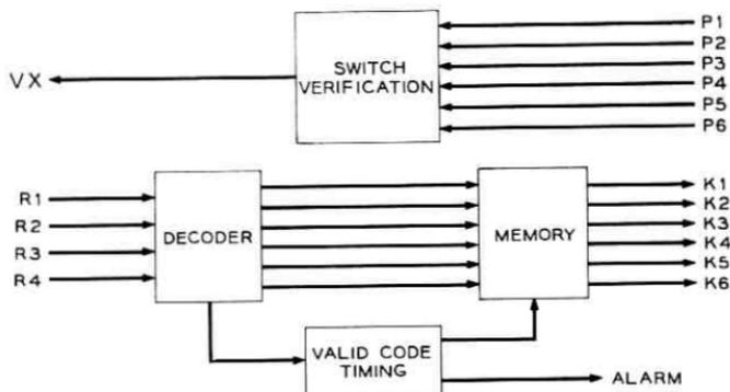
Fig. 15 — Block diagram of receiving logic.
