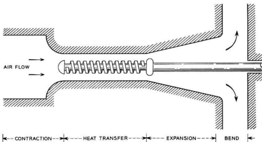
Fig. 35 — Cross section of the collector cooling chamber.
