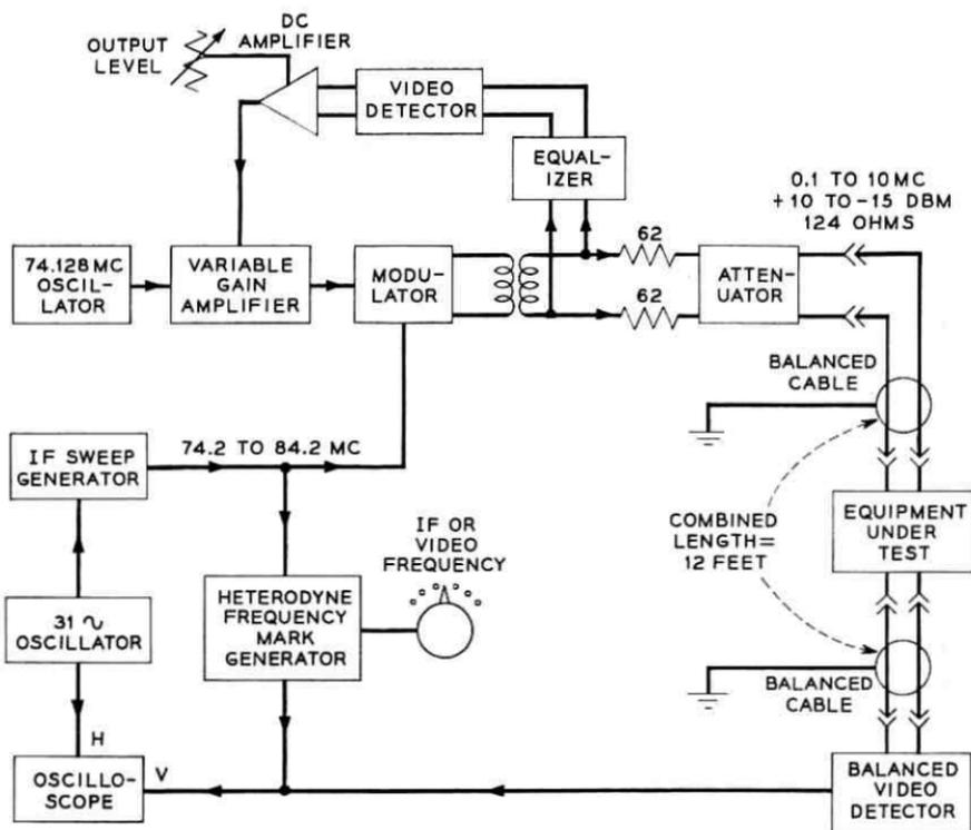
Fig. 10 — Block diagram for video transmission measurements.
