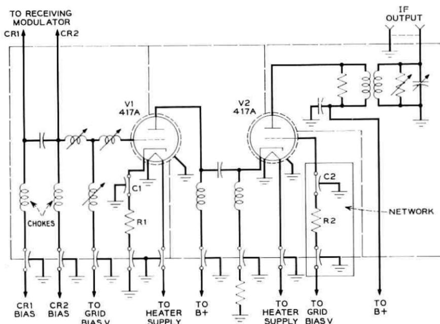
Fig. 6 — Simplified schematic of the IF preamplifier.
