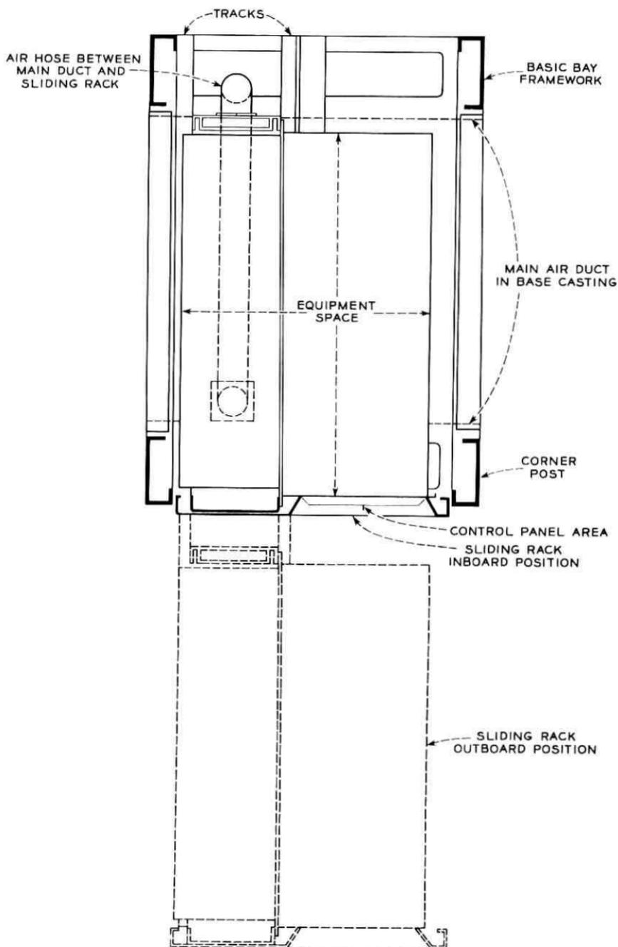
Fig. 4 — Plan view of sliding-rack bay framework.
