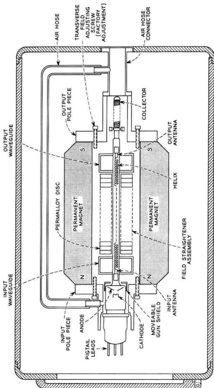
Fig. 25 — Cross section of traveling-wave tube amplifier.
