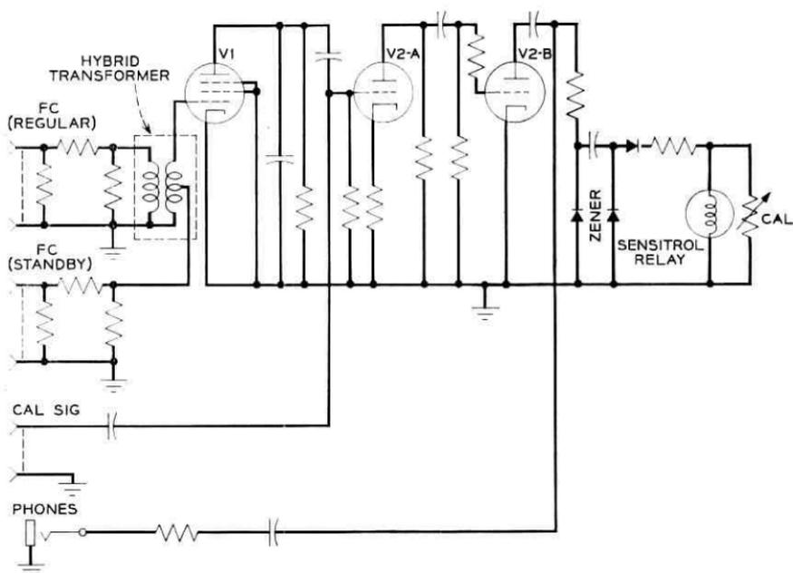
Fig. 4 — Simplified schematic of the frequency comparator.
