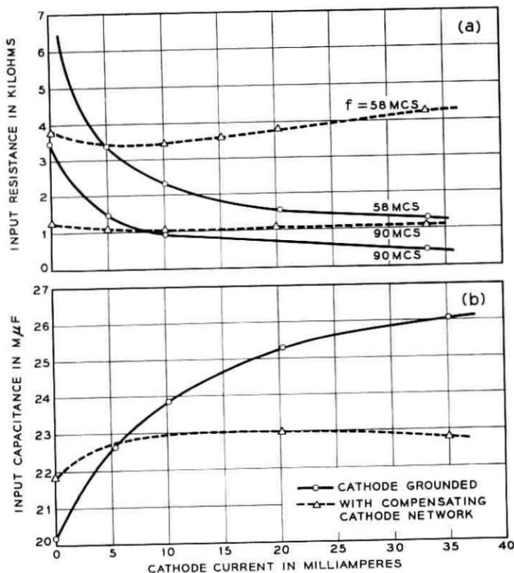
Fig. 11 — Input impedance of the W.E. 448A tetrode.
