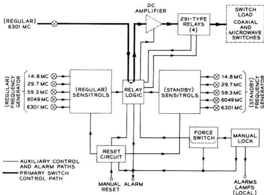
Fig. 11 — Functional diagram of the switching control.
