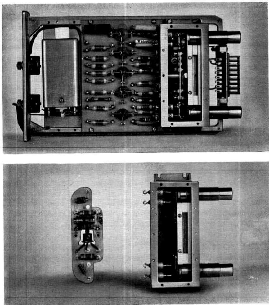
Fig. 15 — Views of an IF level detector unit.
