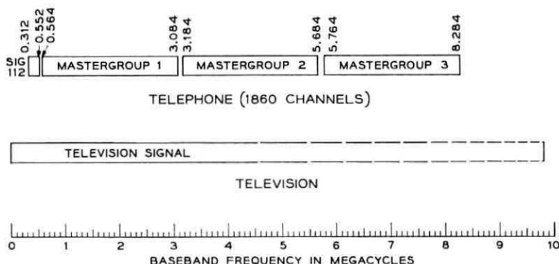
Fig. 3 — The baseband signals of the TH system.
