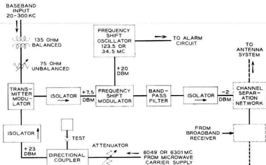
Fig. 3 — Block diagram of auxiliary channel transmitter.
