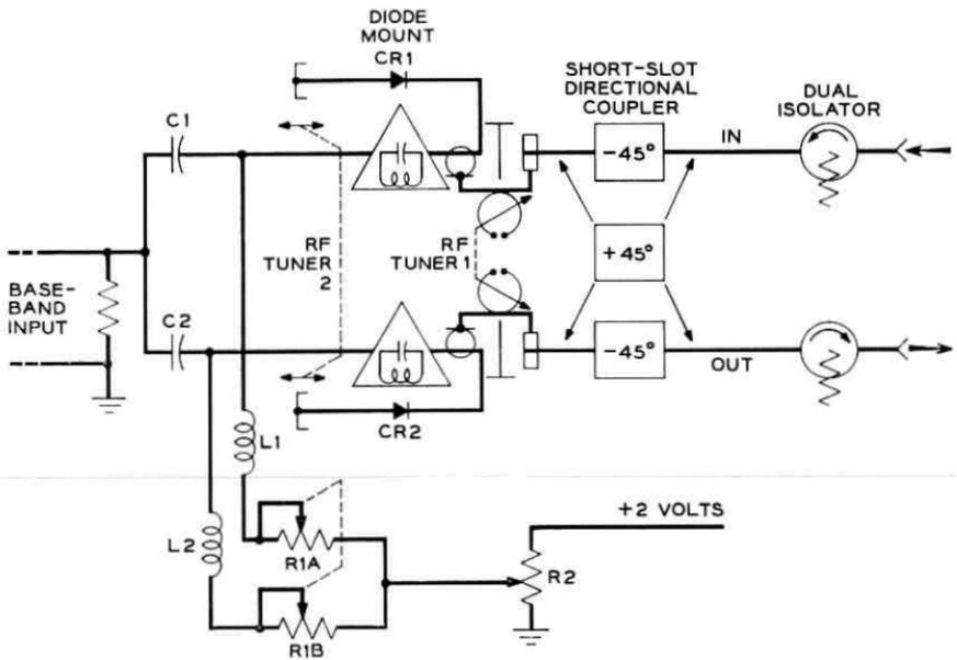
Fig. 5 — Simplified schematic of the transmitter modulator.
