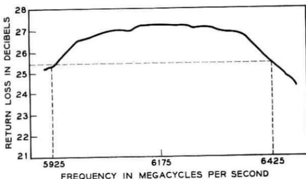
Fig. 34 — Return loss of typical transducer.
