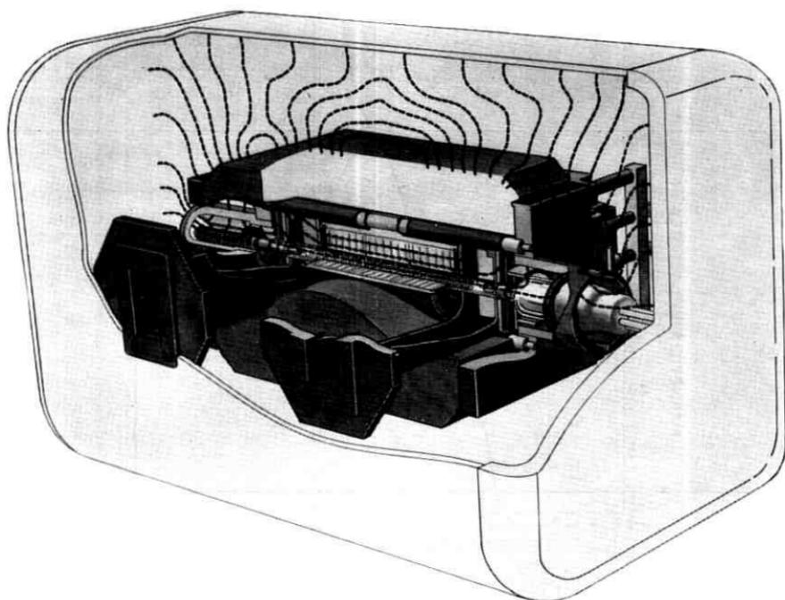
Fig. 30 — Magnetic assembly of the traveling-wave tube amplifier.
