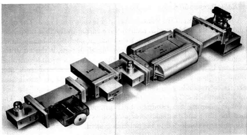
Fig. 4 — Modulator of auxiliary channel transmitter.
