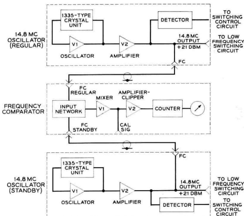
Fig. 3 — Block diagram of the 14.8-mc supply circuit.
