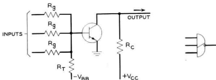
Fig. 16 — Basic TRL gate and symbol.
