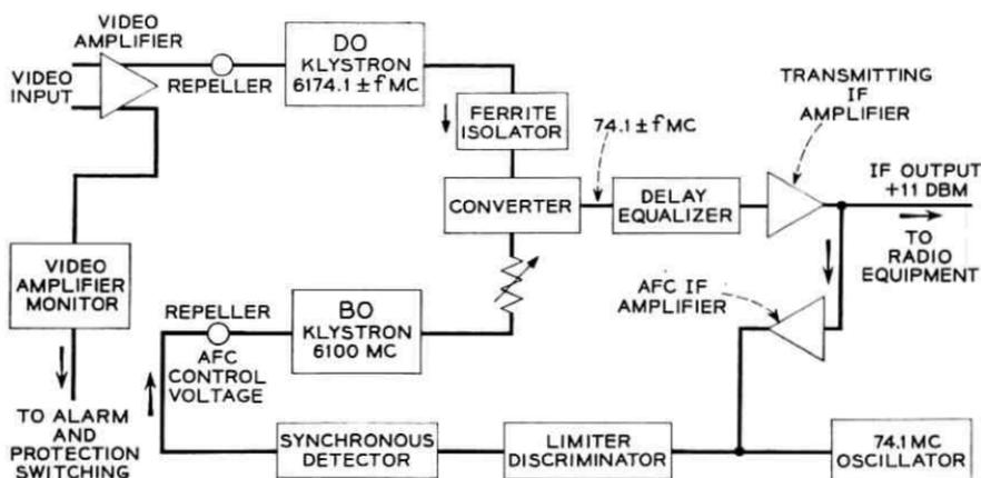
Fig. 2 — Block diagram of FM transmitter.
