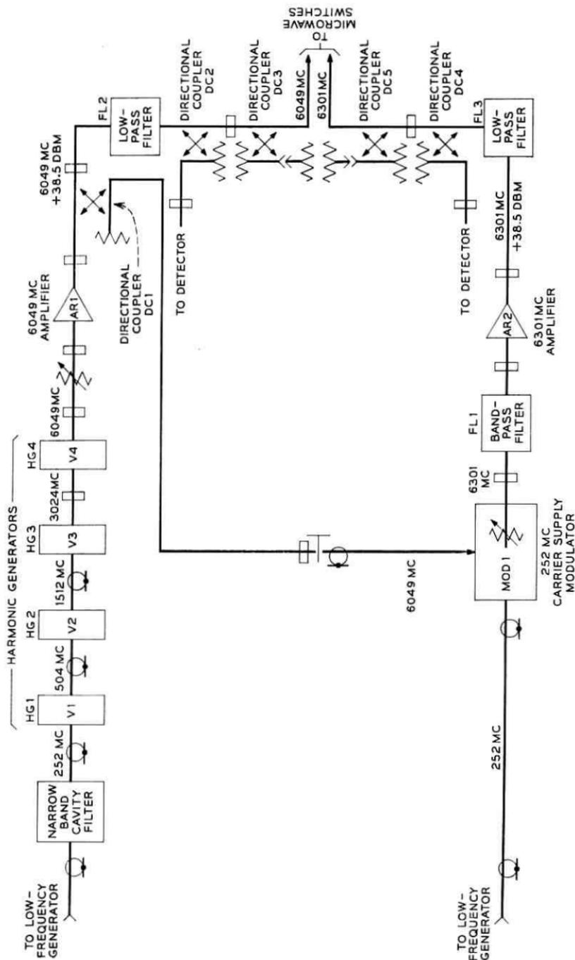
Fig. 6 — Block diagram of the high-frequency generator.
