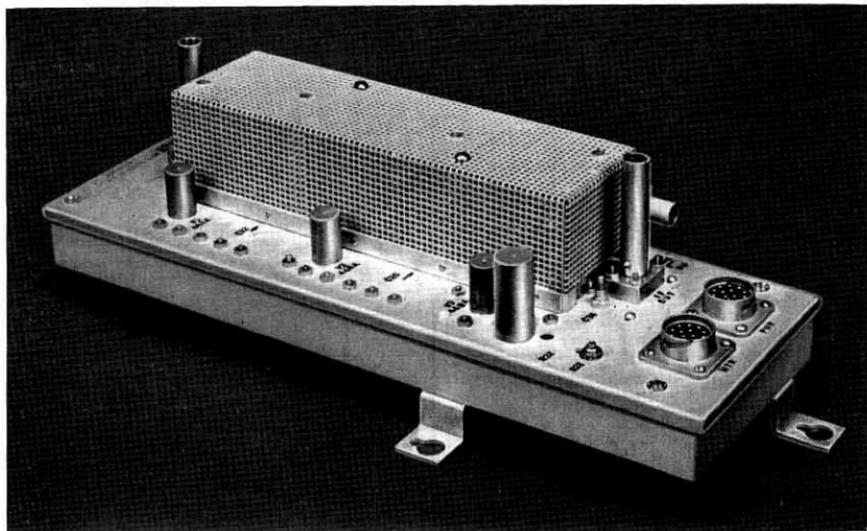
Fig. 16 — The IF amplifier-limiter.
