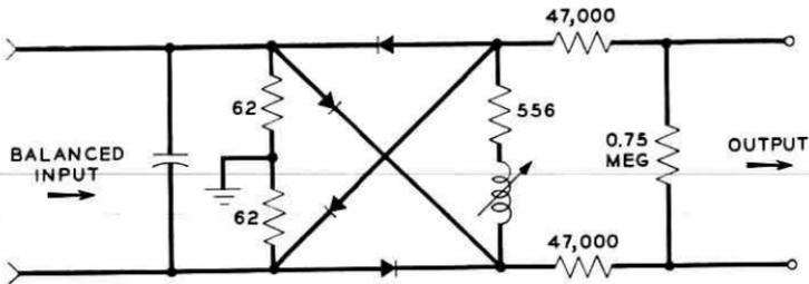
Fig. 11 — Circuit of the balanced video detector.
