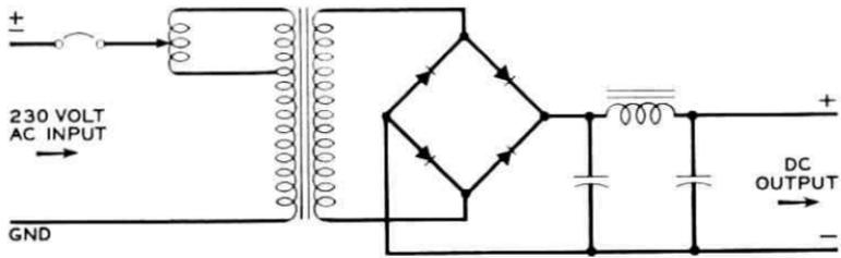
Fig. 4 — Typical circuit of adjustable, unregulated rectifier.
