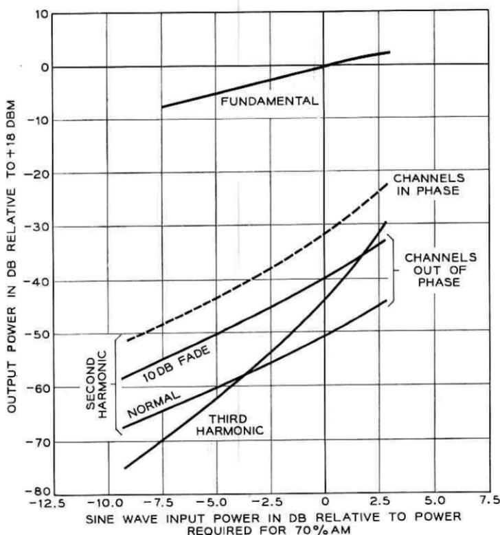
Fig. 10 — Typical modulation performance of a one-hop system.
