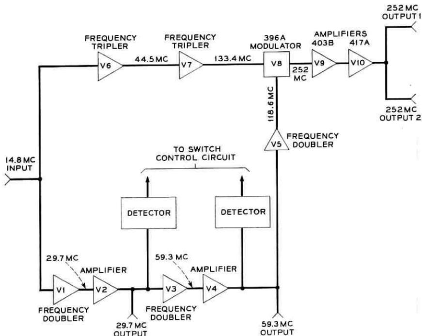
Fig. 5 — Block diagram of the low-frequency generator.
