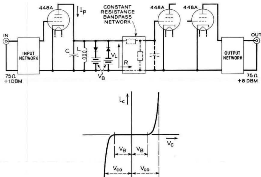
Fig. 15 — Simplified schematic of the IF amplifier-limiter, with typical voltage-current dc clipping characteristic.
