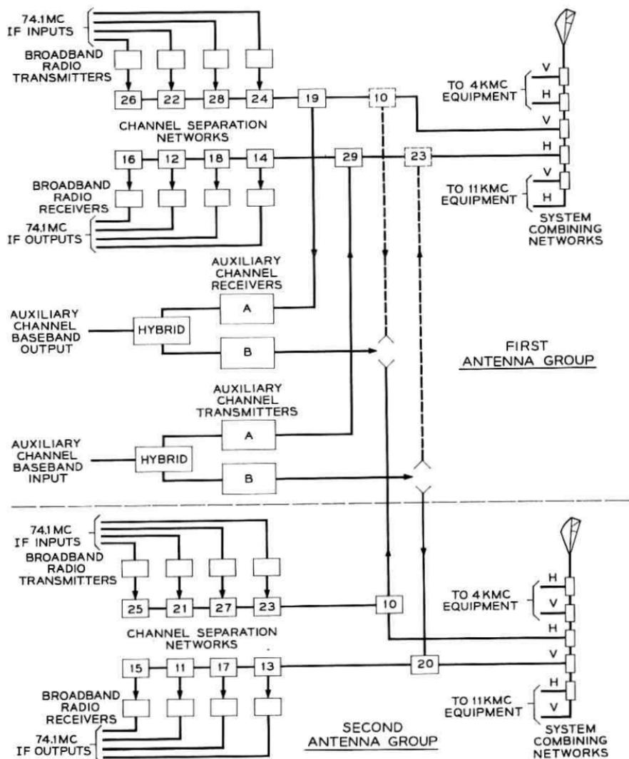
Fig. 4 — Diagram of antenna connections.
