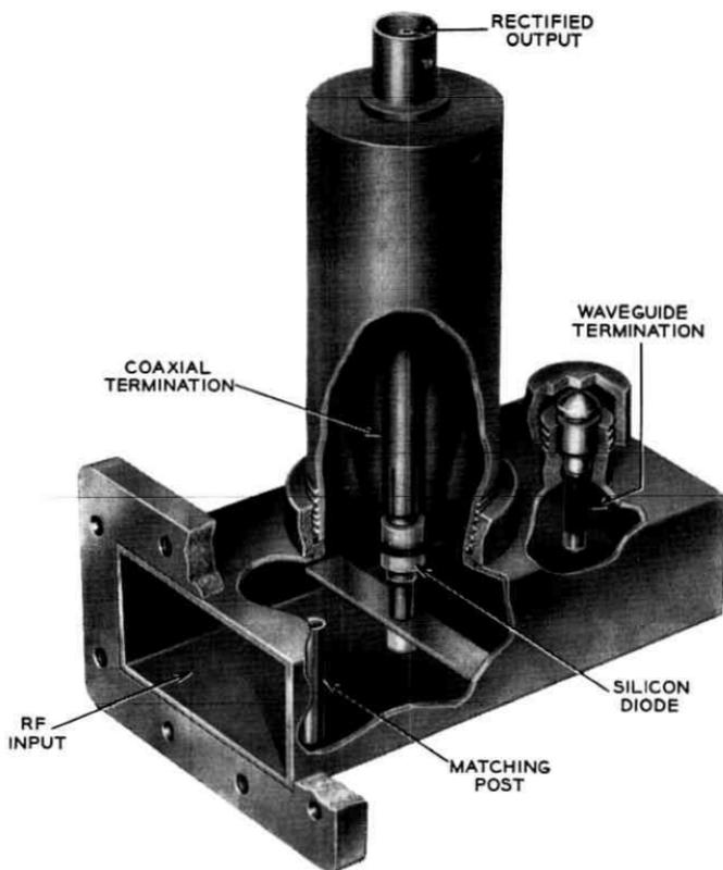
Fig. 5 — Internal configuration of the RF detector.
