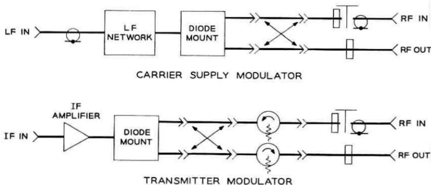
Fig. 22 — Schematics of the two types of modulators.
