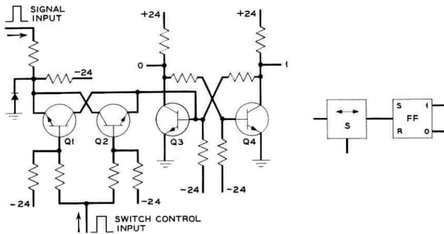
Fig. 19 — Bi-lateral switch and special flip-flop with symbols.
