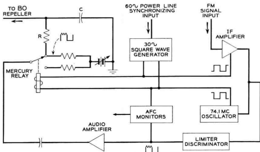
Fig. 4 — Functional schematic of the AFC system.
