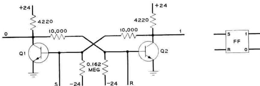
Fig. 18 — Standard flip-flop circuit and representation.
