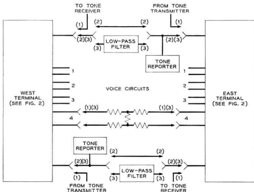
Fig. 8 — Simplified block diagram showing special terminal interconnections.
