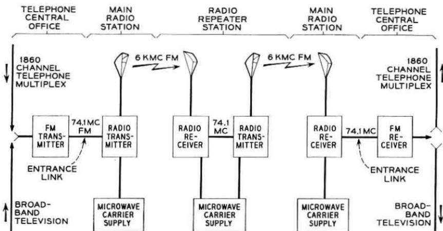
Fig. 1 — Block diagram of the TH system.
