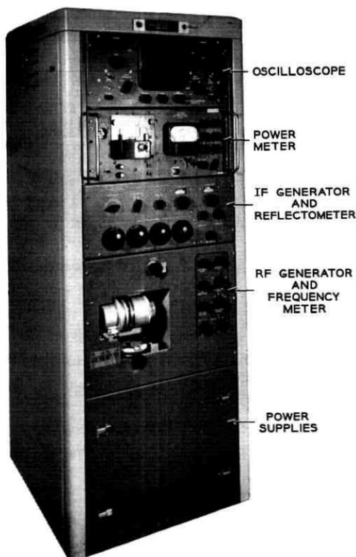
Fig. 3 — Front view of the transmitter-receiver test set.
