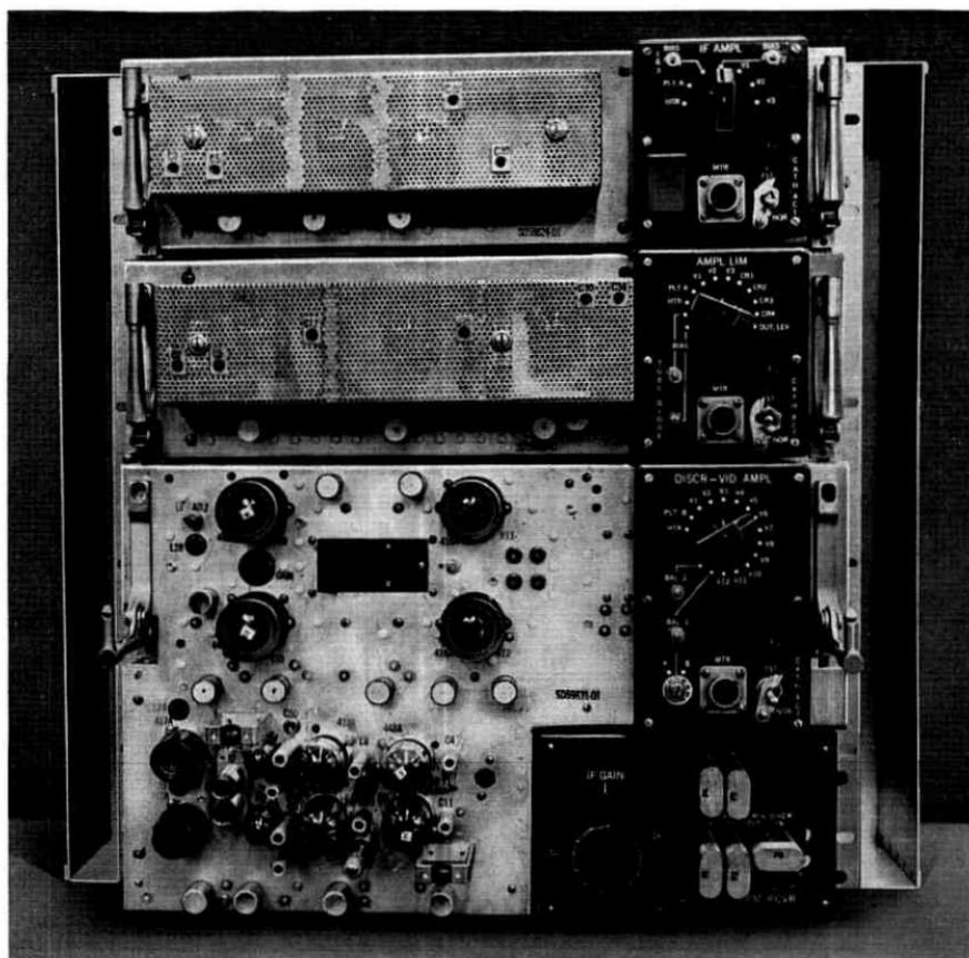
Fig. 6 — The FM terminal receiver.
