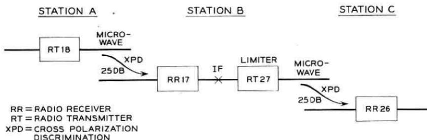
FIG. 11 — Basic mechanism of tertiary interference.
