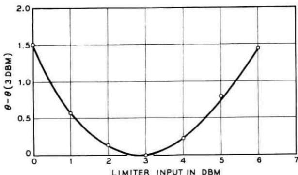
Fig. 18 — AM to PM conversion at 74 mc as a function of limiter input power.
