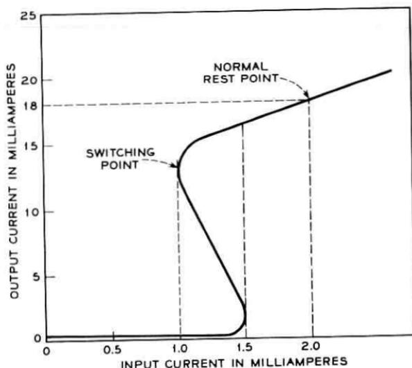
Fig. 12 — Typical transfer characteristic of the magnetic amplifier
