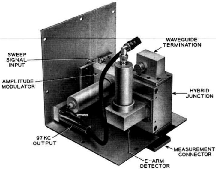
Fig. 7 — Waveguide components of the RF reflectometer.
