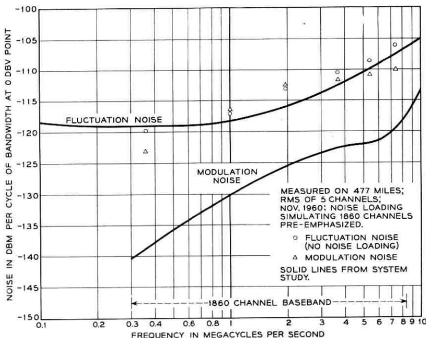
FIG. 7 — Modulation and fluctuation noise for 4000 miles of TH radio, as calculated in system study and as extrapolated from field measurements.
