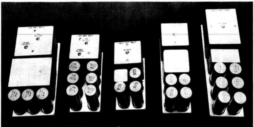
Fig. 5 — Rectifier packages showing family resemblance of designs.
