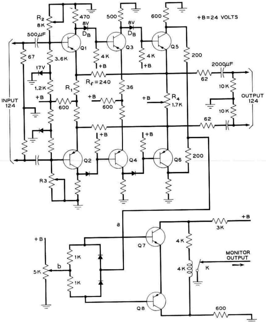
Fig. 10 — Simplified schematic of baseband amplifier.
