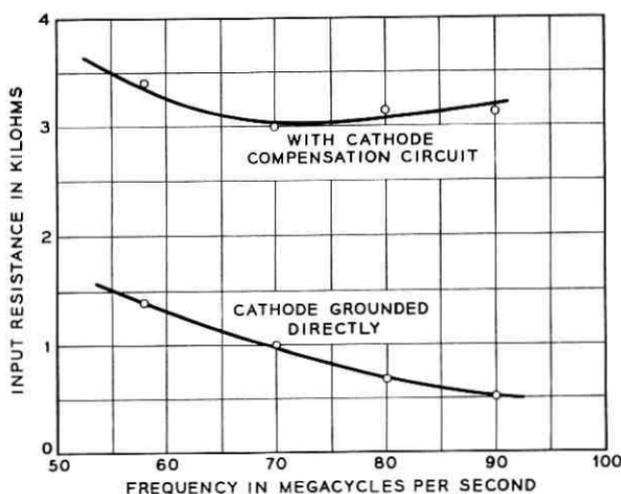
Fig. 7 — Input resistance of a W.E. 417A triode: cathode grounded directly and with cathode compensation circuit.
