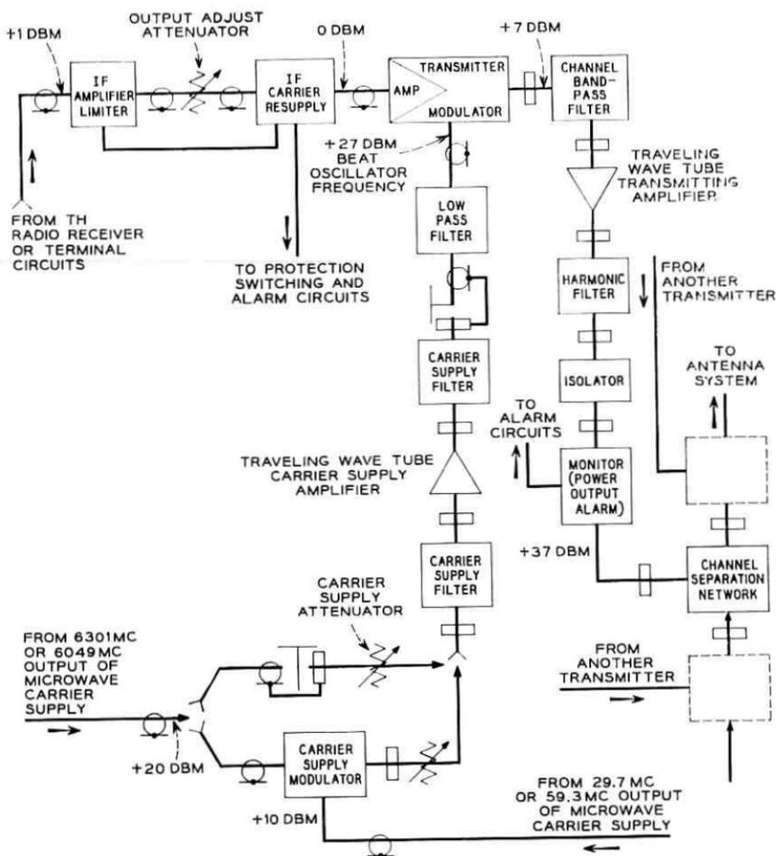
Fig. 13 — Block schematic of the TH radio transmitter.
