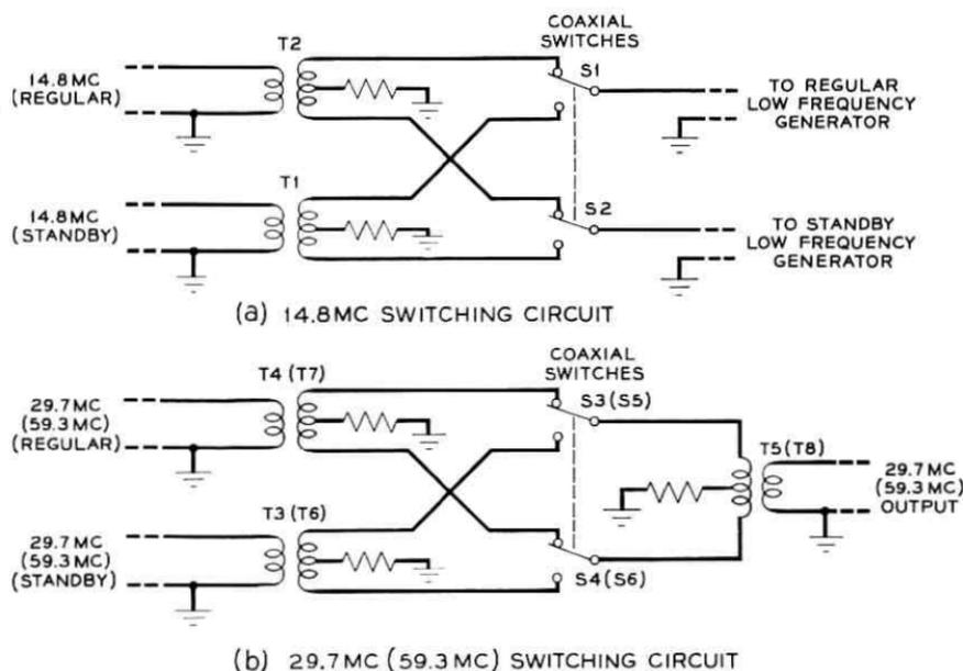
Fig. 8 — Simplified schematic of the low-frequency switching circuit.
