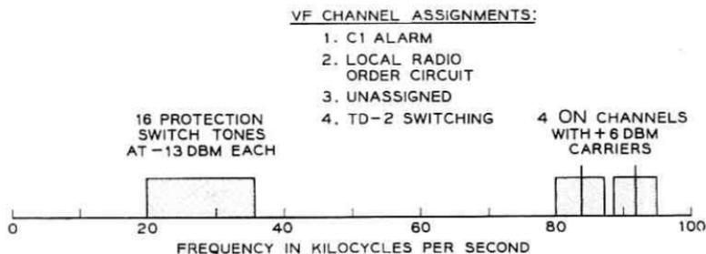
Fig. 1 — Baseband signal spectrum for auxiliary radio channels.
