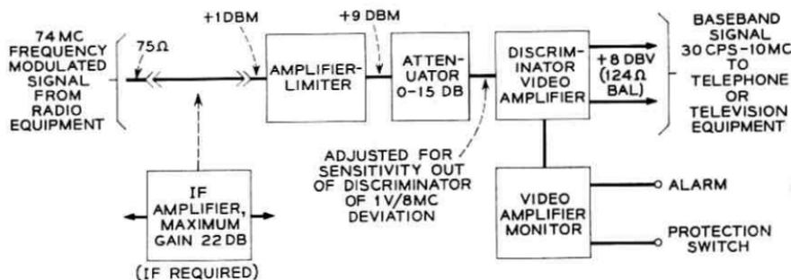
Fig. 5 — Block diagram of FM receiver.
