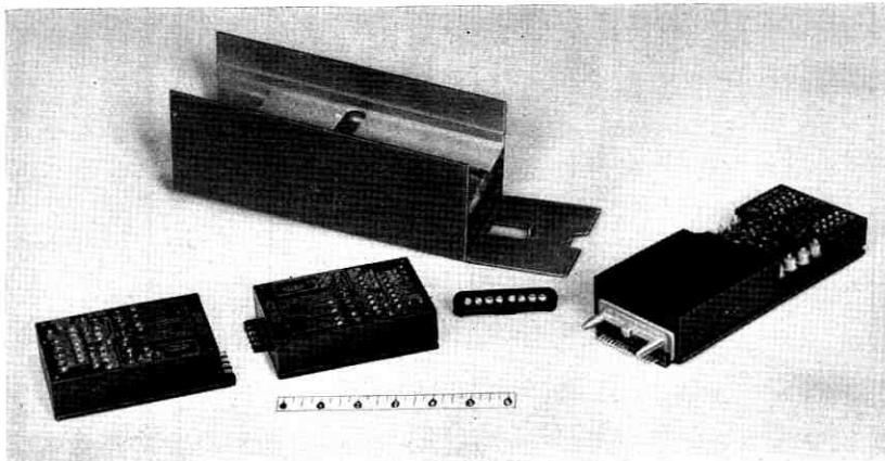
Fig. 38 — Exploded view of complete E6 repeater.
