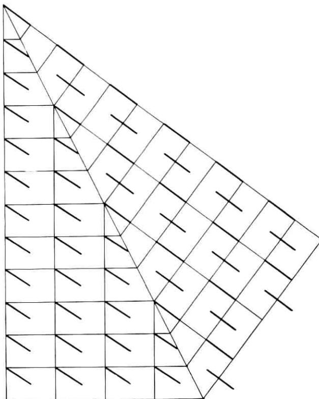
Fig. 19 —  $(110)[010]:(310):(200)[\frac{1}{2}\frac{1}{2}0]$  phase boundary in  $(310)$  twin.
