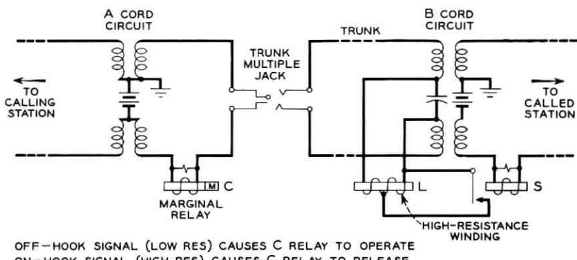
Fig. 2 — High-low signaling.
