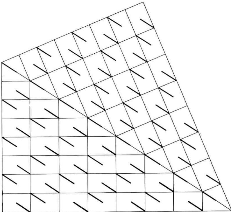
Fig. 14 —  $(110)[\frac{1}{2}\frac{1}{2}0]:(110):(110)[\frac{1}{2}\frac{1}{2}0]$  domain boundary in (110) twin.
