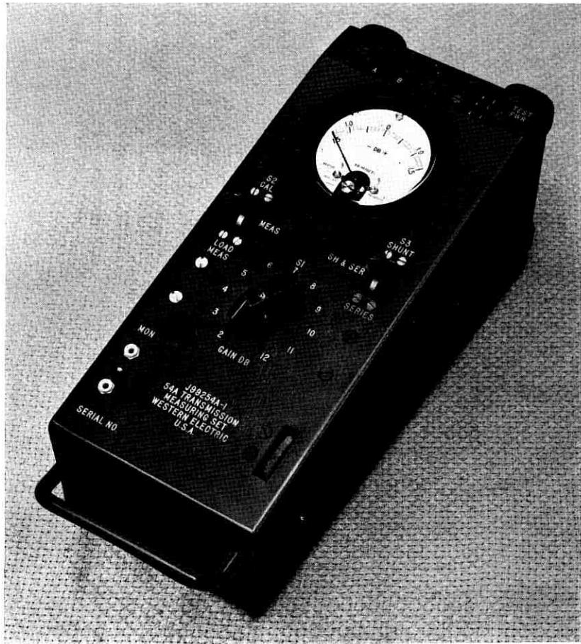
Fig. 40 — 54A transmission measuring set.
