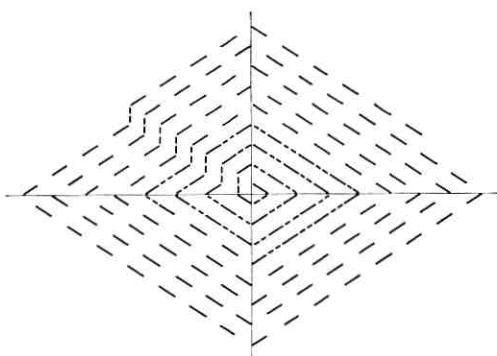
Fig. 25 — Single-spiral crystal containing  $(110)[\frac{1}{2}\bar{1}0]$ -type domains. One  $(200)$  fold is required in every loop to maintain the stacking sequence.
