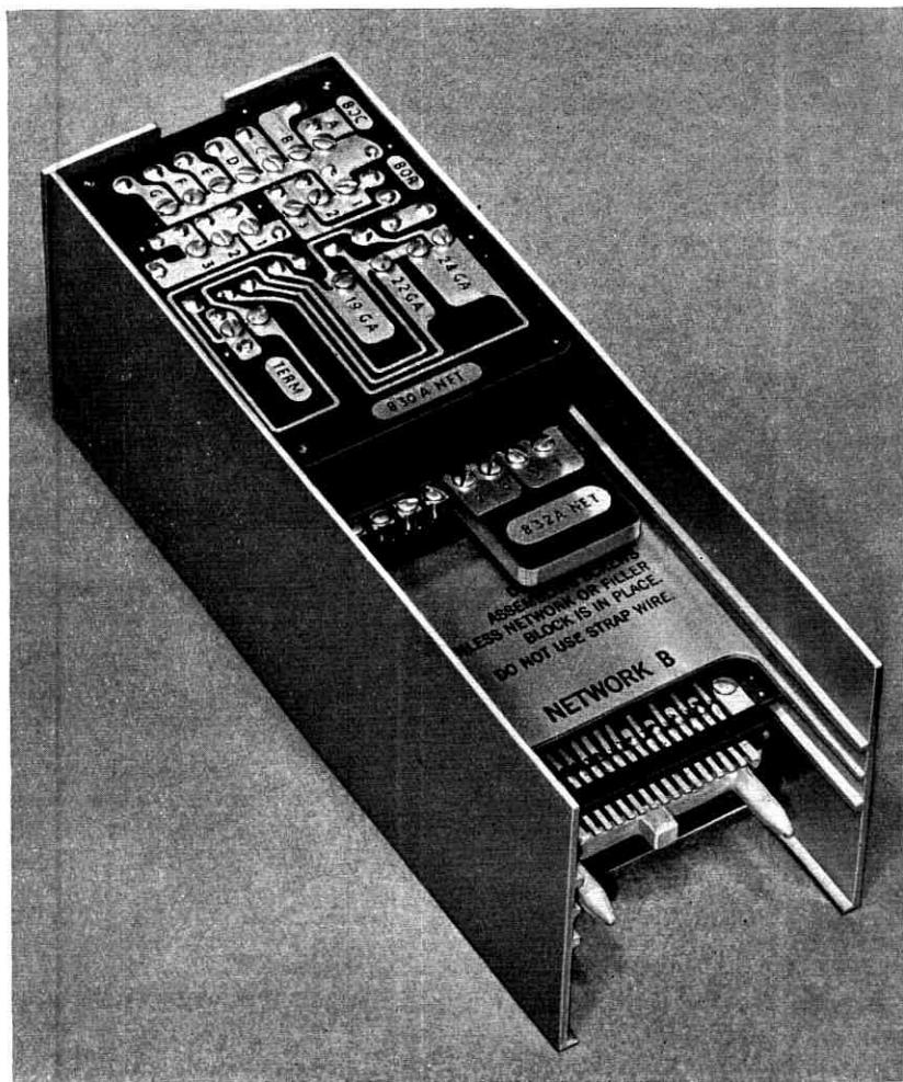
Fig. 39 — The E6 repeater — arranged for terminal use.
