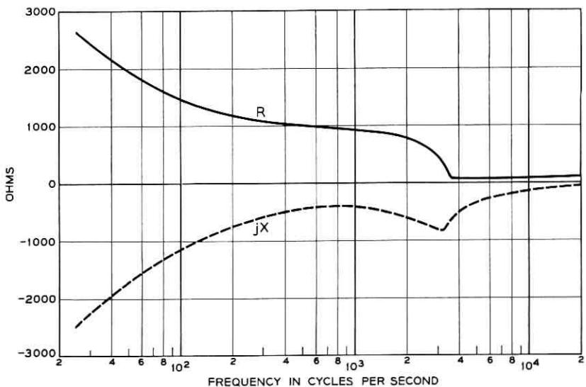
Fig. 27—Characteristic impedance of full-section H-88 loaded cable.
