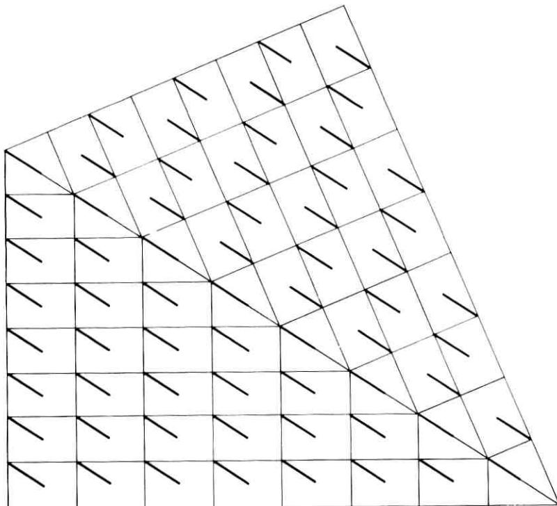
Fig. 15 —  $(110)[010]:(110):(110)[\frac{1}{2}\frac{1}{2}0]$  phase boundary in  $(110)$  twin.
