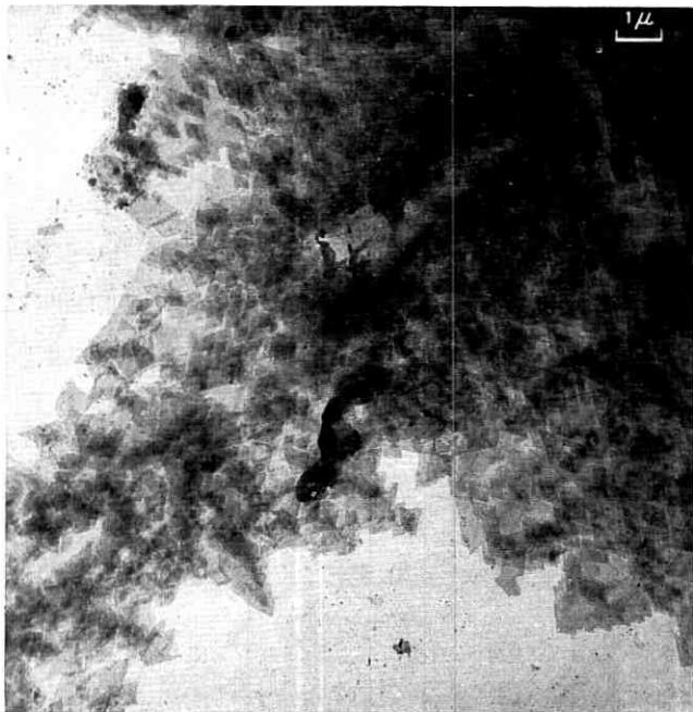
Fig. 2 — Bright-field micrograph of crystals twinned across (530) plane.
