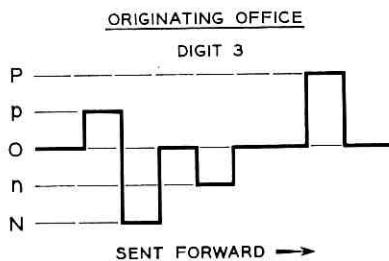
Fig. 13 — PCI pulsing.
