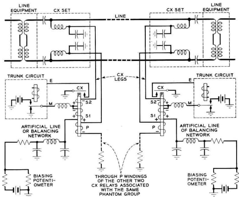
Fig. 8 — Composite signaling circuit for one-voice channel.
