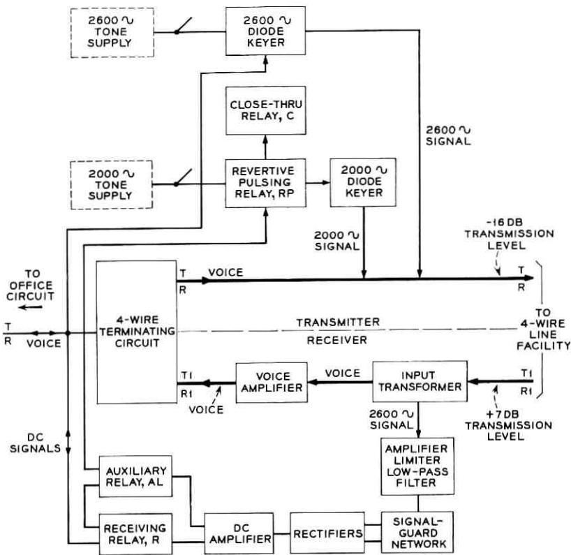
Fig. 21 — Basic elements of SF signaling unit — terminating terminal revertive pulsing.
