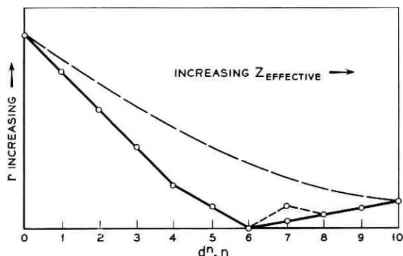
Fig. 7 — Variation of "ionic radius" with effective nuclear charge for medium-strong spin-orbit coupled octahedral complexes. The configurations  $d^n$ , ( $n = 0, 4, 5, 6, 7, 10$ ) are states of perfect cubic ("pseudo spherical") symmetry. The states  $d^3$  and  $d^8$  are but slightly asymmetric due to their spin distributions.
