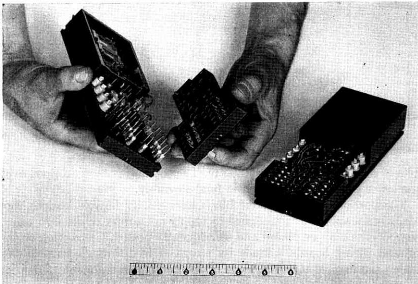
Fig. 36 — The E6 negative impedance converter.
