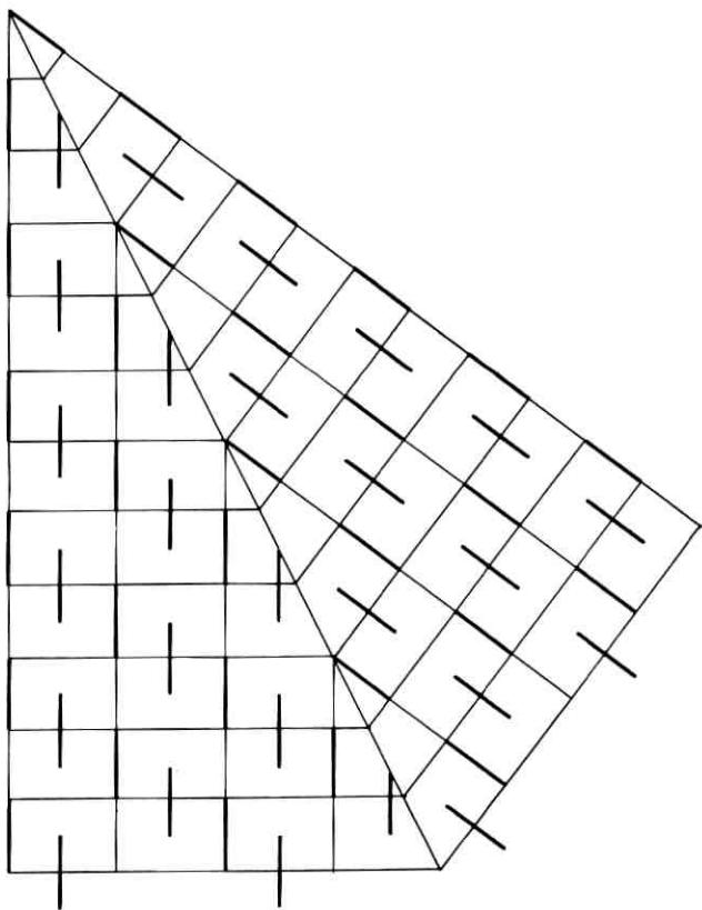
Fig. 18 —  $(200)[\frac{1}{2}\bar{1}0]:(310):(200)[\frac{1}{2}\bar{1}0]$  domain boundary in (310) twin.
