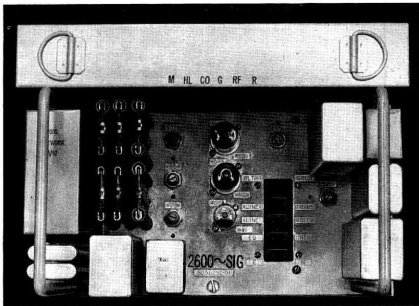
Fig. 16 — 2600-cycle SF unit (electron tubes).
