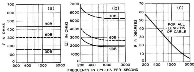
Fig. 6 — Approximate values of  $r$  and  $Z$  for built-out 19-gage H-88 cable.
