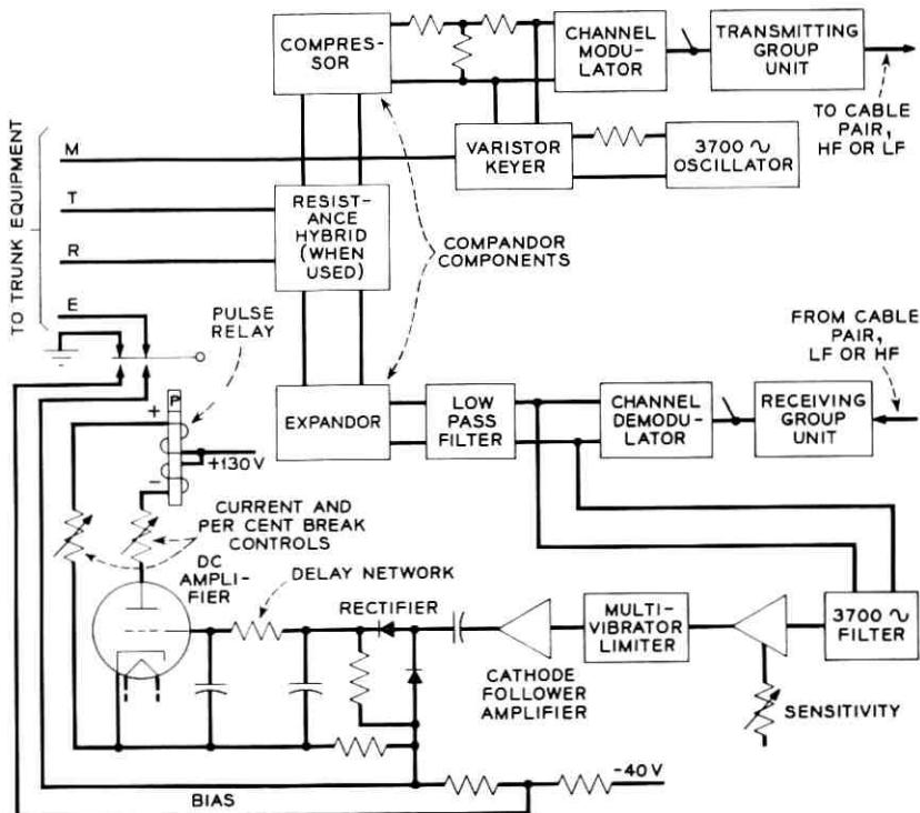
Fig. 18 — N-1 carrier signaling system (out-of-band).
