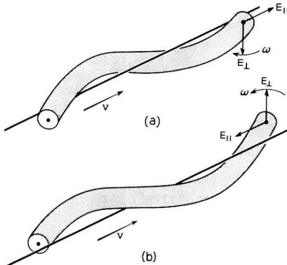
Fig. 3 — Beam motion for (b) fast and (a) slow synchronous waves excited at a frequency  $\omega$ .
