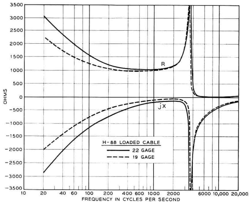
Fig. 14 — Characteristic impedance of 0.5 end-section H-88 loaded cable.
