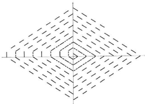
Fig. 26 — Single-spiral crystal containing  $(110)[\frac{1}{2}\bar{1}0]$ -type domains. When the  $(200)$  folds are arrayed along the horizontal axis a vacancy is generated with each loop.
