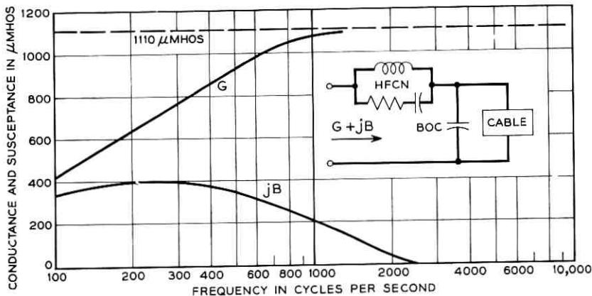
Fig. 30 — Admittance characteristic of high-frequency network, BOC, cable.
