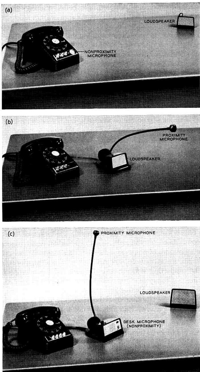
Fig. 6 — Hands-free set arrangements for proximity-nonproximity preference studies: (a) 595 telephone set; (b) proximity-talking microphone assembly; (c) combination proximity and nonproximity voice-switched telephone set.
