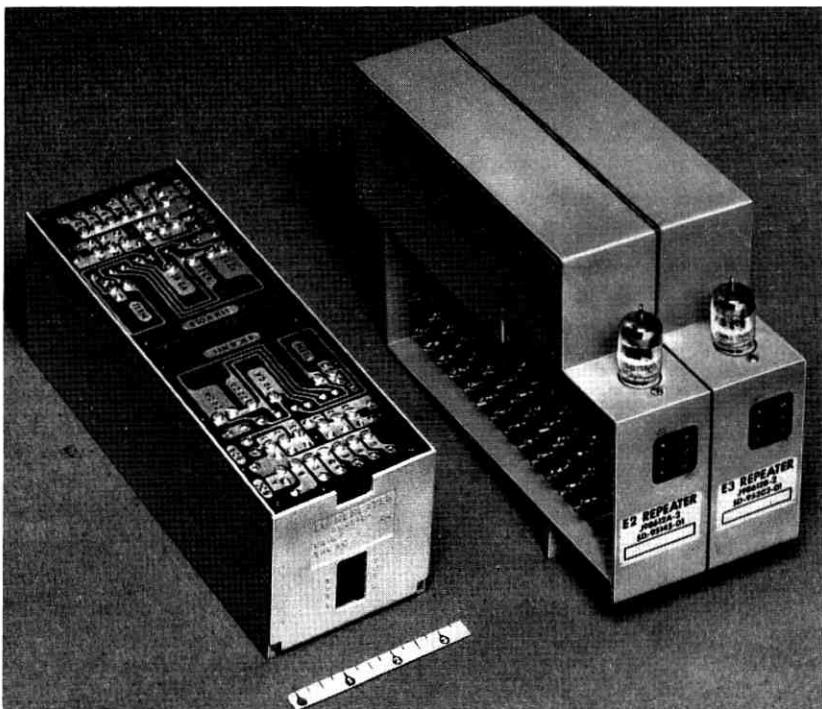
Fig. 3 — E6 repeater (left); E23 repeater (right).
