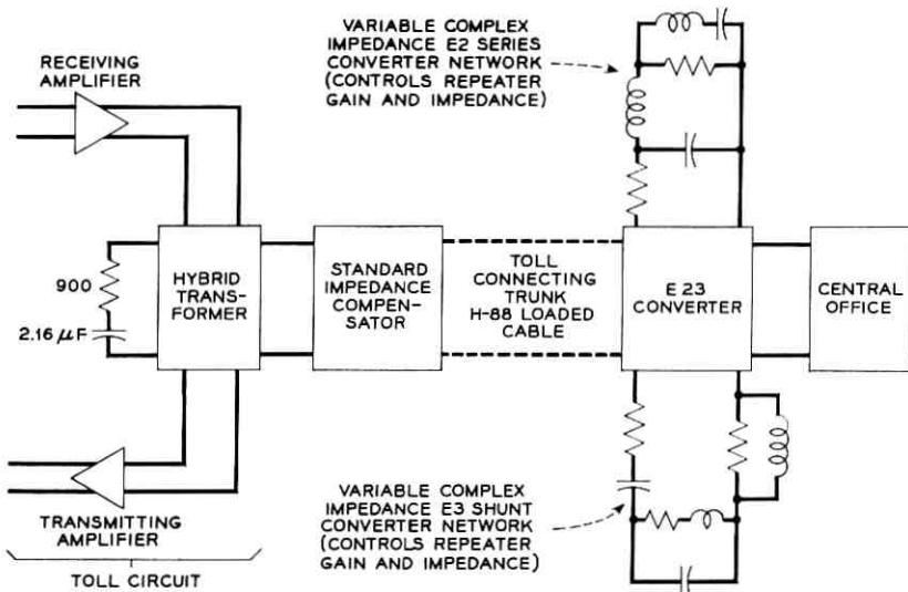
Fig. 1 — E23 repeater installation; terminal use — toll-connecting trunks.
