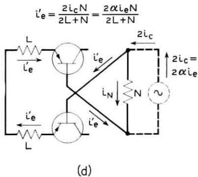
Fig. 9 — (a) Method of showing transistor currents; (b) emitter current due to line voltage  $E$ ; (c) collector currents due to emitter current of (b); (d) positive feedback path completed through lines  $2L$  to give  $i'_e$ .
