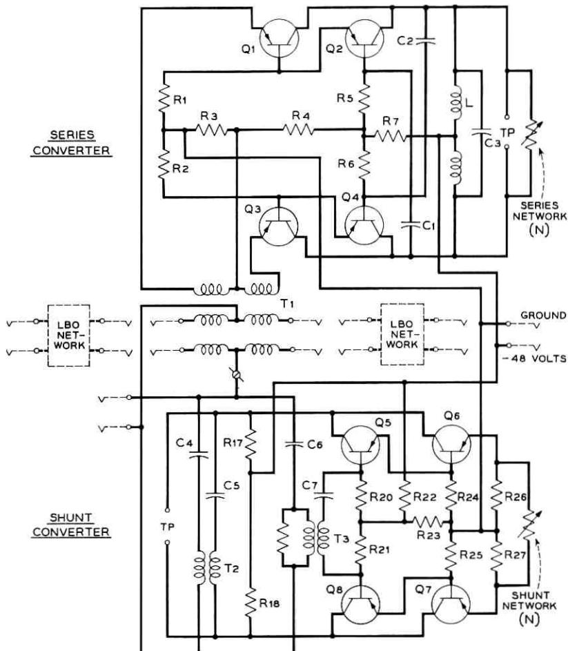
Fig. 12 — Complete schematic of E6 repeater.
