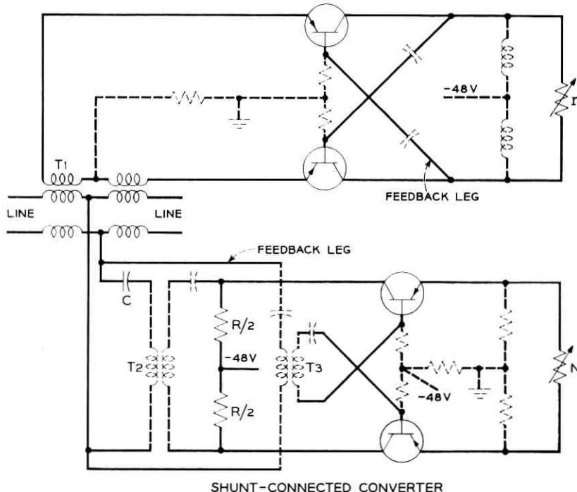
Fig. 8 — Simplified circuit of E6 converters with single transistors in each side of push-pull circuits.
