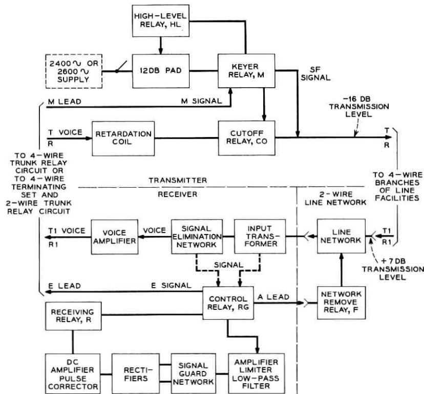
Fig. 17 — Basic elements of SF signaling circuit.
