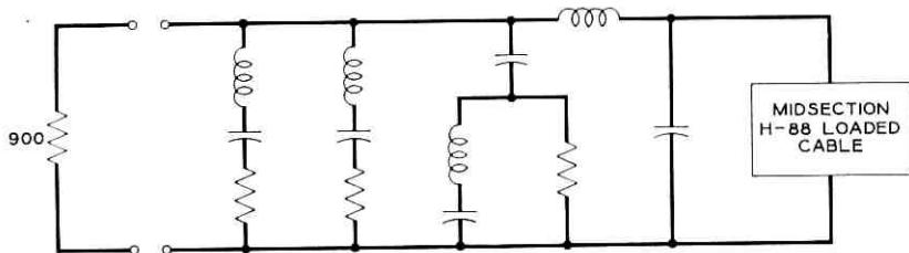
Fig. 21 — Two-terminal pair fractional termination LBO network.
