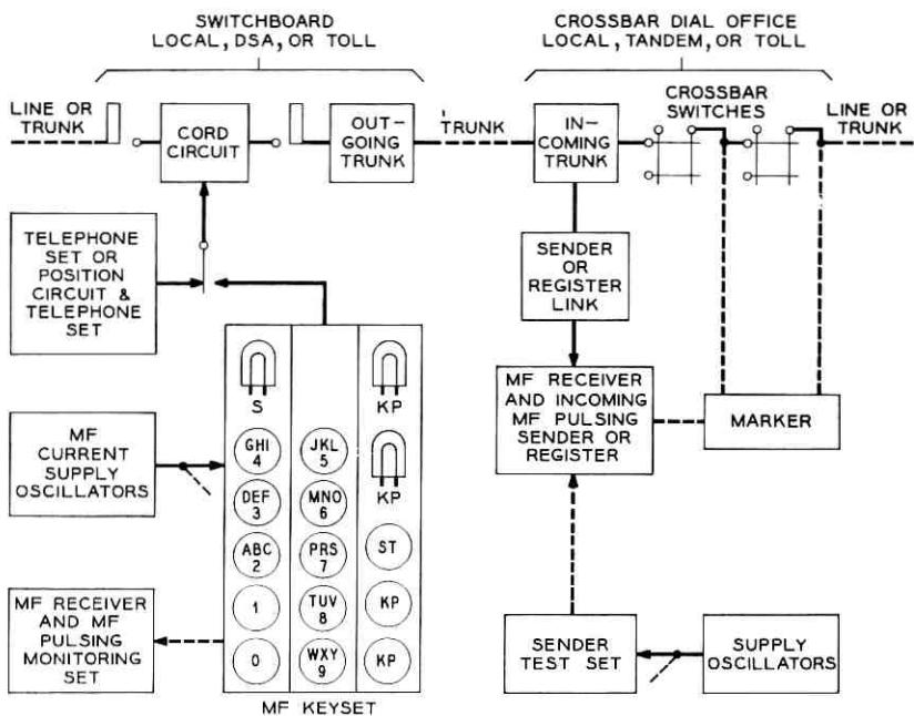
Fig. 22 — Plan of MF pulsing system.
