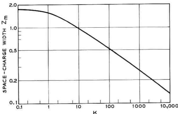
Fig. 5 — The space-charge width for the space-charge approximation.
