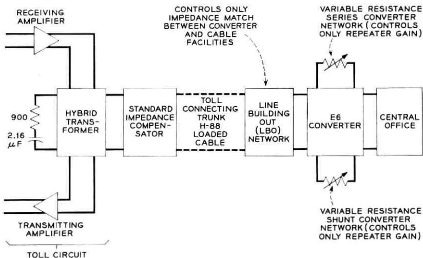
Fig. 2 — E6 repeater installation; terminal use — toll-connecting trunks.
