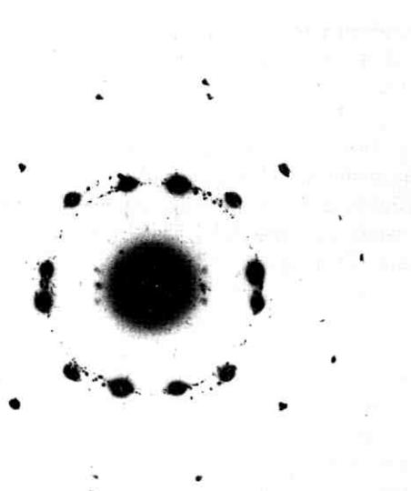
Fig. 1—Electron diffraction pattern given by crystals twinned across (530) plane.
