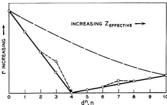
Fig. 8 — Variation of "ionic radius" with effective nuclear charge for medium-strong spin-orbit coupled tetrahedral complexes. The configurations  $d^n$ , ( $n = 0, 4, 8, 9, 10$ ) are states of perfect cubic ("pseudo spherical") eurythmy. The states  $d^2$  and  $d^7$  are but slightly asymmetric due to their spin distributions [the same may be said for  $d^6$  if it exhibits maximum spin].
