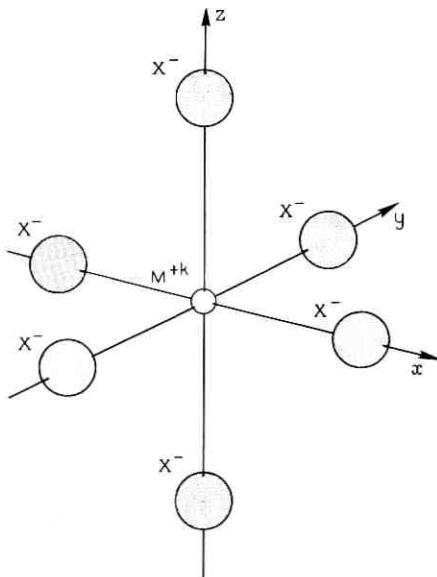
Fig. 1 — Geometrical disposition of an octahedral complex.
