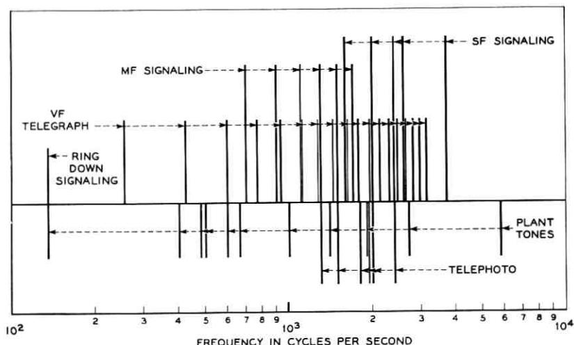
Fig. 1 — Various signaling and plant tones.
