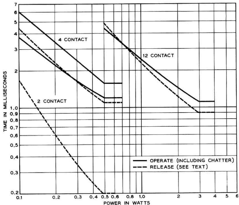
Fig. 11 — Relay function times at optimum  $G_c$ .
