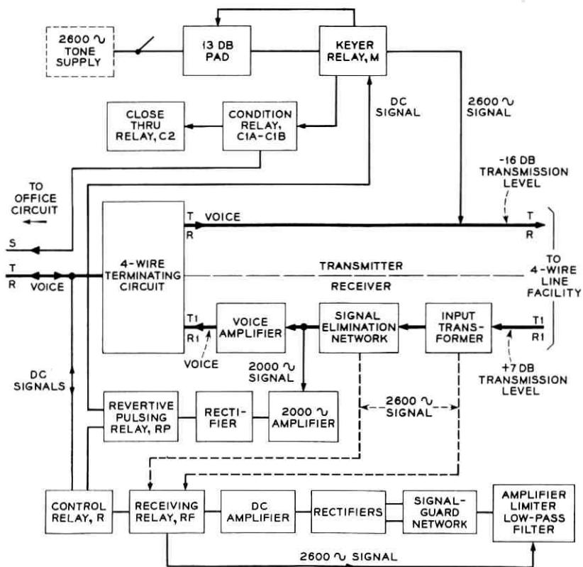
Fig. 20 — Basic elements of SF signaling unit — originating terminal retractive pulsing.
