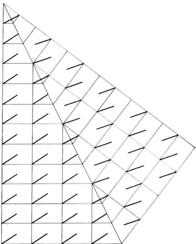
Fig. 20 —  $(\bar{1}\bar{0})[010]:(310):(\bar{1}\bar{0})[\frac{1}{2}\frac{1}{2}0]$  phase boundary in  $(310)$  twin.
