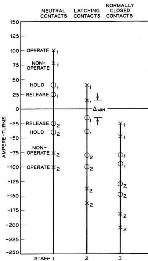
Fig. 7 — Typical characteristics of neutral and magnetic-biased relay.
