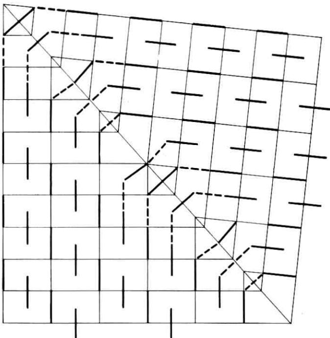
Fig. 22 —  $(200)[\frac{1}{2}\bar{2}0]:(530):(200)[\frac{1}{2}\bar{2}0]\cdot 2[\frac{1}{2}20]$  phase boundary in (530) twin.
