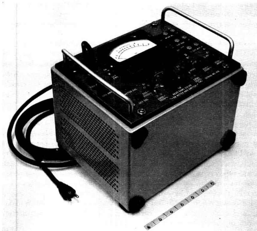
Fig. 42 — 54C return loss measuring set.
