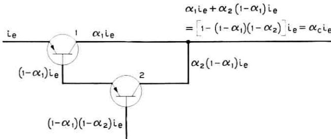
Fig. 13 — Compound transistor arrangement corresponding to single transistor.
