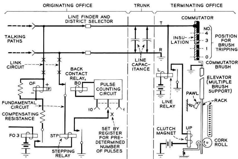
Fig. 11 — Retractive pulsing between panel offices.
