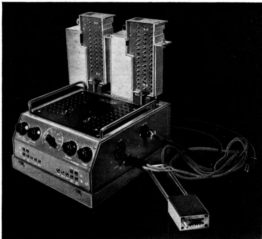
Fig. 25 — Test set showing repeaters and test cords.
