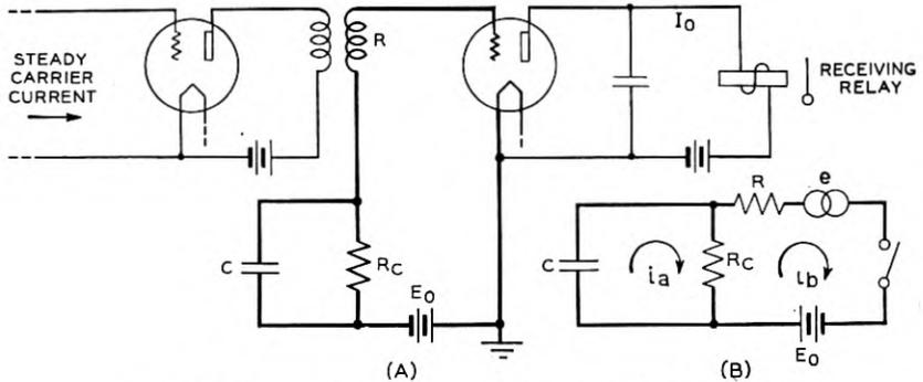
Fig. 25—Theory of level compensator. A. Simplified circuit.
