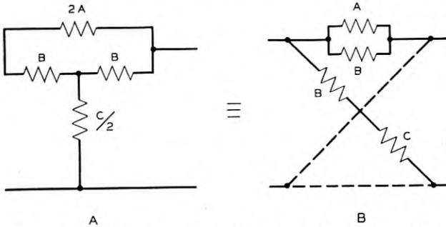
Fig. 10—Equivalence between bridge  $T$  and lattice networks.
