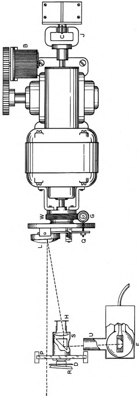
Fig. 2—The mechanical scanner and sweep frequency generator.
