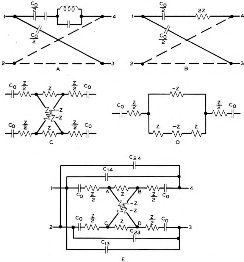
Fig. 15—Four-terminal equivalent network for divided plate crystal.
