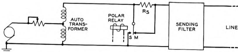
Fig. 8—Relay sending-circuit.
