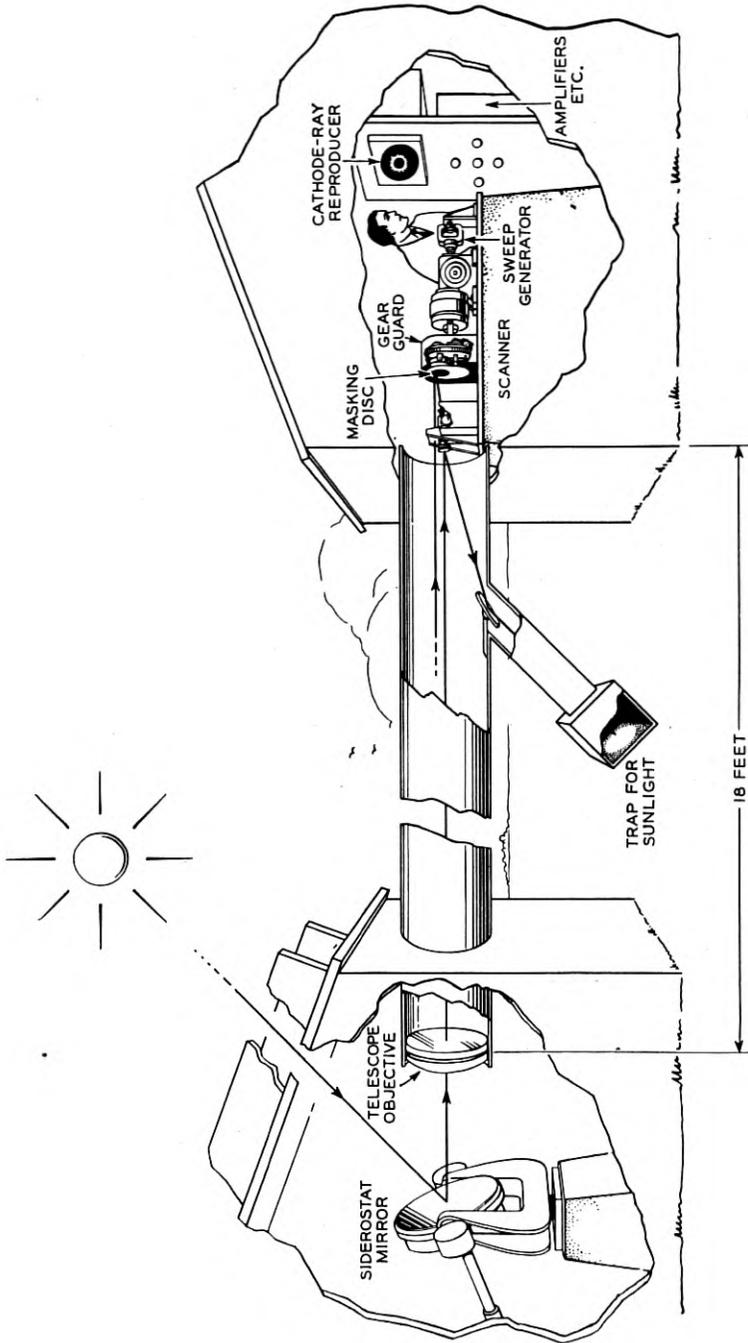
Fig. 1—Layout of apparatus at the Cook Observatory.
