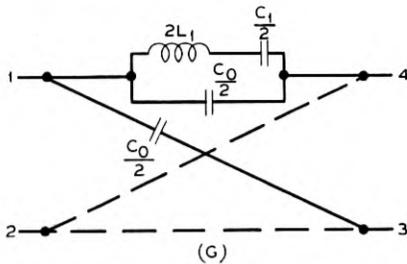
Fig. 14—Equivalent networks to represent transmission through divided plate crystal.
