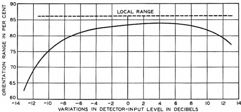
Fig. 5—Teletypewriter orientation-range vs. variations in detector input-level.
