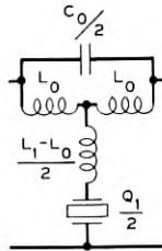
Fig. 11—A bridge  $T$  band elimination crystal filter.
