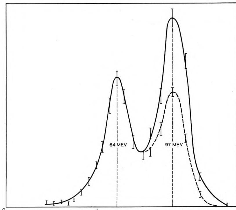
Fig. 2—Distribution-in-energy of fission-fragments of uranium.
