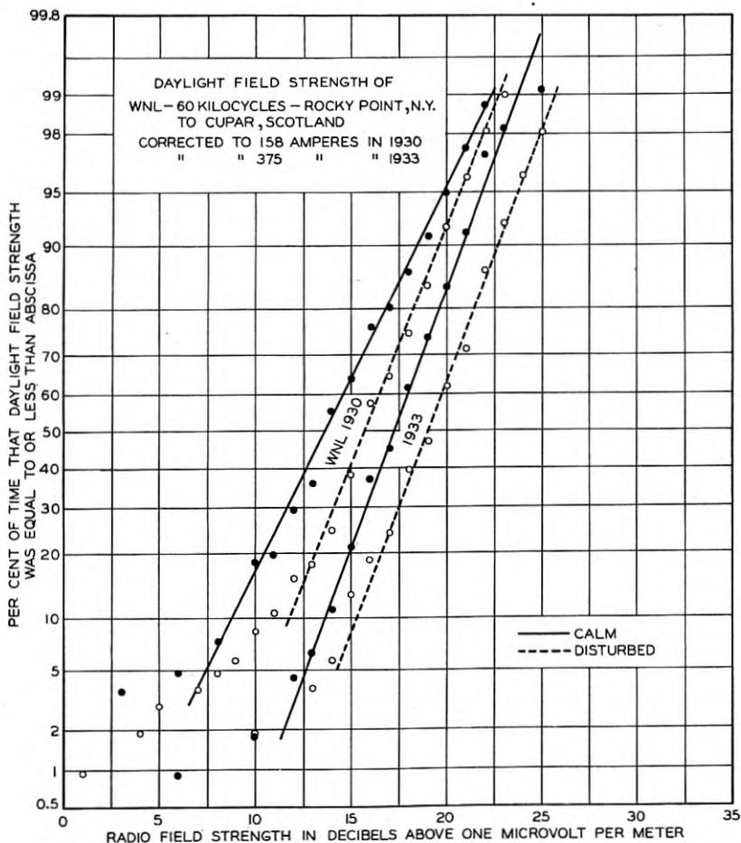
Fig. 7—Cumulative distribution of daily averages of long-wave radio field strength on days of magnetic calm and on days of magnetic disturbance. Daylight transmission path, WNL.
