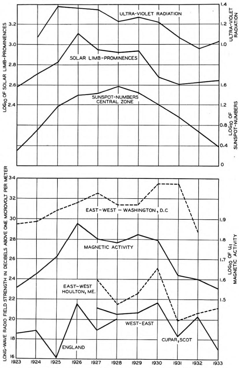
Fig. 2—Annual averages of solar phenomena, terrestrial magnetic activity, and long-wave radio transmission during one 11-year sunspot cycle.
