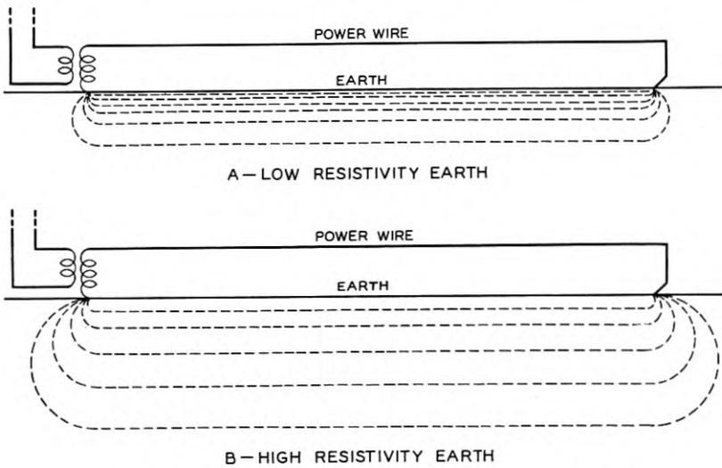
Fig. 3—Current distribution in earth of different resistivities.
