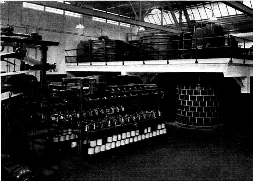
Fig. 3—Wire supply and pulp preparation equipment.
