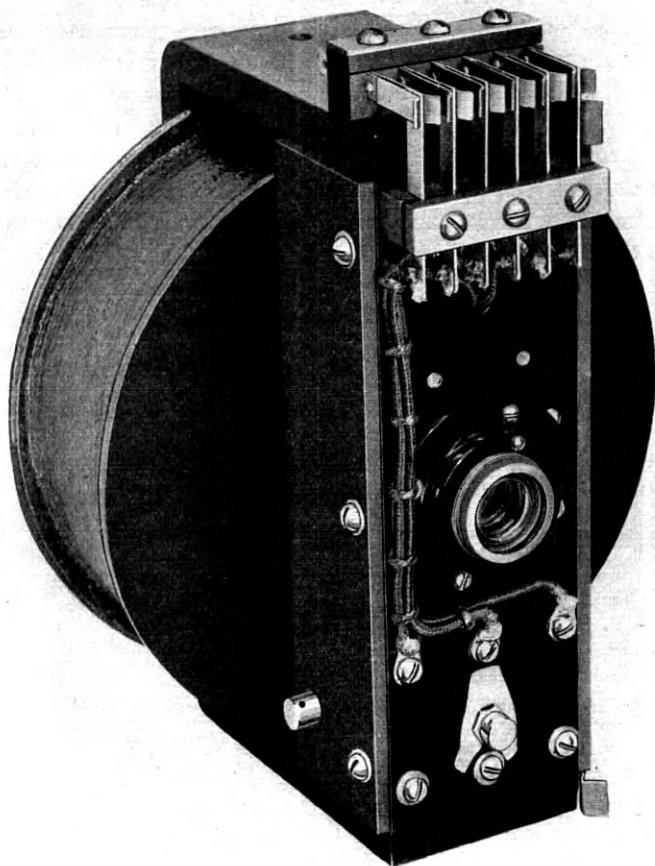
Fig. 13—Galvanometer element of rapid record oscillograph.
