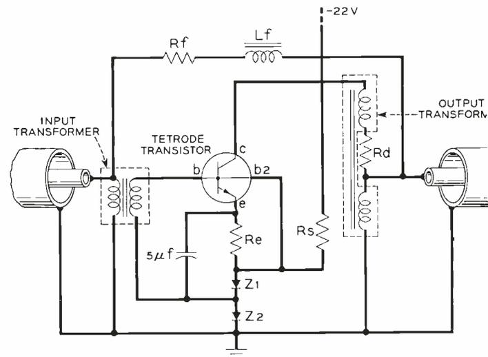
Fig. 5 — The amplifier electrical circuit.
