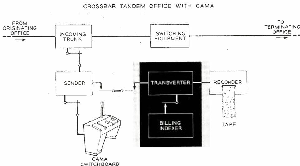
Fig. 2—Block diagram showing position of transverter and billing indexer in a crossbar tandem CAMA office.
