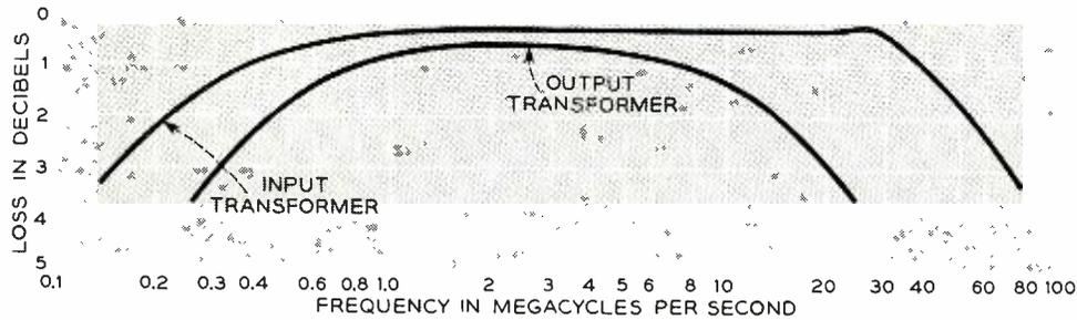
Fig. 4 — Transformer loss-versus-frequency characteristics.
