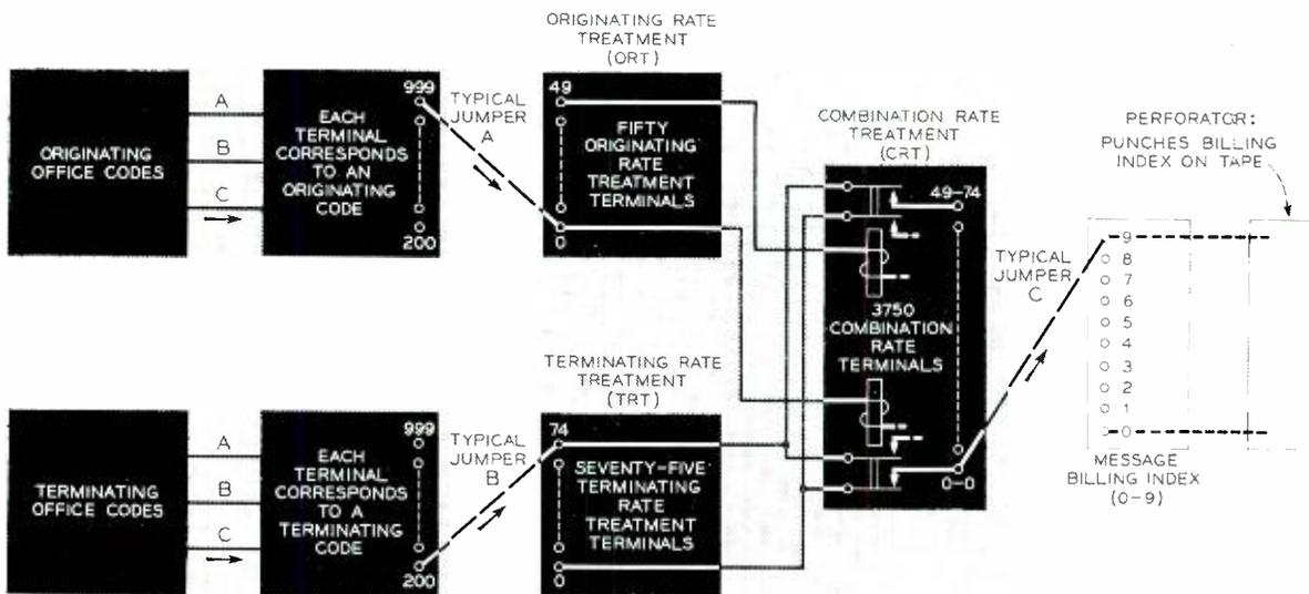
Fig. 3 — Diagram showing method of deriving billing index.
