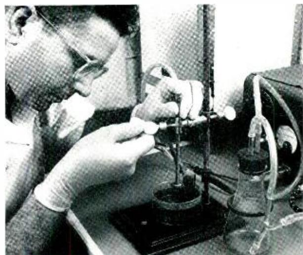
Fig. 2 — J. N. Borges electroplating a fast recombination contact to a slice of germanium.
