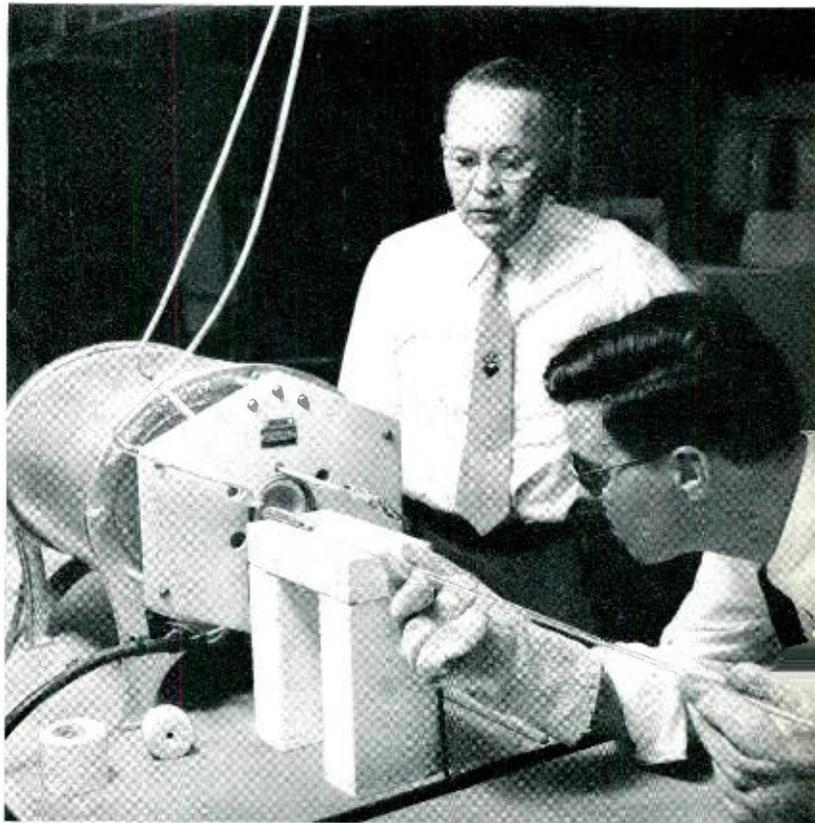
*Fig. 3 — C. S. Fuller (left) and J. A. Ditzenberger engaged in a diffusion experiment. Mr. Ditzenberger is shown inserting into a furnace a tube containing silicon plate and boron compound.*
