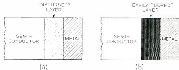
Fig. 1 — Top: "fast recombination" type of contact; bottom: "non-injecting" type of contact.
