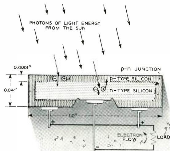
Fig. 2 — Cross-sectional view of a plate of silicon prepared as a solar cell, illustrating creation of electron-hole pairs by photons of light energy.
