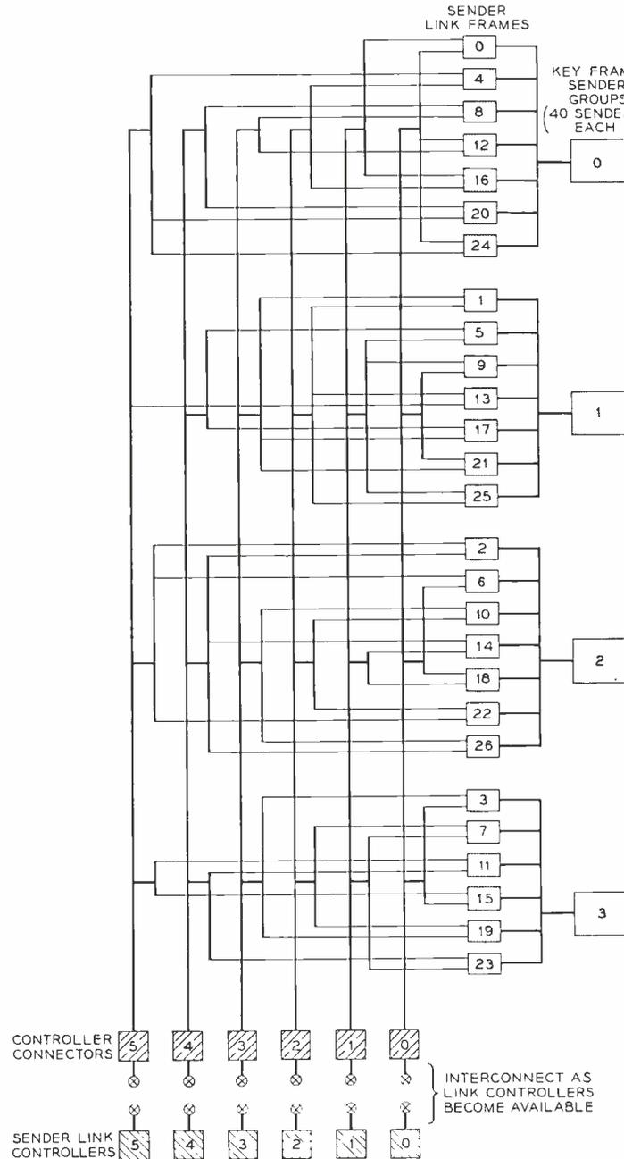
Fig. 3 — How senders may be distributed among the various link frames is shown in this diagram. Six link controllers and six connectors can direct traffic from approximately 2,700 trunks.
