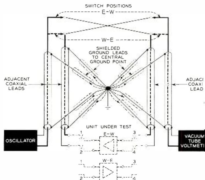
Fig. 4 — Final arrangement of coaxial cables and shielded ground leads in the test set.
