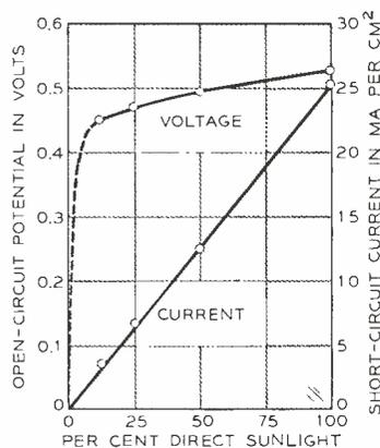
Fig. 5—Open-circuit voltage and short-circuit current for different percentages of sunlight, at an operating temperature of 25°C.
