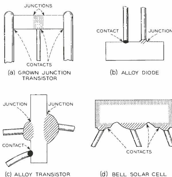
Fig. 4 — Four uses of non-injecting contacts.
