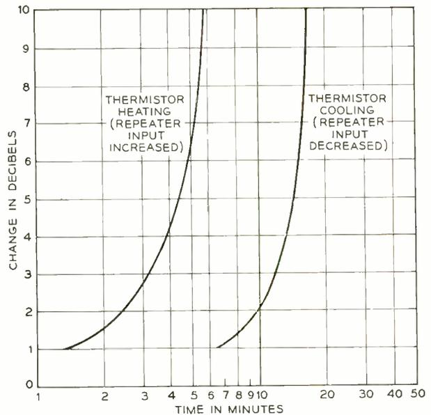
Fig. 3—Heating and cooling characteristics of the thermistor beads used in the repeaters.
