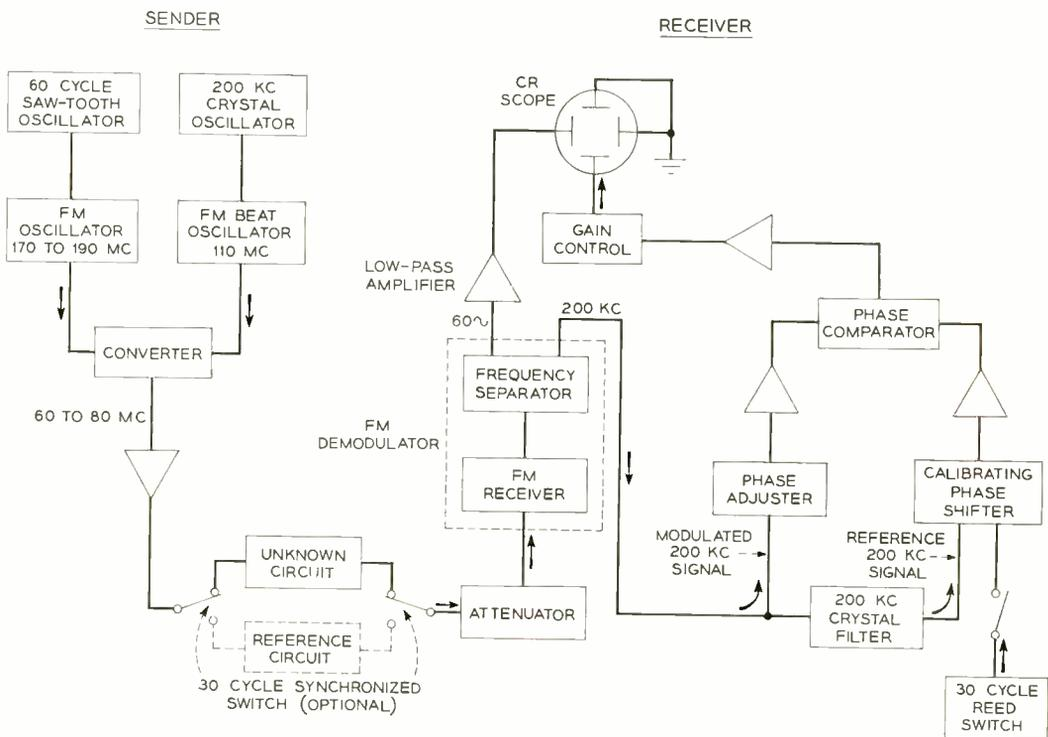
Fig. 3 — Block diagram showing the principal components in a delay distortion scanner.
