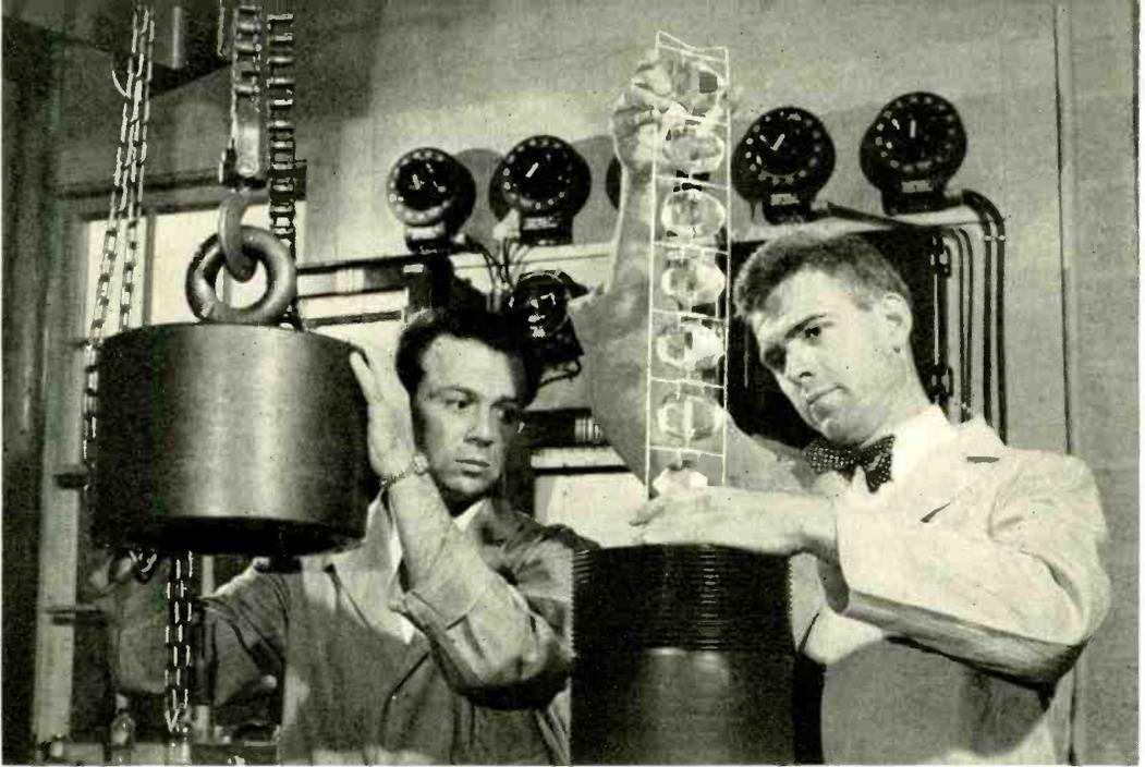
Fig. 6 — The author and A. J. Caporaso (left) removing a group of crystals from an autoclave.
