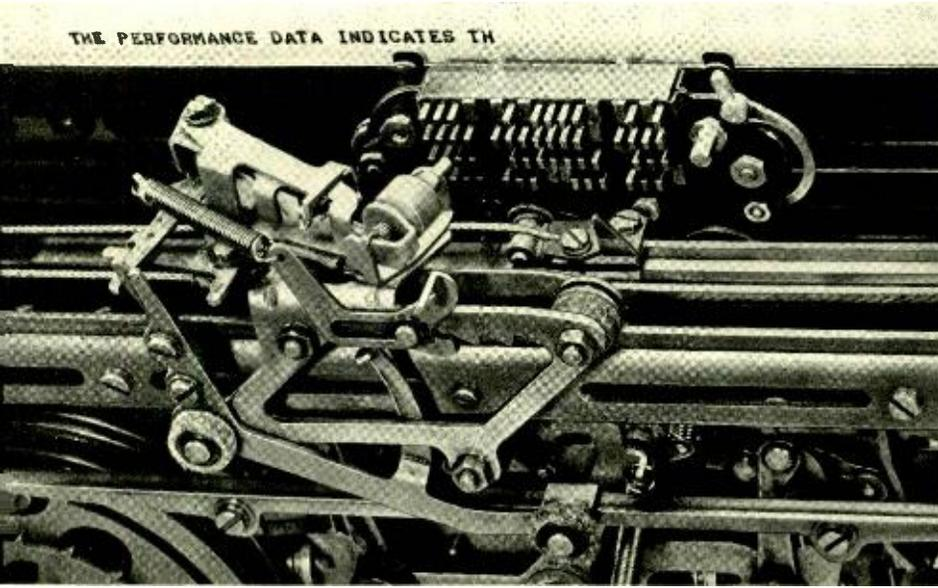
*Fig. 3 — When the type-box is in the desired position, the printing hammer drives the type pallet against the ribbon and paper.*
