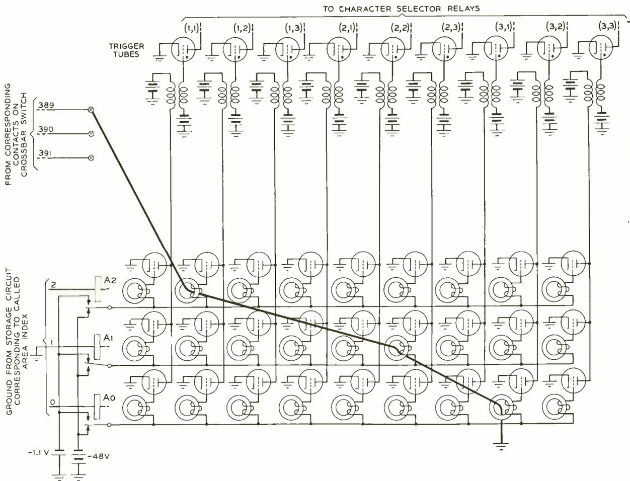
Fig. 4 — Nine ring coils corresponding to each of three dial areas with the line from the 389 contact on the crossbar switch threading one coil in each group.
