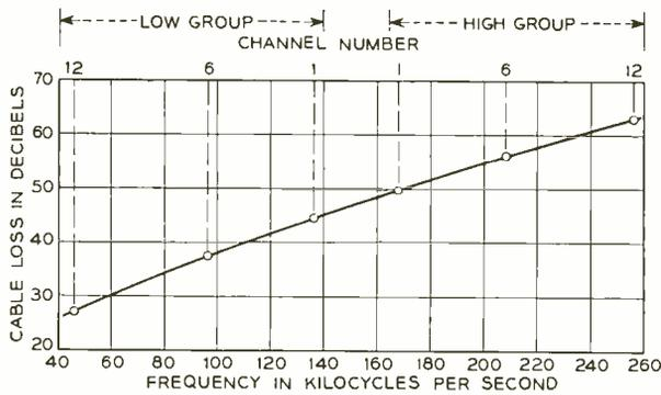
Fig. 1—Typical repeater section loss characteristic.
