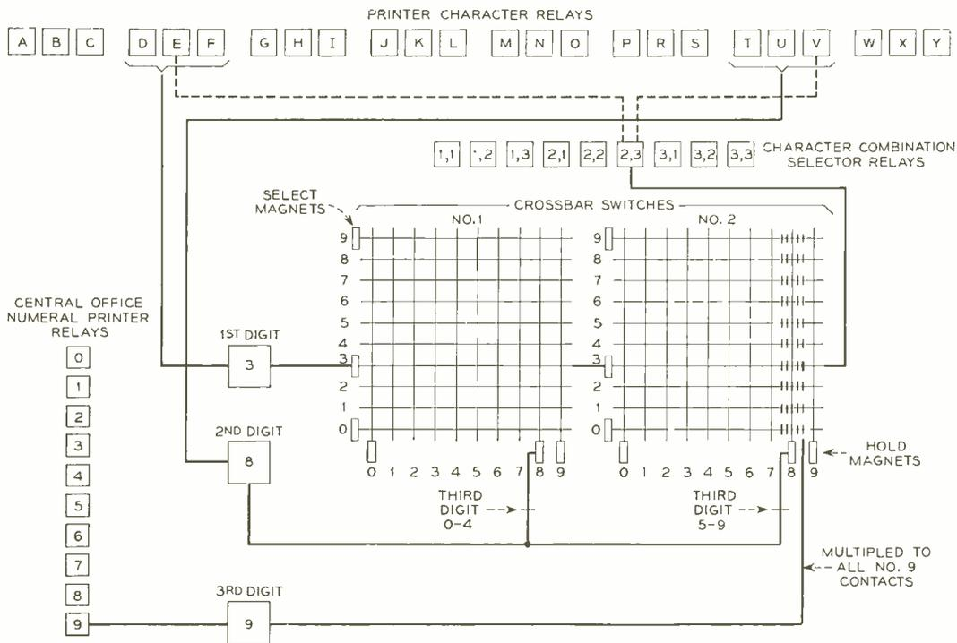
Fig. 3—Block diagram of called office name translator as used for single area translations.
