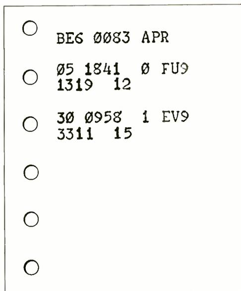
Fig. 5 - Sample toll slip from printer showing calls to the FULTON-9 and EVERGREEN-9 offices.
