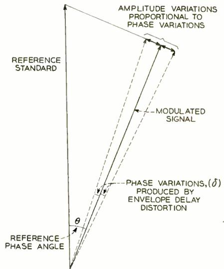
Fig. 5—Vector diagram illustrating the method used to transform phase to amplitude variations.
