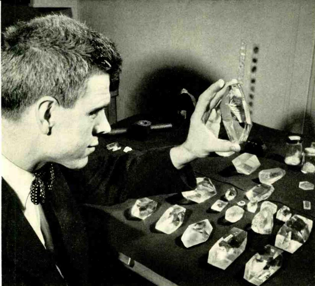
*Fig. 1 — The author examining artificially grown quartz crystals.*
