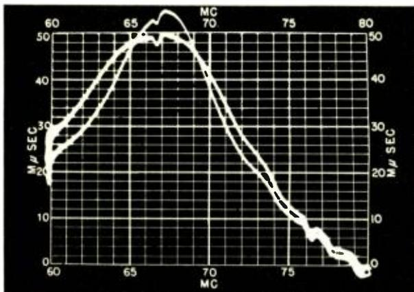
Fig. 2—Superimposed traces on the screen of a CRO tube produced by a standard equalizer and a similar unit under test.
