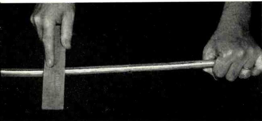
*Cleaning lead sheath preparatory to use of the cable sheath slitter is essential to the final soldering operation.*
