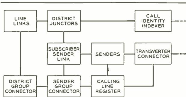
Fig. 6—Auxiliary equipment in a No. 1 crossbar office to transmit information from the line link frames to the senders.
