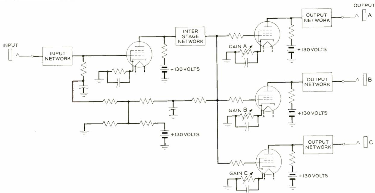
Fig. 2—Circuit of the distributing amplifier.
