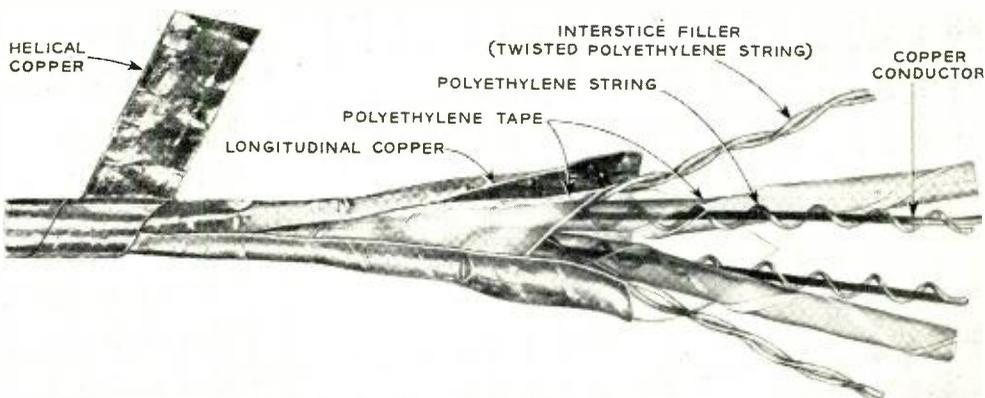
Fig. 1—Construction details of the various elements, including the longitudinal inner copper shield now incorporated in the standard video pair.
