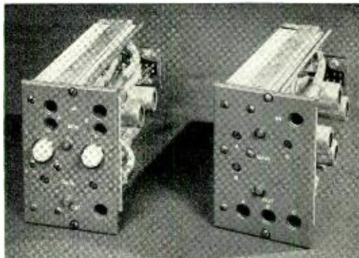
Fig. 3—A switching amplifier at the left, and a distributing amplifier at the right.
