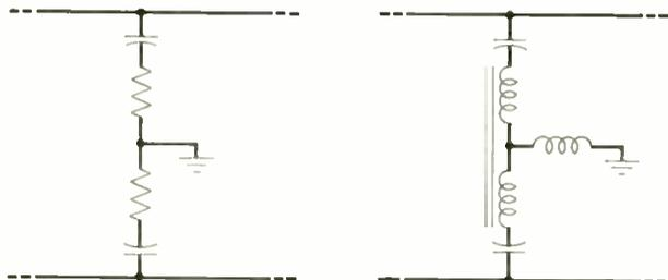
Fig. 1—Circuit of the 104A protector, at the left, and for the 108A protector, at the right. The lightning protection has been omitted for simplicity.
