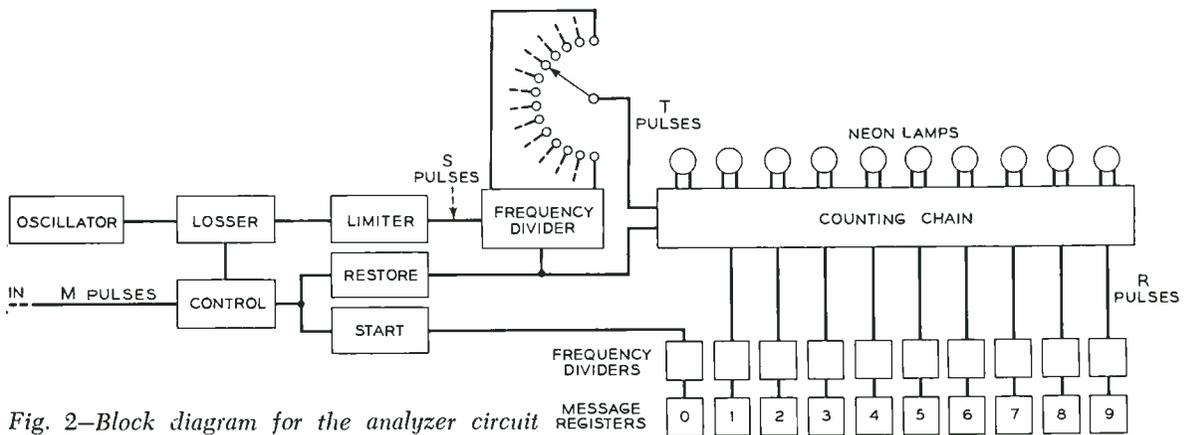
Fig. 2—Block diagram for the analyzer circuit
