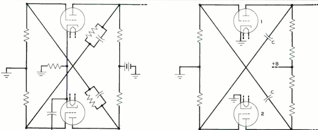
Fig. 3—A multi-vibrator circuit, right, and the similar analyser circuit, left
