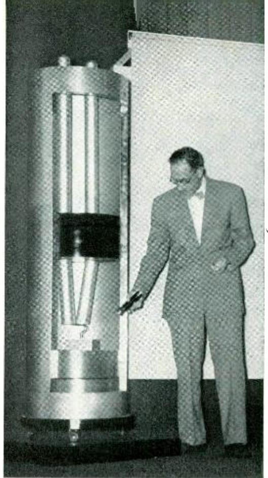
*At the demonstration, Ralph Bown described the Transistor using this 100-to-1 model*
