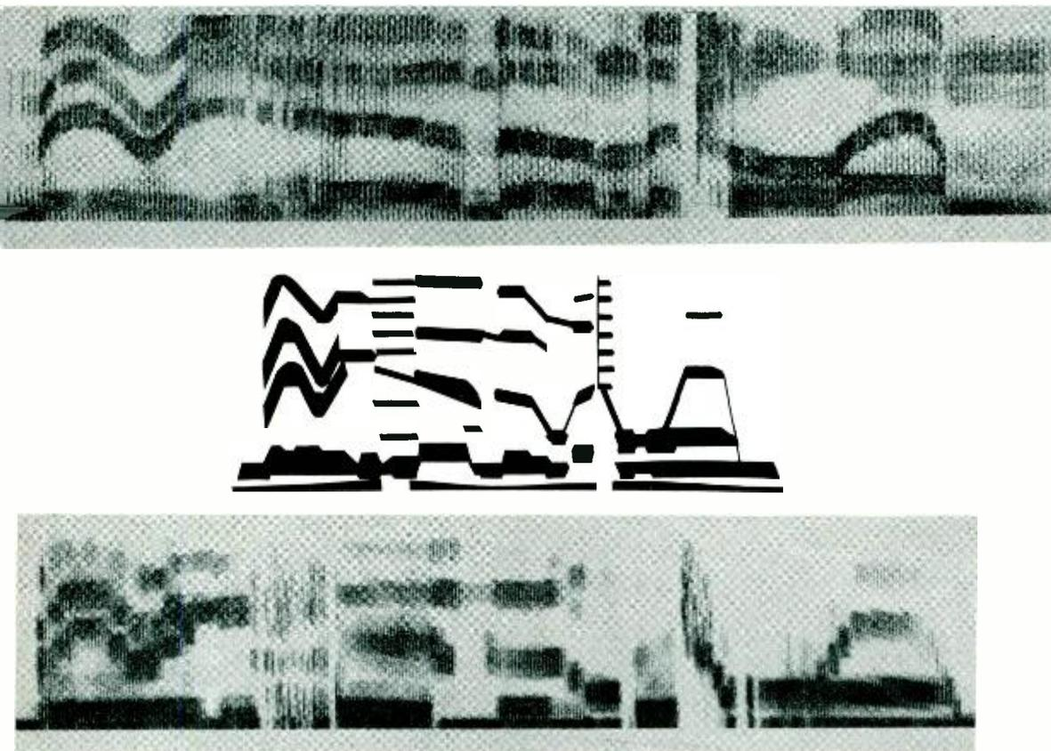
Fig. 2—A real-speech spectrogram above; a corresponding playback pattern in the mid
