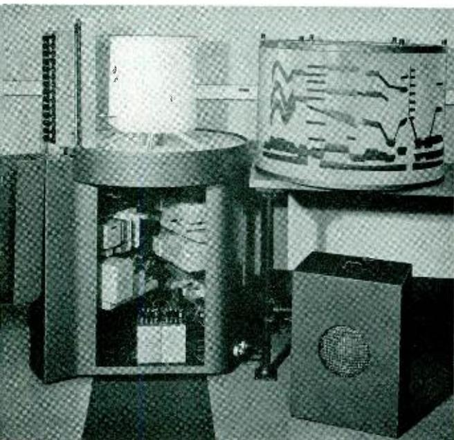
*Fig. 3—The speech playback apparatus with drum removed exposing the fluorescent light arrangement, the hood for the photoelectric cell rack lowered, and a panel below taken off exposing the synthesizing units*
