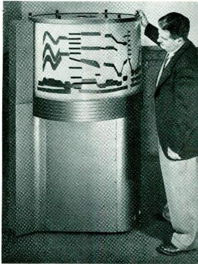
Fig. 1—The playback apparatus for visible speech
