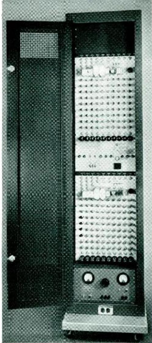
*Fig. 6 — Two analyzer panels are mounted with their power supplies in a single cabinet*
