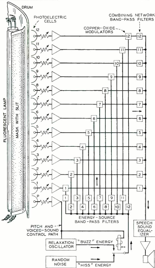
Fig. 5—Block schematic of the playback circuit showing the fluorescent lamp with its slit housing, the drum wall, the cells and the associated equipment
