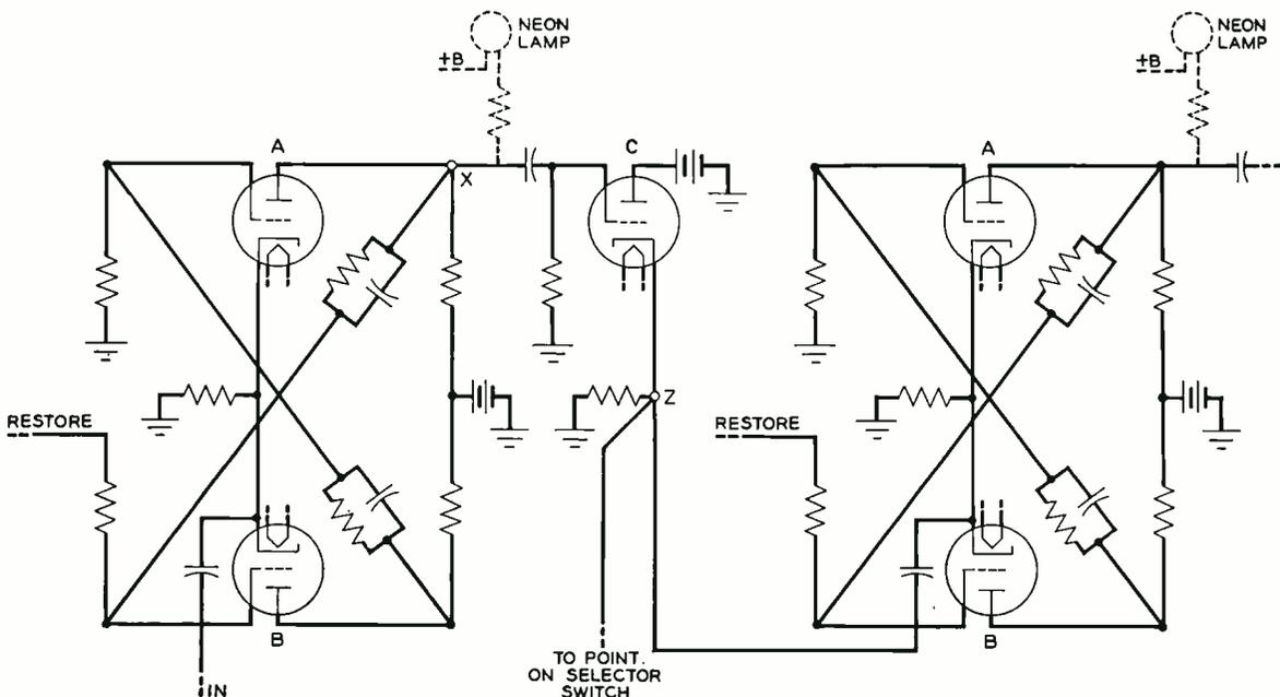
Fig. 4—Two stages of the frequency dividing circuit. A similar circuit is also used for registering with neon lamps as indicated in dotted lines above
