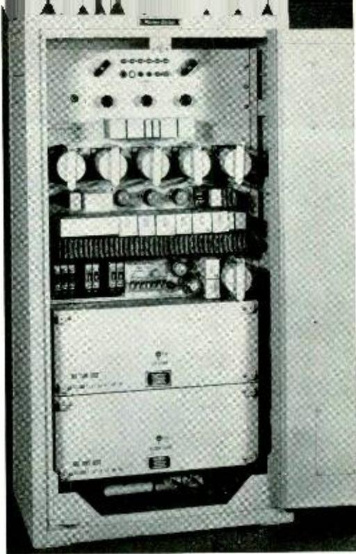
Fig. 5—The automatic telegraph monitoring set
