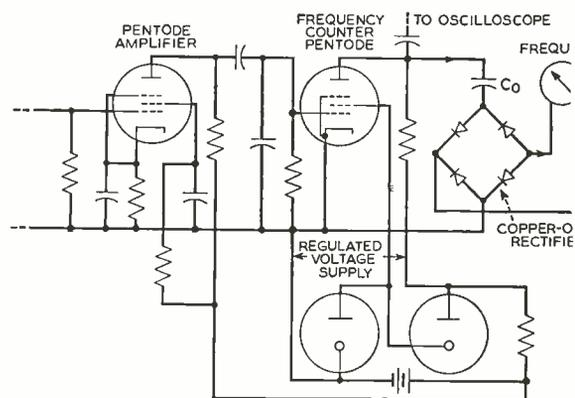
Fig. 5—Schematic of the frequency meter
