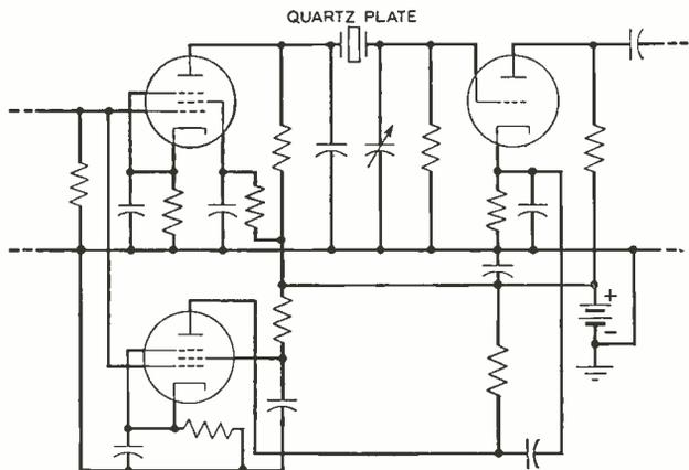
Fig. 4—Schematic of the filter
