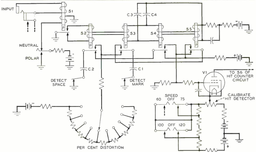
Fig. 2—Simplified schematic of the hit detector circuit
