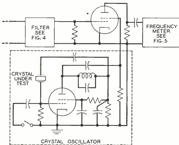
Fig. 3—Simplified schematic of the calibrator circuit
