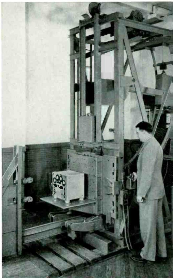
*Fig. 8—Light-weight, high-impact shock testing machine being operated by A. Taggerty*
