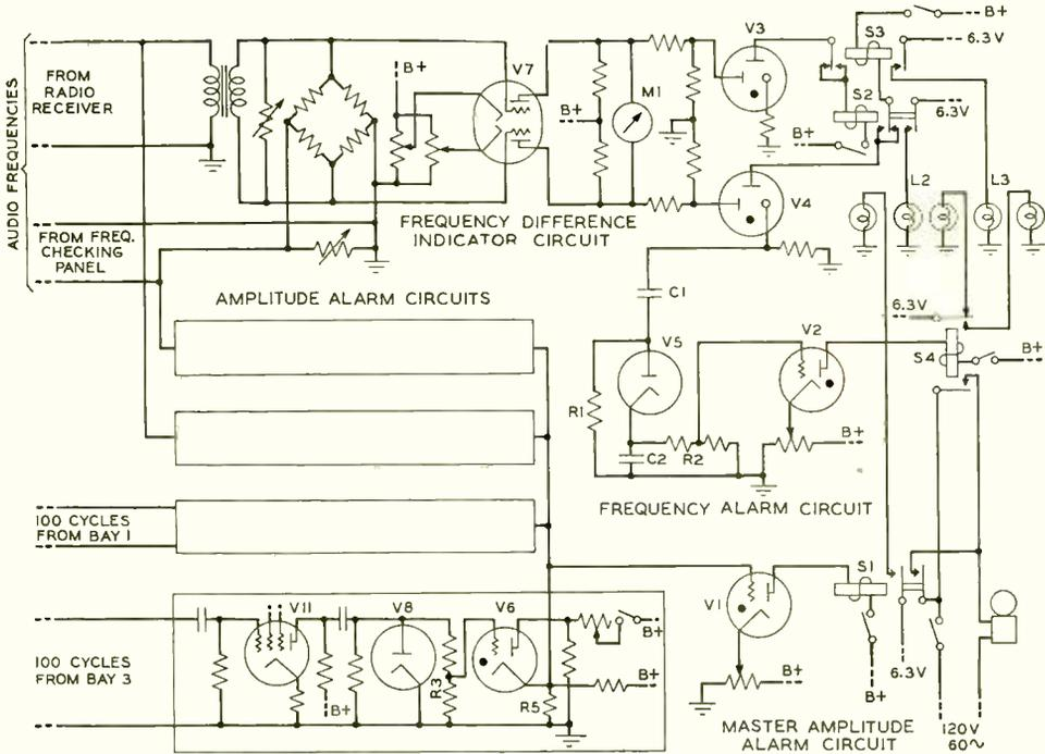
Fig. 2—Alarm and comparison circuit
