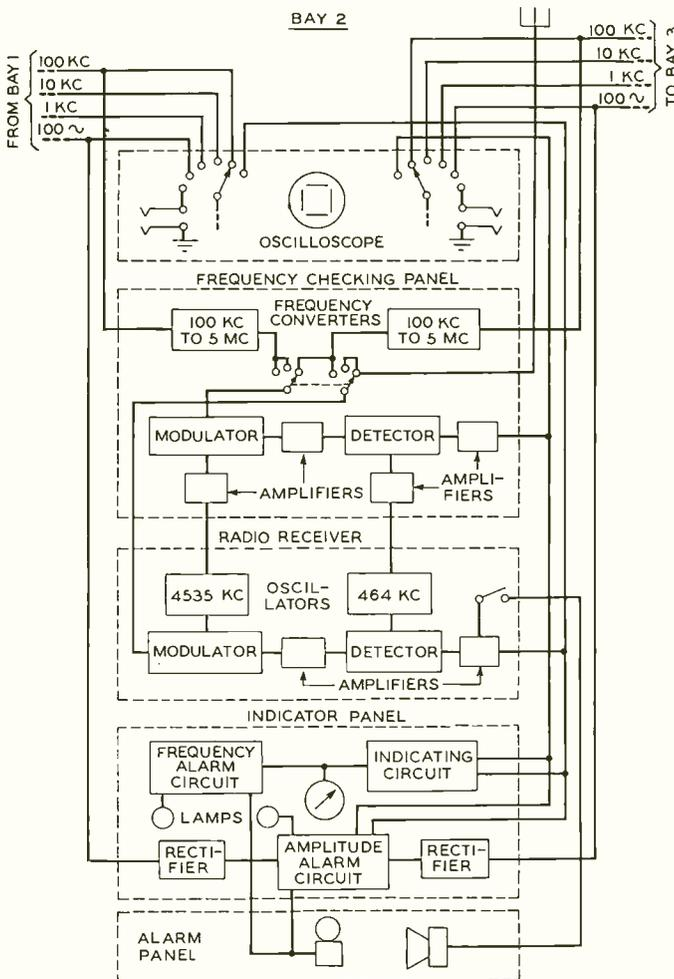
Fig. 1—Block schematic of circuits of checking bay—bay 2 in the actual line-up
