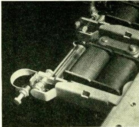
Fig. 5—To make the clutch on the elevators of the panel selectors release more quickly and thus reduce overthrow of the brushes, a U-shaped spring has been added
