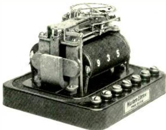
*The 60-A selector: as the armature vibrates, it advances the wheel from which stop-pins are seen projecting downward*
