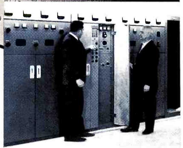
**In electronic phototypesetting** ... this Fototronic system is in operation at Typo Photo Composition, Inc., Philadelphia, Pa. The keyboard console (foreground) has a built-in digital computer, uses simple typewriter keyboard. The computerized print-out unit behind it exposes type on film or paper, is capable of handling output of up to six keyboard consoles simultaneously.
