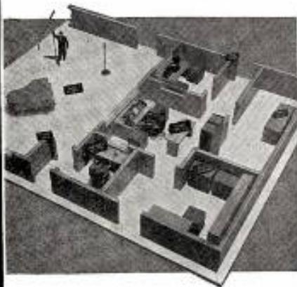
The plan above is one of three basic radio station designs, for new or modernized stations, now available from RCA. It approaches the ultimate for a larger type of radio station. Spacious studio area is incorporated in this plan, with area for other operational requirements; the transmitter would be located in its own building. By considering each plan individually, you can suit your special needs exactly.
