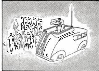
**FIELD EVENTS.** A DuMont-equipped Television Truck is a small station in itself . . . including cameras, control and sound equipment, relay transmitter and directional antenna. The relay receiver is located with the main transmitter.
