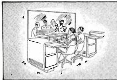
**PRODUCER'S CONTROL DESK.** Monitors show scenes being picked up by different cameras . . . with the largest monitor showing the scene selected for broadcasting. The producer sees the scene exactly as looker-listeners see it on DuMont Telesets.
