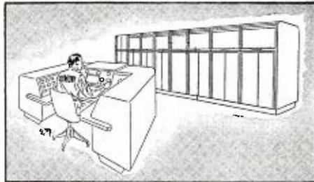
**TRANSMITTER AND CONSOLE.** All meters, oscillographs, controls and clocks are separately mounted in the console for safety, easy visibility and centralized operation. Video and audio signals (sight and sound) are transmitted from different antennae located on the same transmitting tower.
