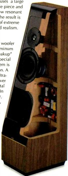
The baffle is sloped to properly position the drivers for correct time alignment and accurate reproduction of transient musical information. The grilleboard incorporates rounded edges to greatly reduce energy diffraction which contributes to very "open" reproduction.
