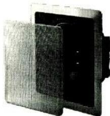
The WS008A is constructed from a one-piece baffle and chassis to reduce vibrations. The woofer has a mineral filled polypropylene cone with a rubber surround and high temperature Kapton voice coil. The tweeter is a 1" Aluminum dome with a Neodymium magnet and ferrofluid cooling. The crossover is 24dB per octave, with polypropylene capacitors in the tweeter circuit for greater clarity.
