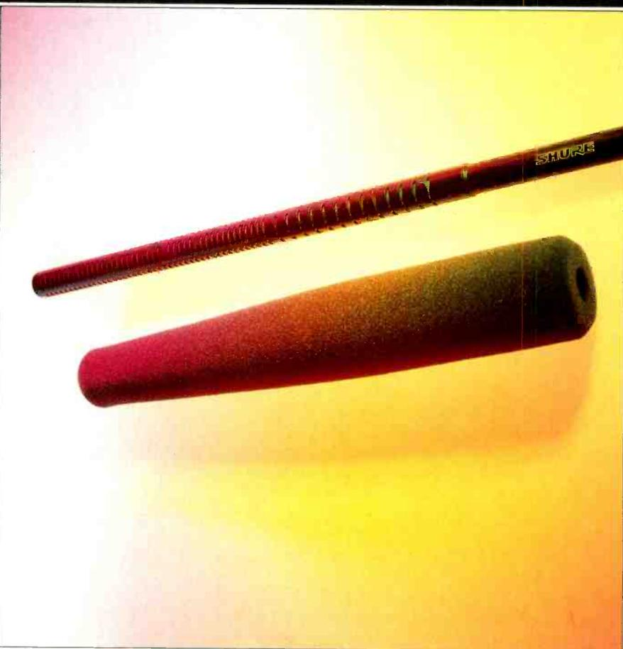
Shotgun, or line, microphones are designed for high directivity in long-distance sound pickup. While early models (see sidebar) used tubes 5 or 6 feet in length, modern units like the Shure SM89 use slotted or perforated tubes, about one-third as long as those of early shotguns, coupled to high-sensitivity transducers. These line microphones use the principle of wave interference to achieve their high
