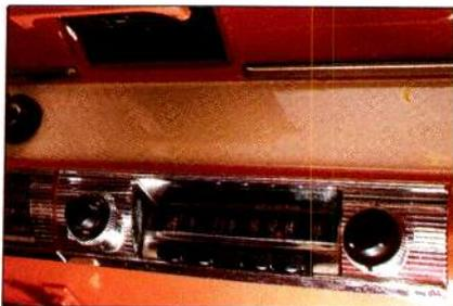
*. . . or is it? Note the CD changer's remote control under the ashtray (top), the preamp knobs peeking out from under the radio buttons, and the digital display barely visible between 8 and 10 on the radio dial.*
