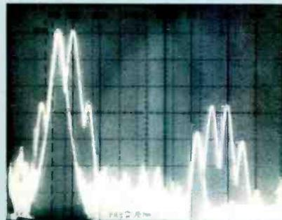
Fig. B2—Third-order distortion products. At left are 500- and 600-Hz fundamentals, flanked by third-order difference products. At right are third harmonic of 500-Hz fundamental (1,500 Hz), third-order sum products of 500 and 600 Hz, and third harmonic of 600 Hz (1,800 Hz). Scales: Horizontal, 200 Hz/div.; vertical, 10 dB/div.
