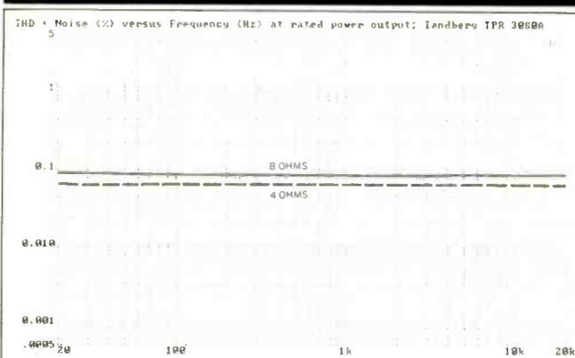
**Fig. 7—Amp THD + N vs. frequency; 8-ohm performance (solid curve) measured at full rated output of 80 watts per channel; 4-ohm performance (dashed curve) measured at 115 watts, 15 watts above rated output.**
