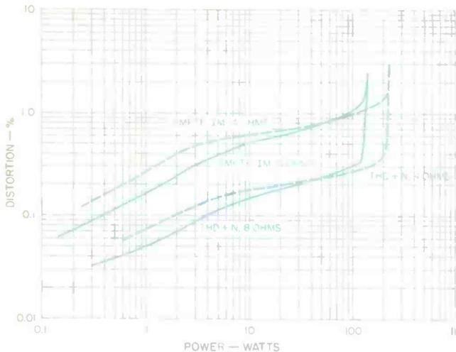
**Fig. 8**—SMPTE IM and THD + N vs. power for 4 and 8 ohms. THD + N is for a 1-kHz test signal, with distortion products measured from 400 Hz to 80 kHz.
