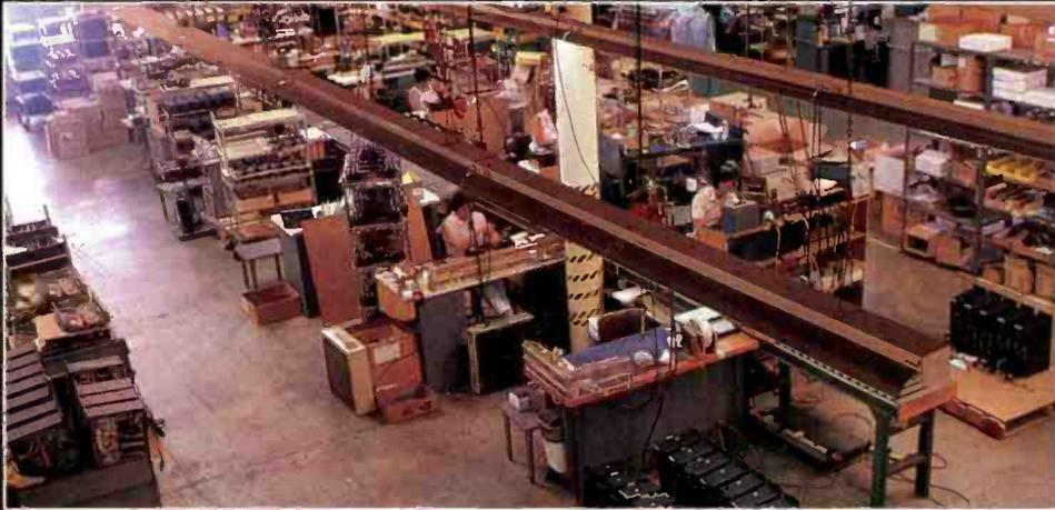
One hundred percent quality control is seen on EVERY unit manufactured. EVERY completed unit is electronically tested for specification accuracy and then EVERY unit is connected to a high fidelity system and listened to—just like you would at home. If your unit meets or exceeds the critical standards set forth on these tests, it is then packaged for shipment.
