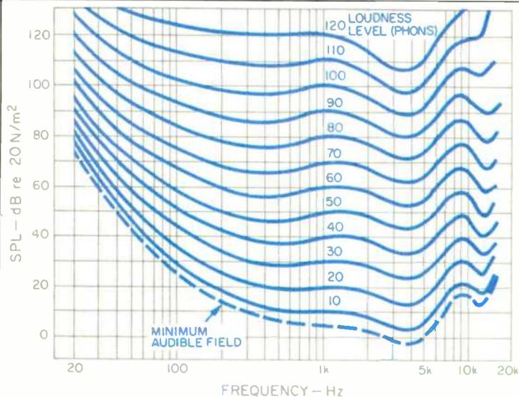
Fig. 1A—Equal-loudness contours, showing how average human hearing sensitivity varies with frequency and level. (After Robinson and Dadson.)
