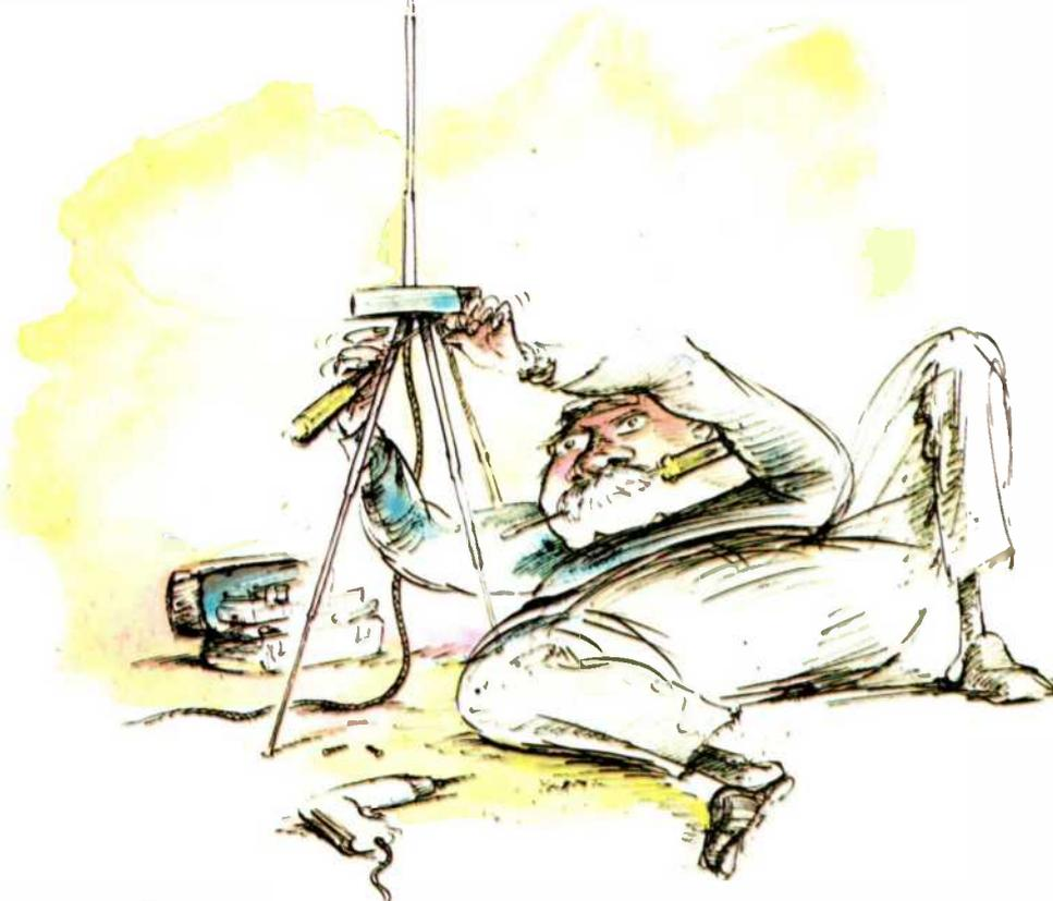
The antenna itself is of the same kind of rod as the legs. I used collapsible replacement antenna rods, which are available from most radio/TV supply shops. In fact, any metal rod that can be worked into the configuration shown will serve the same function. The minimum length required, however, is 28 inches.
