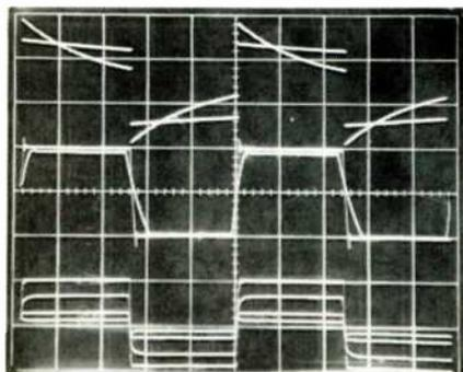
**Fig. 6**—Line-section square-wave response. Top trace is at 20 Hz, with IHF and instrument loading (traces superimposed). Middle trace is at 20 kHz, 10 V peak to peak, with instrument and IHF loadings superimposed. Bottom trace is at 20 kHz, instrument loading, for various volume control positions; see text.
