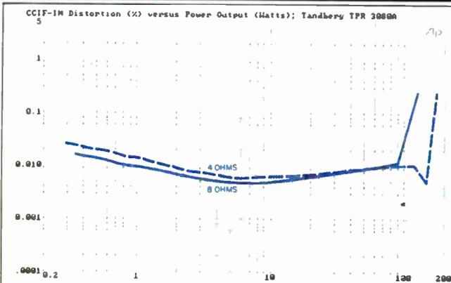
Fig. 10—CCIF-IM (two-tone) distortion vs. power output for 8- and 4-ohm loads.
