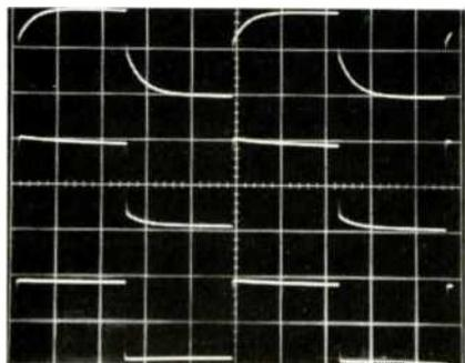
**Fig. 4—MM phono response to pre-equalized 1-kHz square wave at three input levels.**
