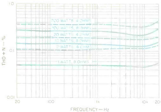
**Fig. 7**—THD + N vs. frequency for MS100 amp, at various power levels, into 4 and 8 ohms.
