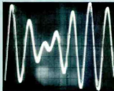
Fig. B1—Waveform of 500- and 600-Hz test signal.
