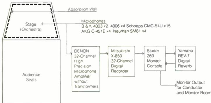
Fig. 2—Setup for Denon's anechoic recording.
