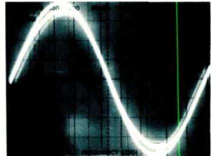
Fig. 23—Shape of playback sine wave with low distortion (larger trace) and with 3% distortion (smaller trace); see text.
