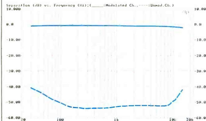
Fig. 5—Frequency response and stereo separation. Note change of vertical scale from Fig. 1.
