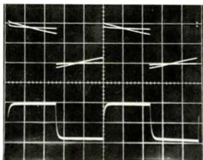
**Fig. 3—MM phono response to pre-equalized square waves of 40 Hz (top trace) and 10 kHz (bottom trace), for both instrument and IHF loading. The effects of the**
