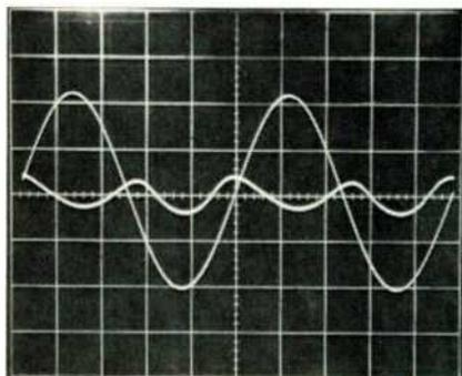
**Fig. 9—Response to 10-watt, 1-kHz sine wave. Distortion products (predominantly even harmonic) are superimposed.**
