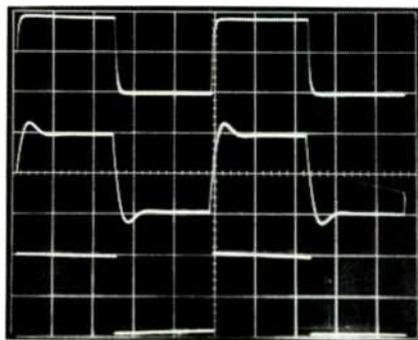
**Fig. 11—Amplifier response to square wave. Top trace is 10 kHz with 8-ohm resistive load. Middle trace is 10 kHz with 2- $\mu$ F capacitance across 8-ohm load. Bottom trace is 40 Hz with 8-ohm load. Scales: Vertical, 5 V/div.; horizontal, 20  $\mu$ S/div. (top and middle) and 5 mS/div. (bottom).**
