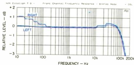
**Fig. 1—Front-channel frequency response, stereo mode.**
