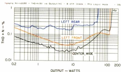
**Fig. 12—THD + N vs. amplifier output, Dolby Pro Logic mode.**
