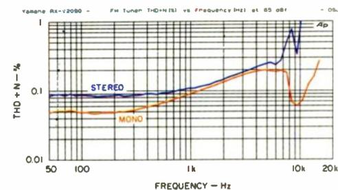
**Fig. 9—THD + N vs. frequency, FM tuner section.**
