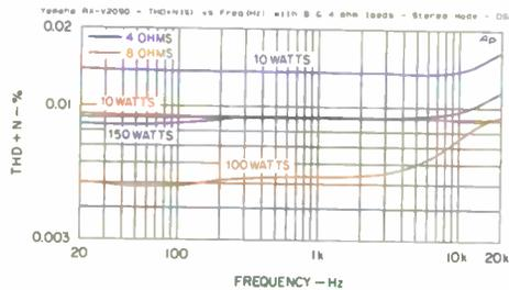
**Fig. 1—Receiver's THD + N vs. frequency, stereo mode. (All graphs presented here are for the RX-V2090.)**
