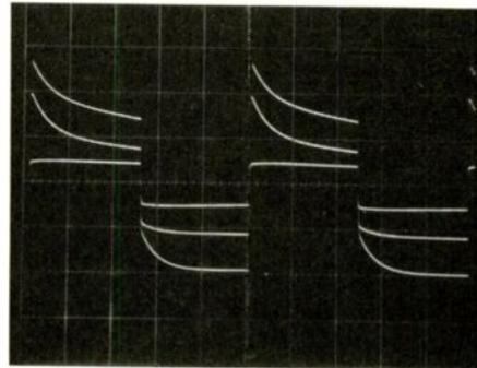
**Fig. 5—Effect of increased drive level into phono section, showing 1 kHz at three different**
