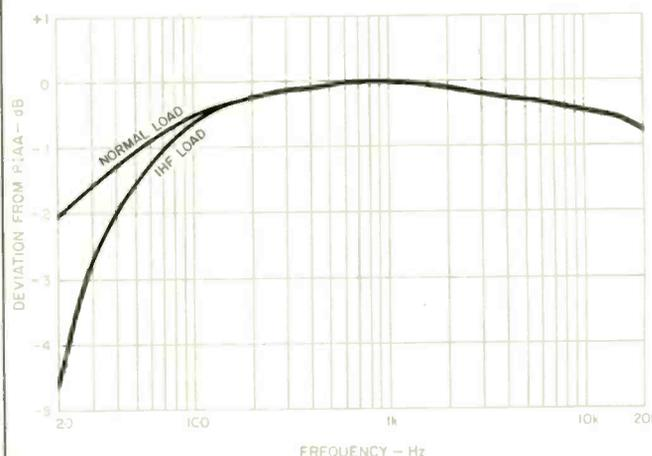
Fig. 3—RIAA equalization error for normal load (90 kilohms and 250 pF) and IHF load (10 kilohms and 100 pF). Shown for right channel, measured at tape output.
