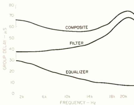
Fig. 4—Group delay of anti-aliasing filter (middle curve); first-order, all-pass phase-equalizer network (bottom curve), and composite response (top curve) of filter and equalizer.
