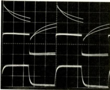
**Fig. 4—Phono-preamp square-wave response: 40 Hz (top), 1 kHz (middle), and 10 kHz (bottom). Dual traces show effects of normal and IHF loads. (Vertical**
