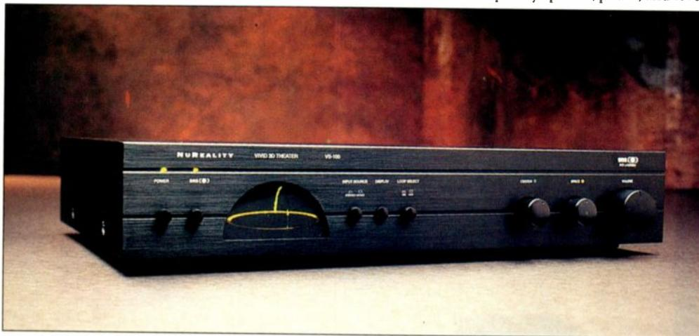
One of the oldest, best-established techniques for doing this is the Sound Retrieval System (SRS), used by NuReality in its series of Vivid 3D processors. Invented by Arnold Klayman, SRS is said to use processing based on the psychoacoustics of head-related transfer functions. These functions help the brain localize sounds precisely, in all directions, because the spectral characteristics, or frequency content, of those sounds vary according to the direc-
