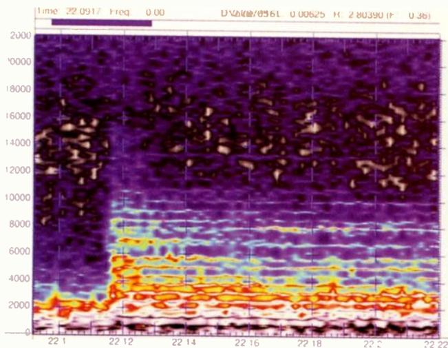
**Fig. 1**—“Three-dimensional” spectrogram of a piano-attack transient after passage through a Sony K-1203 SBM noise shaper. Time is charted horizontally in seconds, frequency vertically in hertz; amplitude is indicated by color (see color key below). Note the slight bulge, or “puff,” from the left edge of the attack’s vertical structure, between about 6 and 8.8 kHz.
