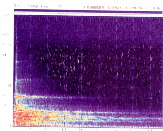
Fig. 11—Spectrogram of the HDCD-encoded rendering of the piano note. Note how the tails of the partials are lengthened and intensified.
