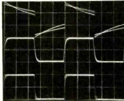
Fig. 7—Line-amp square-wave response: 20 Hz (top), 20 kHz with volume control set 8.5 dB below maximum (middle), and 20 kHz with volume control fully clockwise (bottom). Dual traces
