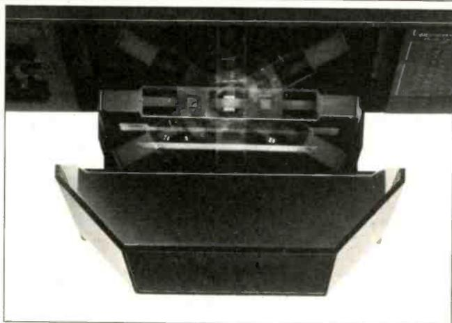
To maintain azimuth accuracy, the RX-505's UDAR (Unidirectional Auto Reverse) system physically reverses the cassette instead of merely reversing the transport's motion.
