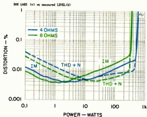
**Fig. 3—THD + N and SMPTE IM distortion vs. power output.**
