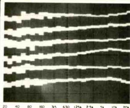
Fig. 2—Forward and “reverse” record/playback responses, overlaid. From top to bottom: EXII tape without NR, EXII with Dolby C NR, SX tape without NR, SX with Dolby C NR, ZX without NR, and ZX with Dolby C NR. (Vertical scale: 5 dB/division.)
