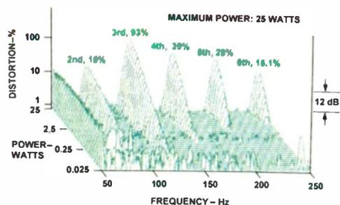
Fig. 7—Harmonic distortion for E<sub>1</sub> (41.2 Hz).
