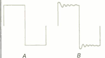
Fig. 2—Square wave before (A) and after (B) phase shift.
