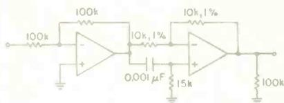
Fig. 6—A first-order, active, all-pass network for correcting group delay of digital recordings.
