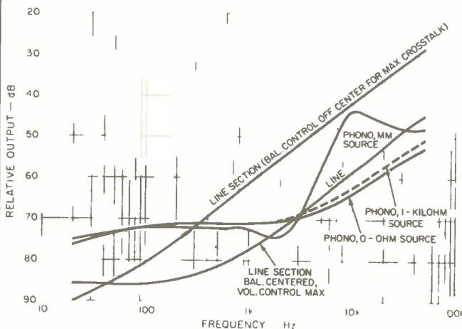
**Fig. 6—Crosstalk vs. frequency for line and phono sections. Note increase in line-section crosstalk when balance control is moved towards driven channel. (The same effect was seen**
