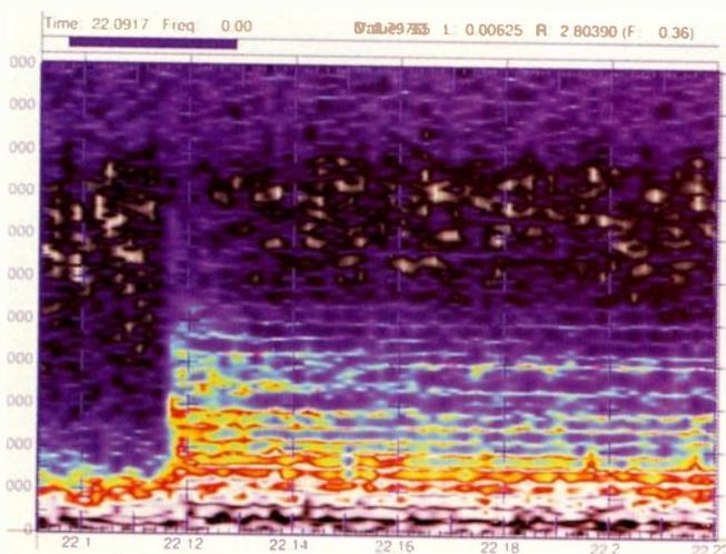
**Fig. 2**—Spectrogram of the same piano attack in Fig. 1, this time processed through an Apogee UV-1000, which uses the company’s UV-22 20-to-16-bit redithering process but no noise shaping. The slight “puff” of energy visible in Fig. 1, ahead of the attack, is absent here.
