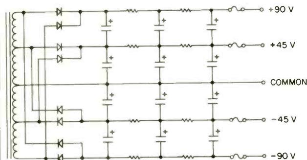
Fig. 2—Power-supply configuration. Four diodes at center form one bridge rectifier, top and
