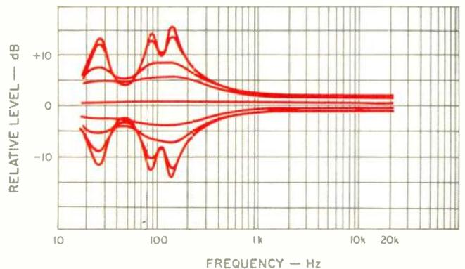
**Fig. 2—Swept-frequency responses with 31.5-, 90- and 125-Hz filters set successively for steps of 3 dB from  $-12$  to  $+12$  dB.**
