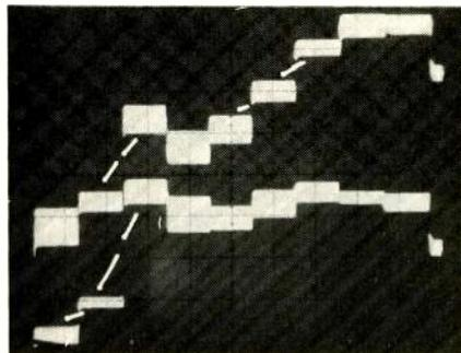
Fig. 6—One-third octave response of stage-monitor loudspeaker before (top curve) and after (bottom curve) equalization. Vertical sensitivity, 5 dB/div.; horizontal,  $\frac{1}{3}$  octave from 25 to 250 Hz.
