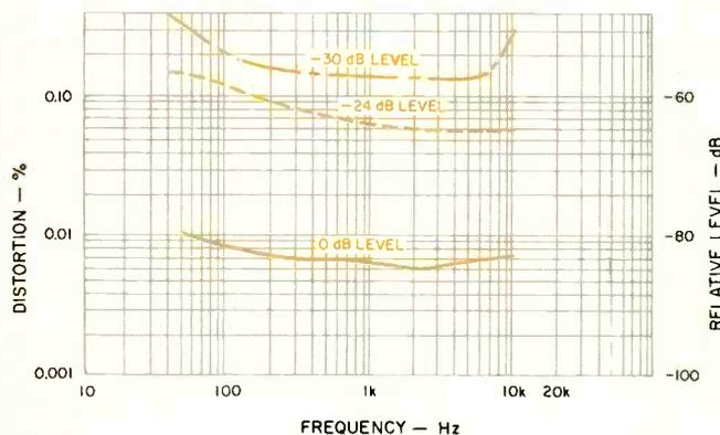
Fig. 2—Harmonic distortion vs. frequency at three output levels.
