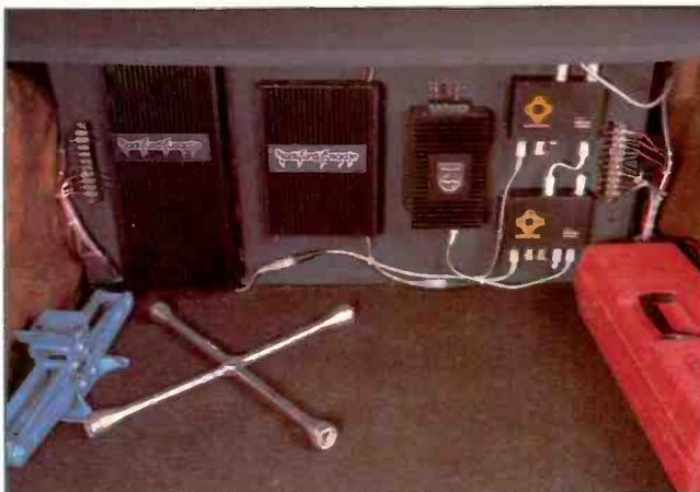
The amp rack on the back of the subwoofer housing. From left to right: Rockford Power VI amplifier for woofers, Rockford Power II amplifier for midrange, Philips EN-2200 amp for tweeters, and two AudioMobile CX-E2 crossovers.
