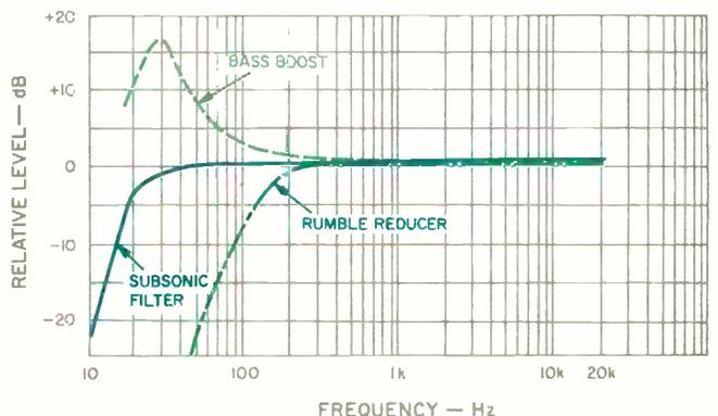
**Fig. 3—Responses of the subsonic filter, the switch-selectable 15 dB boost at 34 Hz, the rumble reducer with out-of-phase signals.**
