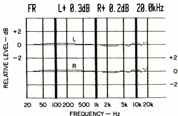
**Fig. 1—Frequency response, left channel (top curve) and right channel (bottom curve).**
