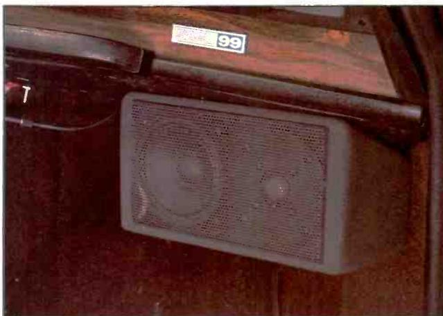
This custom-built enclosure holds an Audax midrange and dome tweeter, each powered by a separate amp.
