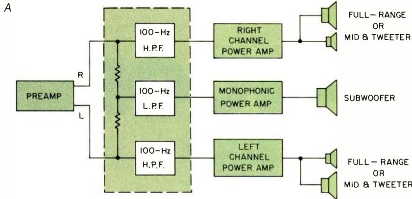
Fig. 1—System connections for center-channel woofer, using monophonic amplifier (A) or stereo amplifier (B) for center channel.
