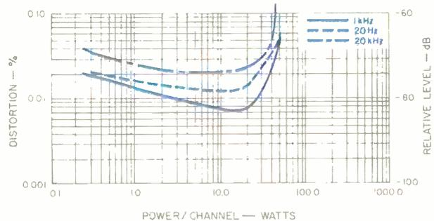
Fig. 1—Power output vs. THD.
