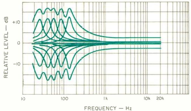
**Fig. 1—Swept-frequency responses of each filter and with all sections at maximum boost and maximum cut, boost and maximum cut,**
