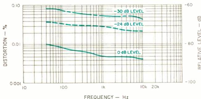
**Fig. 2—THD vs. frequency, at three output levels.**
