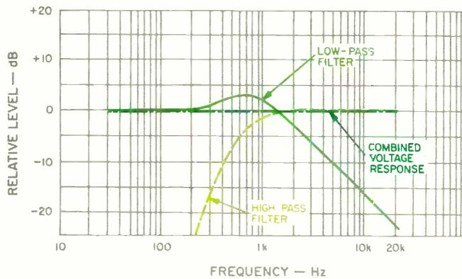
Fig. 4—Responses of the low- and high-pass filters, and their combined voltage response.
