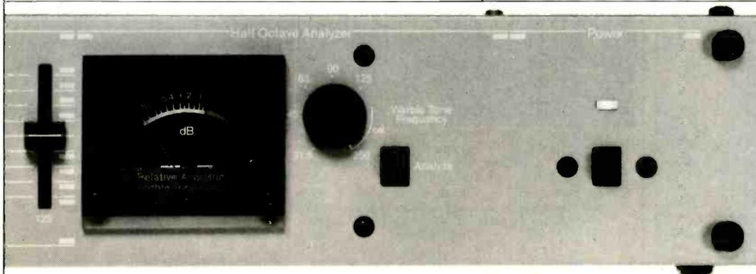
The analyzer section features a highly damped level meter and a warble-tone generator whose frequency is adjustable.
