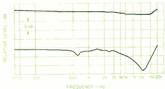
Fig. 1—Frequency response and separation.
