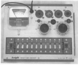
Figure 1. The Knight Kit 400A service-type tube tester by Allied Radio purchased at a Ham swap meet for two dollars.
