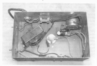
Figure 2. An interior view of the Long fence charger. Note the radio parts used. The metal cabinet measures 9%" x 6" x 4".
