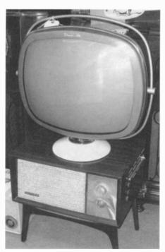
This Philco Predicta, selling for \$225, is the model with the remote console (bottom) which can be separated from the picture tube. A long, flat, multiconductor cable connects the two units.
