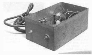
Figure 1. A Long fence charger with the cover off, circa 1940, made when radio parts were no longer available.
