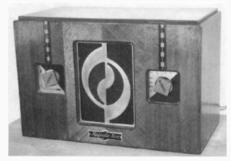
Figure 6. The Model 411, although called the Majestic-Six, has a 5-tube circuit.
