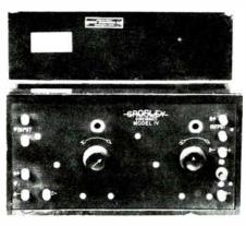
THE CROSLEY MODEL IV (FOUR) WAS A 2-STAGE AMPLIFIER THAT SOLD FOR \$20 IN LATE 1923. IT WAS DESIGNED TO PAIR UP WITH CROSLEY'S MODEL V (AND LATER MODEL 51) AND SHARED THE SAME CABINETS... AND WAS IDENTICAL TO ITS COUSIN, THE ACE 2-B.
