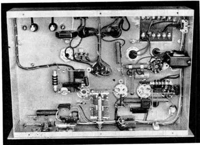
• *There is no hay-wire under the chassis, and the workmanship is not of the rat's-nest variety. Small components are secured to tie-strips and much of the wiring is cabled and laced.*
