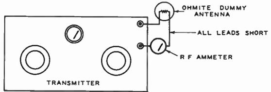
Fig. 3—Dummy Antenna Replacing Untuned Line
