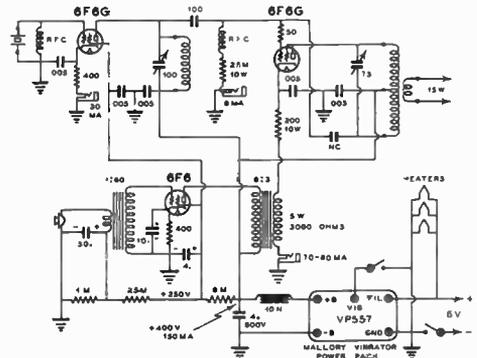
or from a 6.3 volt a.c. power transformer. Standard plug-in coils of the *B & W* type are suitable for the band of operation desired.
