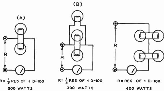
Fig. 4—(A) For 200 Watts. (B)—300 Watts. Fig. 5—Connection for 400 Watts (Max.)
