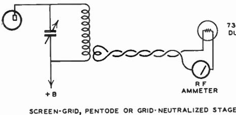
Fig. 8—Screen-Grid, Pentode or Grid Neutralized Stage
