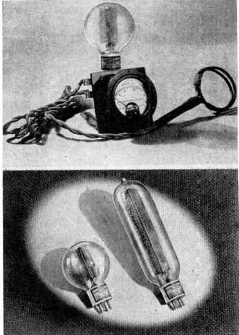
The upper illustration shows an Ohmite Dummy Antenna Resistor, Ammeter and Link Assembly for measuring transmission line losses. The lower illustration shows two Ohmite Dummy Resistors, one for low power measurements, the other for high power (upper illustration referred to as Fig. 9 in text).
