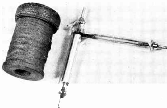
**A** NEW development in antenna changeover relays is the high-vacuum type, illustrated in the photograph. This device will also find numerous other switching applications, because of the high values of voltage which can be broken without danger of external sparking.
