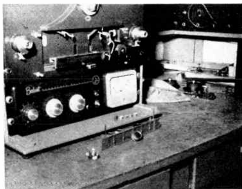
Above: The testing and aligning of tape heads on a mounting bracket. Below: head bracket removed from the machine (it will accommodate five heads for a wide variety of playback flexibility).
