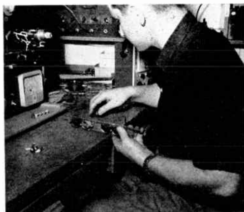
Above: The testing and aligning of tape heads on a mounting bracket. Below: head bracket removed from the machine (it will accommodate five heads for a wide variety of playback flexibility).
