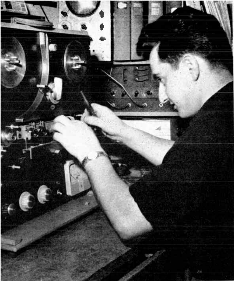
The photograph above shows Sigma's tape expert Bohdan Petryk again, this time hooking up the Stereo triple play head to Kluge's Berlant tape machine.
