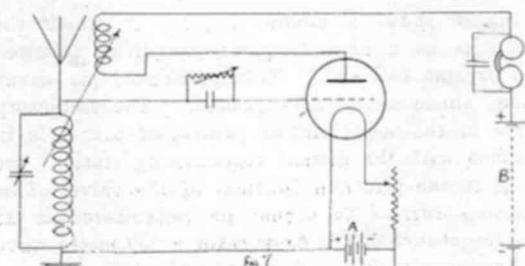
to the filament, thus giving rise to amplified impulses of current in the anode circuit in which are placed the telephone or loud speaker. We now come to the last of the three functions of the valve which was mentioned earlier, viz., rectification.
