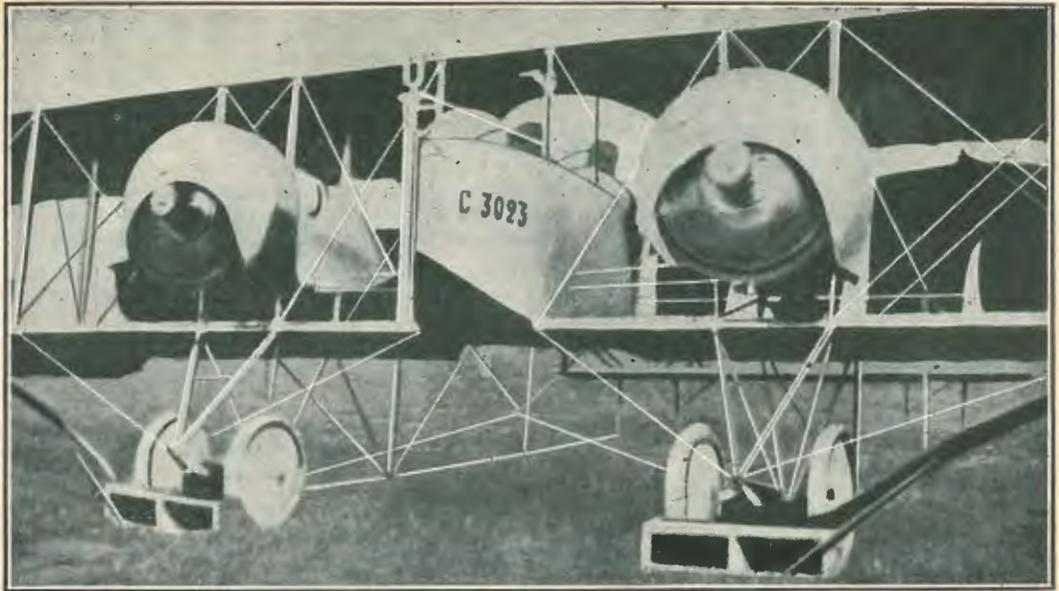
M. Etienne Poulet's Caudron G-4 biplane, showing twin 80 h.p. Le Rhone rotary engines.
