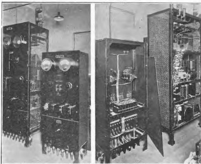
Front and back of Transmitter and Filter Unit at Stations WJY, WJZ and WRC.
