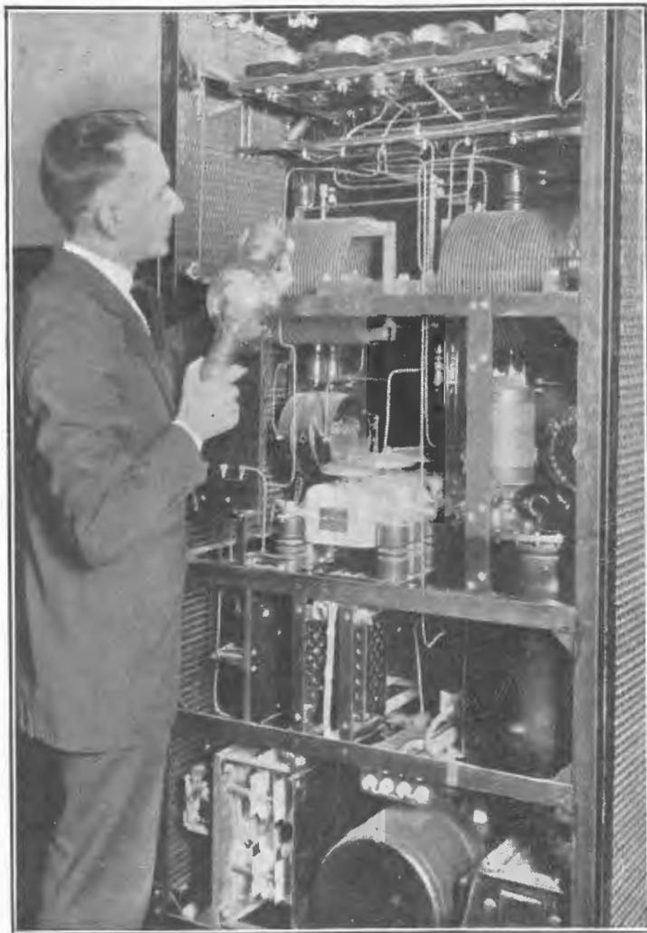
"CLOSE-UP" OF FOUR 250-WATT TUBES AT TOP OF ONE OF AEOLIAN HALL TRANSMITTERS, FROM BACK.
