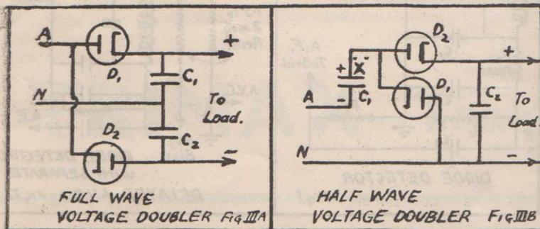
supplies use a H.T. supply of about 100 volts from a half wave rectifier. Voltage doublers cannot be used in A.C.-D.C. receivers.
