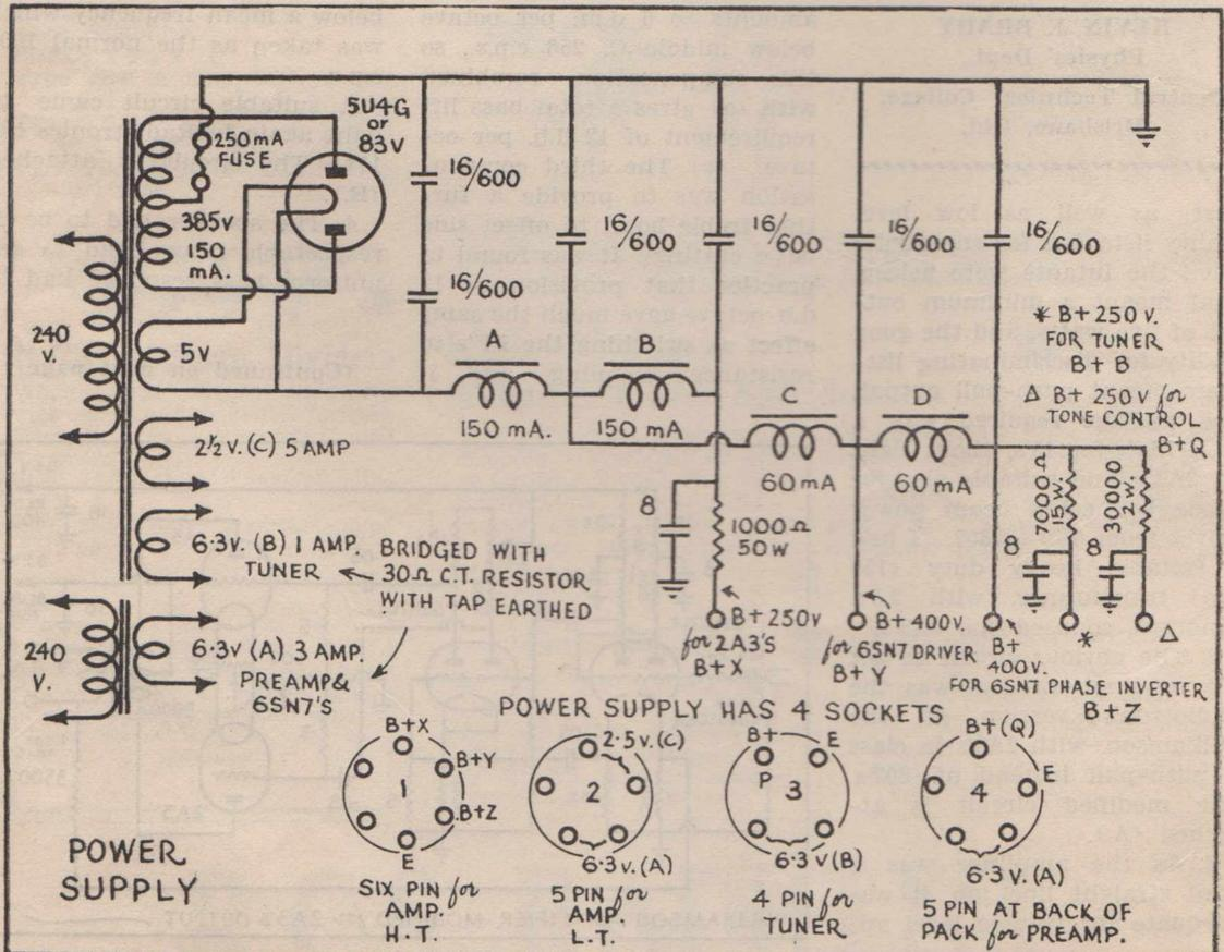
the 2A3's to limit the toasting effect on electrolytic condensers. This hum hunting took by far the most time, but the final arrangement is completely free from any trace of hum, except for a trifle with bass boost fully on and volume at maximum.
