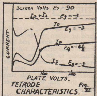
the plate voltage is lower than the screen voltage prevents electrons passing directly to the screen from the plate.
