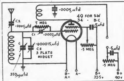
from the control grid lead, aerial condenser, grid winding, grid leak, and grid condenser, as possible, while the 'phone leads must not run anywhere within 4" of the aerial, and if they have to cross it then make the crossing at right angles.
