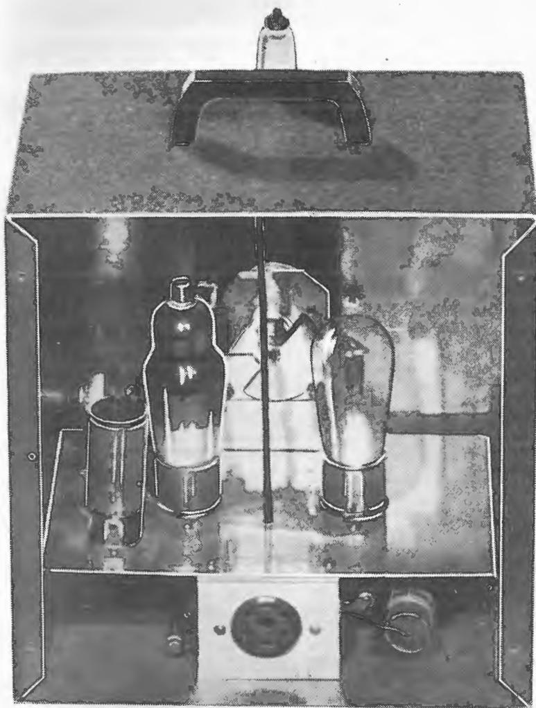
A rear view of the completed instrument. Note particularly the location of the coil, the centre of which should be exactly 2" from the steel back of the cabinet and 1 3/4" from the left-hand side.
