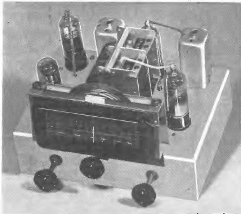
**M**OST notable advance in battery valve technique during the past few years, the new 1.4-volt valves represent an important step forward towards the ideal in battery receiver design. Years ago 6 and 4-volt filaments gave way to 2-volt, and now designers have available a highly successful series of valves requiring only 1.4 volts across the filaments.
