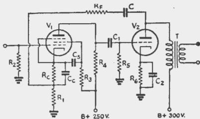
Fig. 4. — Feed-back over two stages.
