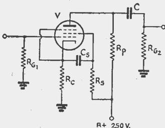
**Fig. 1** — A single-tube current-controlled feedback circuit.
