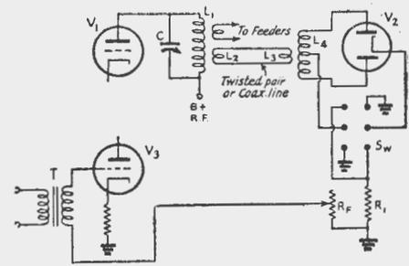
Fig. 7 — Application of negative feedback to a transmitter.
