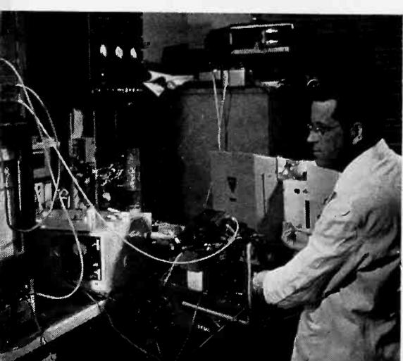
The excitation and emission spectra of crystals are determined with a grating-type spectroradiometer.
