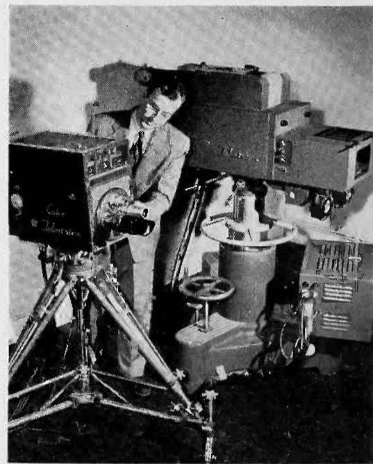
*Brainchild of RCA engineers is this color TV camera, which uses only one pickup tube.*
