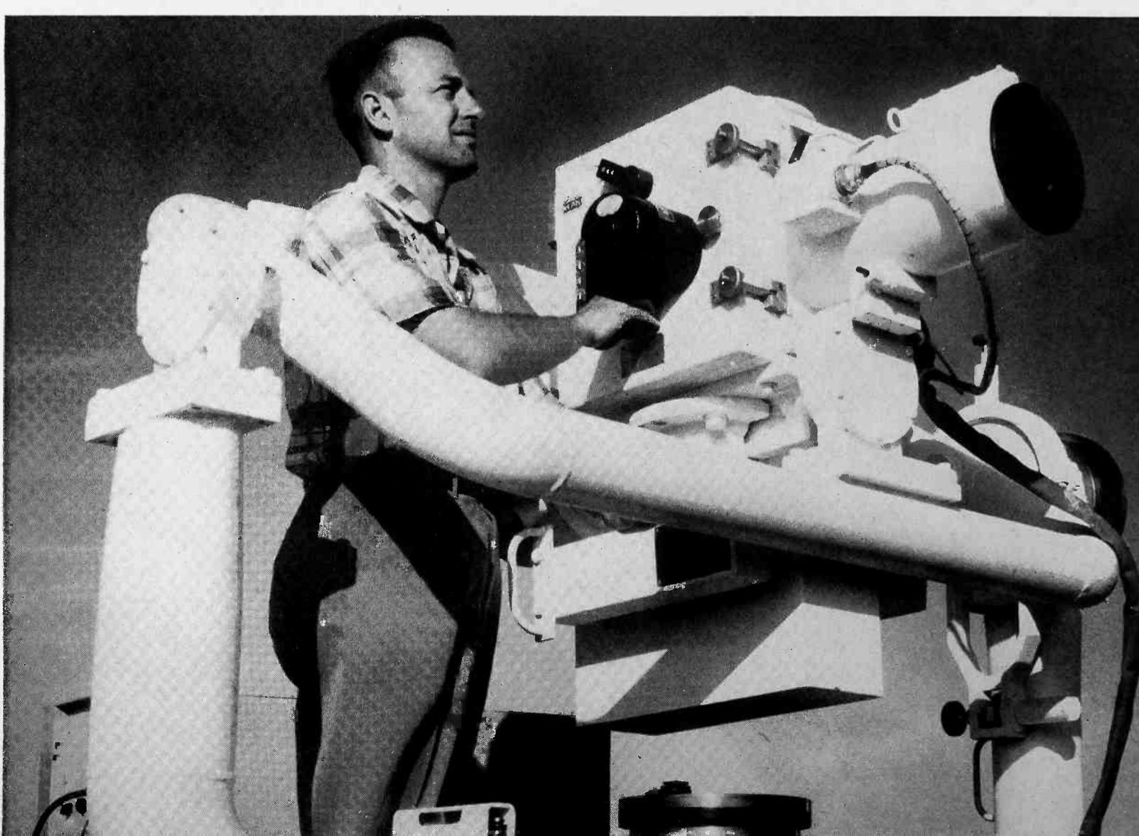
*A modern motion picture camera, equipped with a telescopic lens, is used to track missile flights at Patrick U.S. Air Force Base.*
