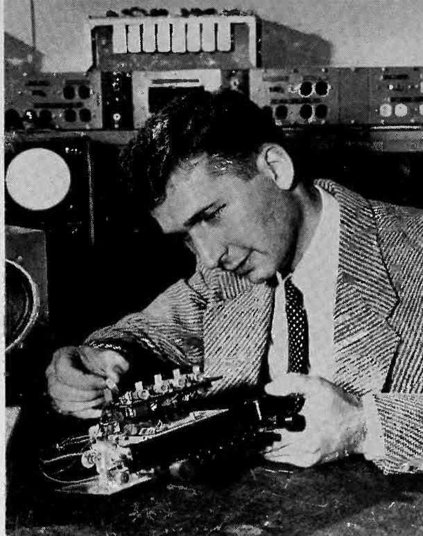
A boon to motorists is this automobile radio, operating from transistors instead of tubes. The transistors operate directly from a 6-volt car storage battery.
