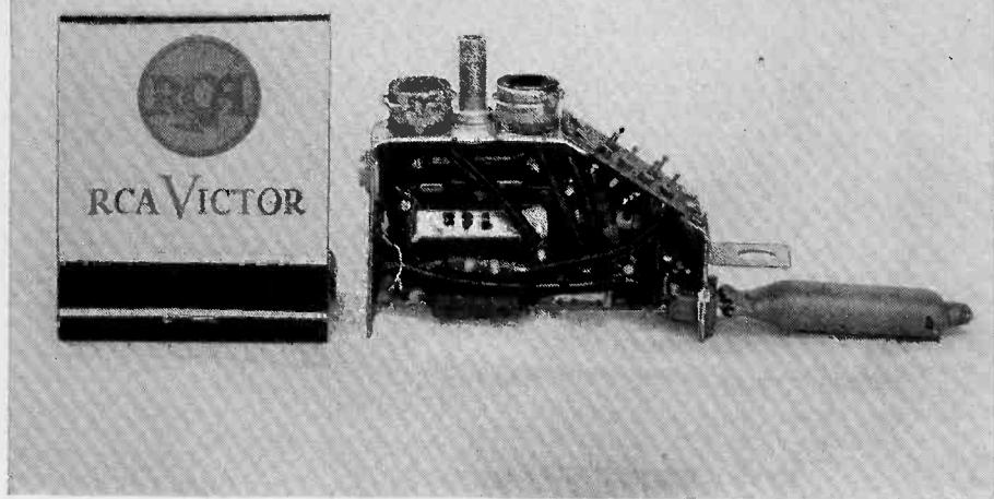
The complete receiver output section of a modern half-size walkie-talkie compared to a match folder. This assembly is a typical result of subminiaturization techniques.
