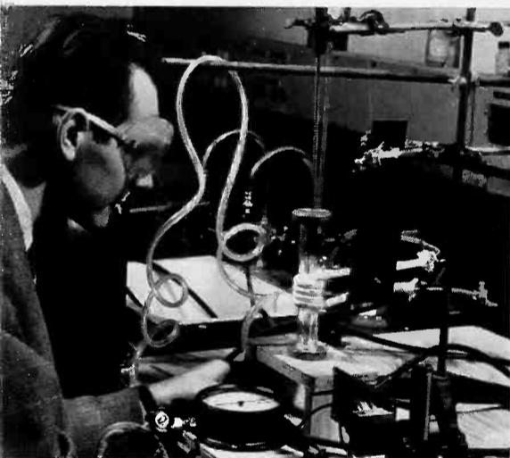
A germanium crystal is grown with the aid of heat generated by a small radio-frequency furnace.
