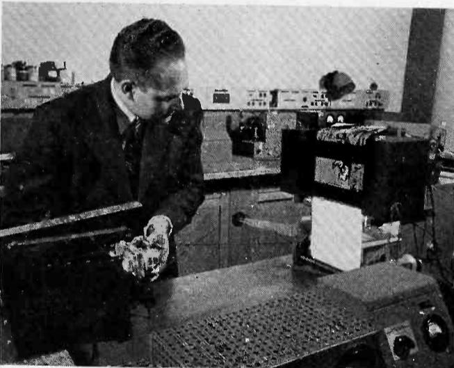
Adjusting a laboratory model of a continuous microfilm enlarger making prints on Electrofax paper.
