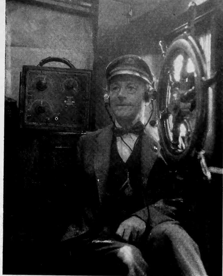
Radio entertainment became available to ships at sea with the introduction of the RCA Radiola II—one of the earliest battery portable receivers.
