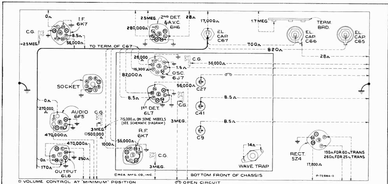
Figure 7—Resistance Diagram
