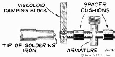
Figure 10—Special Soldering-Iron Tip
