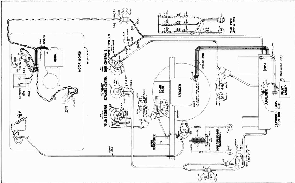
Figure 9—Assembly Wiring
