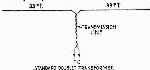
(a) Single Doublet Antenna for 40 Meter Band
