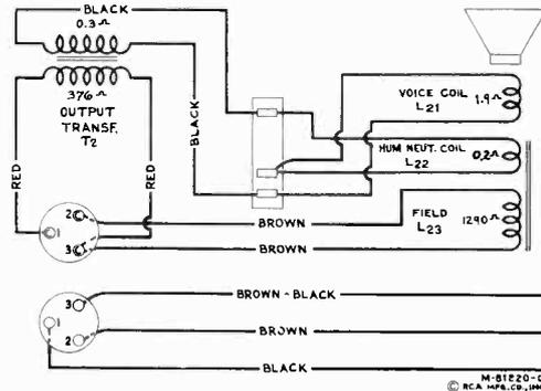
Figure 10—Loudspeaker Wiring
