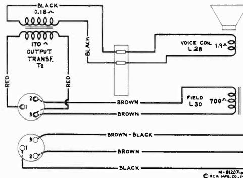
Figure 16—Loudspeaker Wiring
