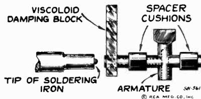
Figure 16—Special Soldering-Iron Tip
