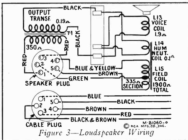
Figure 3—Loudspeaker Wiring
