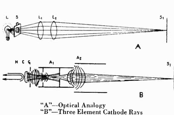
Figure 3—Focusing Cathode Rays
