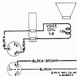
Figure 5—Loudspeaker Wiring
