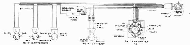
Figure 9—Battery Cable (8BT and 8BK)
