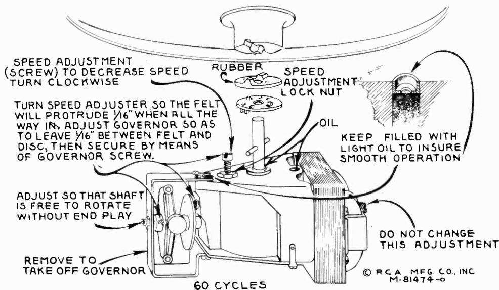
Figure 4—Details of 60-Cycle Motor
