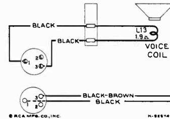
Figure 8—Loudspeaker Wiring
