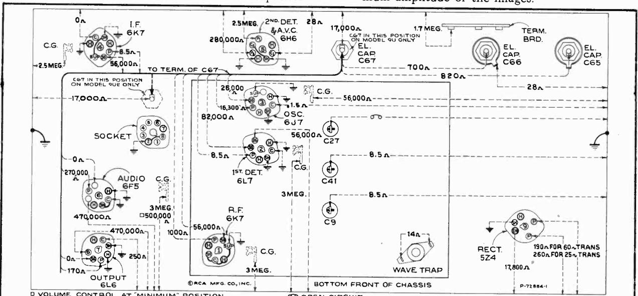
Figure 10—Resistance Diagram
