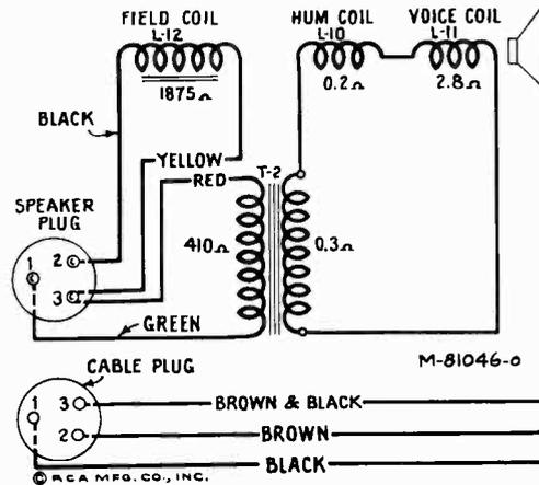
Figure 6—Loudspeaker Wiring
