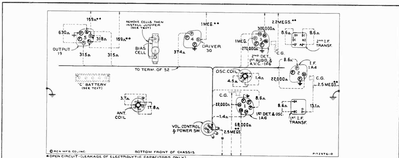
Figure 4—Resistance Diagram
