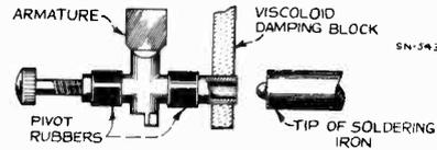
Figure 10—Special Soldering-Iron Tip
