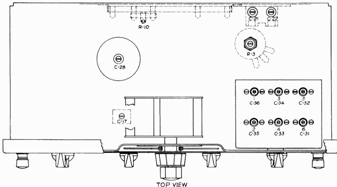
Figure 6—Adjustment Locations (Top View)
