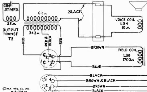
Figure 11—Loudspeaker Wiring
