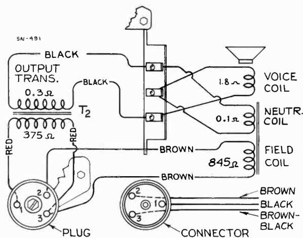
Figure 4—Loudspeaker Wiring
