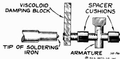
Figure 11—Special Soldering-Iron Tip
