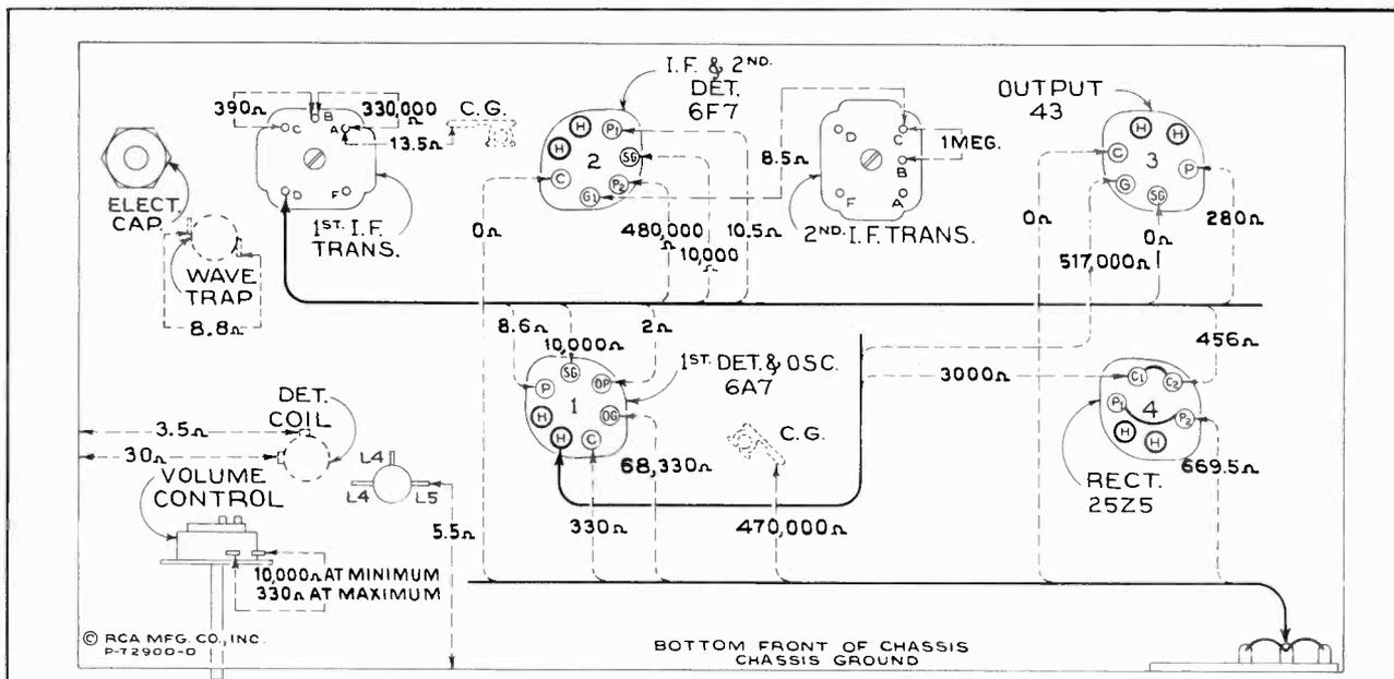
Figure 3—Resistance Diagram
