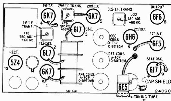
Figure 10—Radiotron and Coil Locations.
