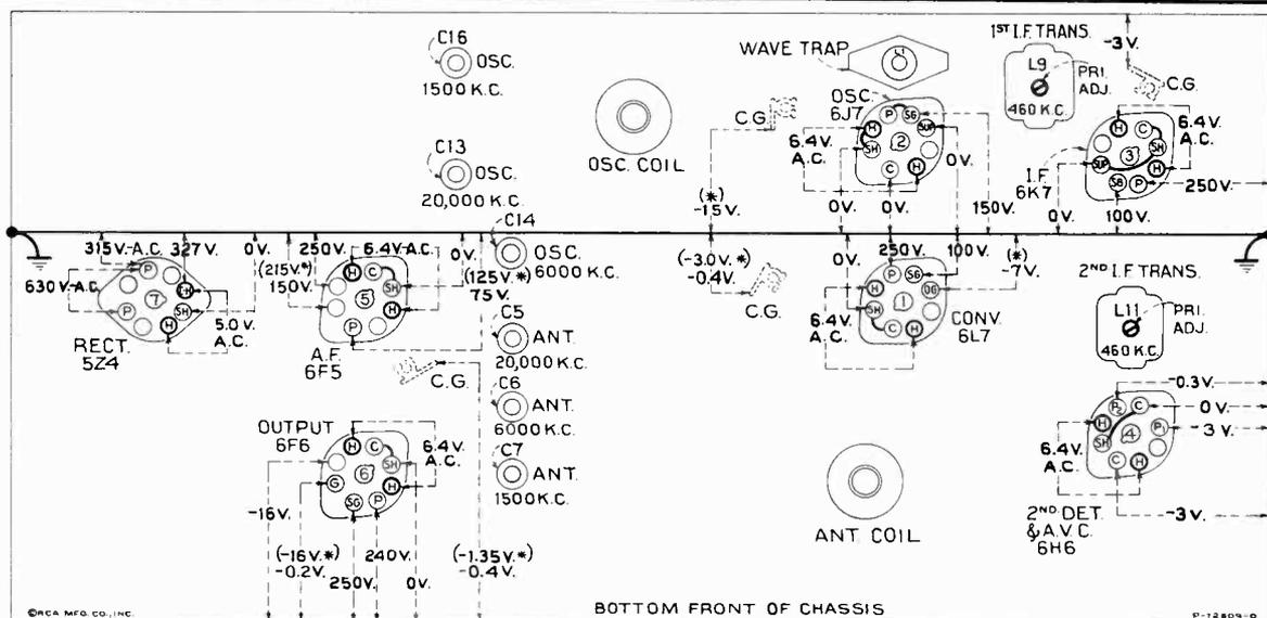
Figure 7—Radiotron Socket Voltages, Coil, and Trimmer Locations
