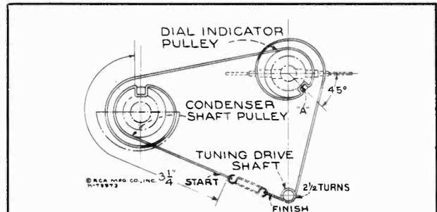
Figure 3—Tuning Drive Cord Mechanism
