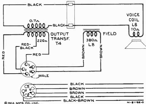
Figure 10—Loudspeaker Wiring
