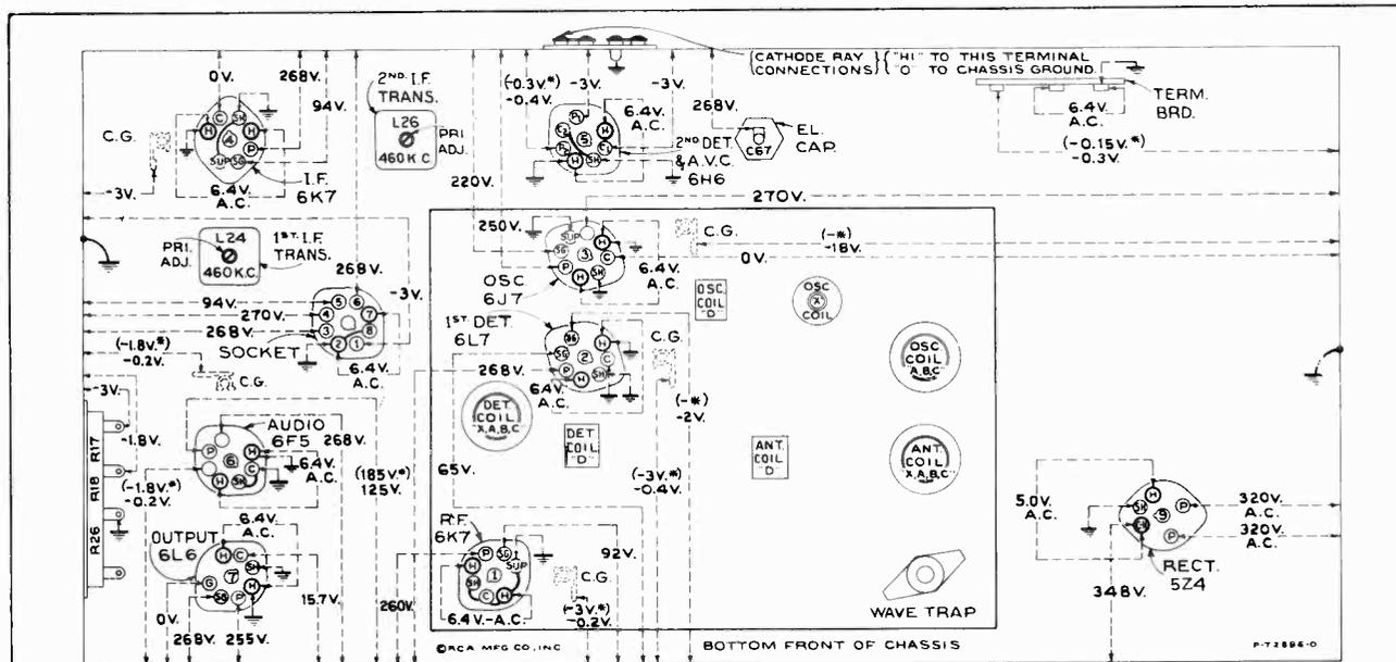
Figure 8—Radiotron Socket Voltages, Coil, and I-F Trimmer Locations
