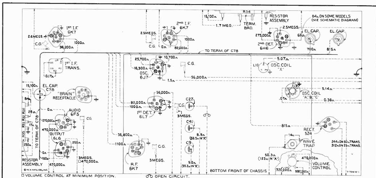
Figure 7—Resistance Diagram
