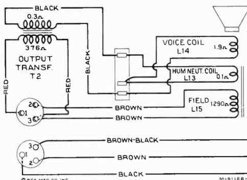
Figure 5—Loudspeaker Wiring
