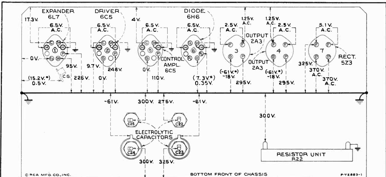
Figure 7—Radiotron Socket Voltages
