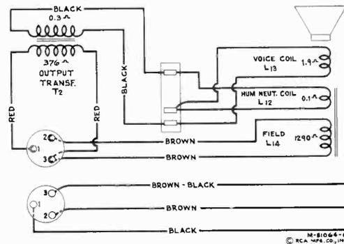
Figure 6—Loudspeaker Wiring
