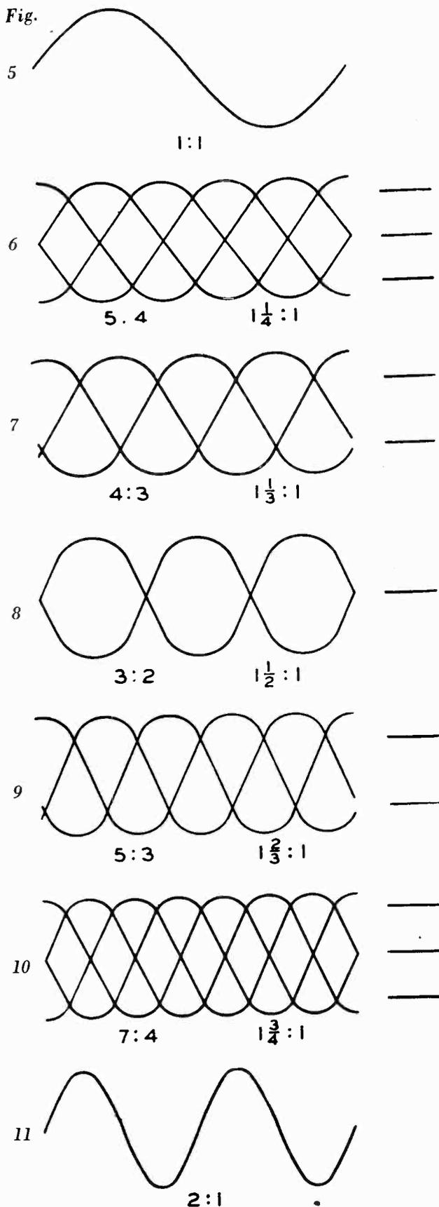
are the ratio of unknown voltage frequency to "saw tooth" oscillator frequency.
