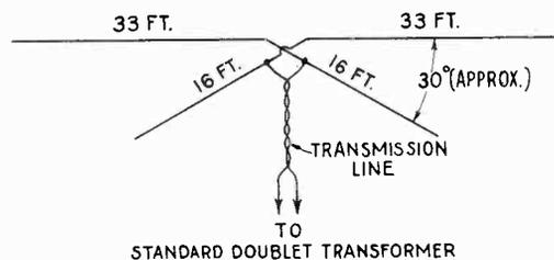
(b) Double Doublet Antenna for 40 and 20 Meter Bands
