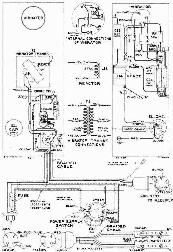
Figure 5—Power Unit Wiring (8BT6 and 8BK6)
