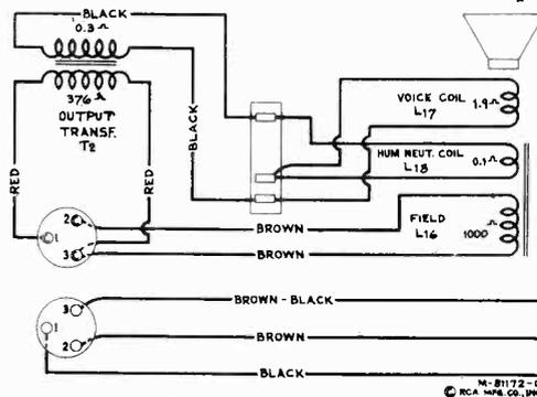
Figure 6—Loudspeaker Wiring
