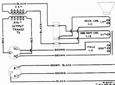
Figure 5—Loudspeaker Wiring
