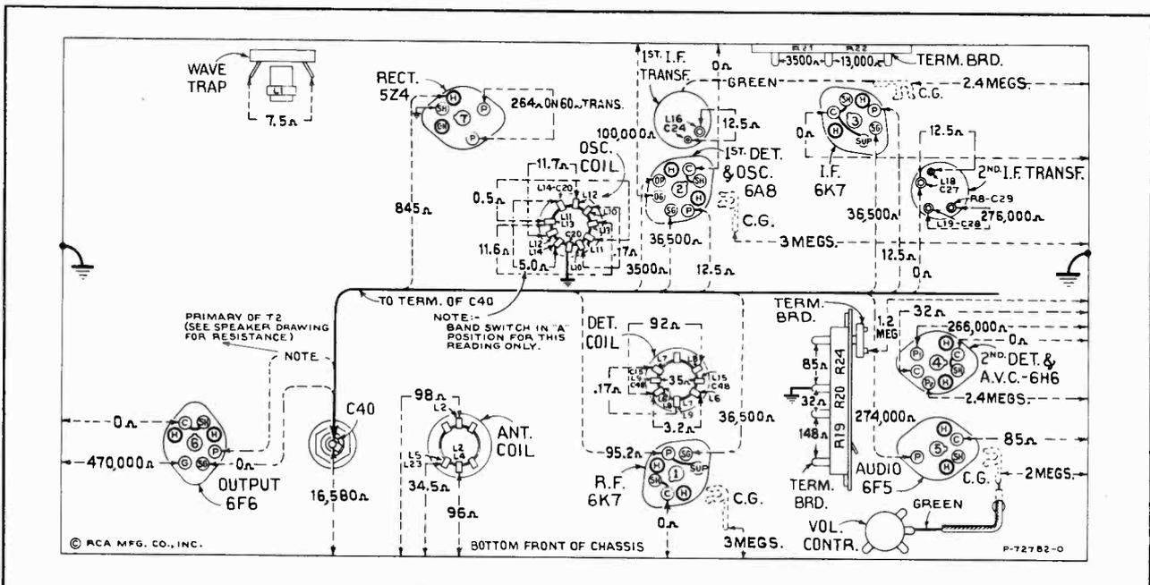
Figure 4—Resistance Diagram
