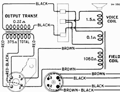
Figure 5—Loudspeaker Wiring
