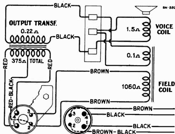
Figure 5—Loudspeaker Wiring
