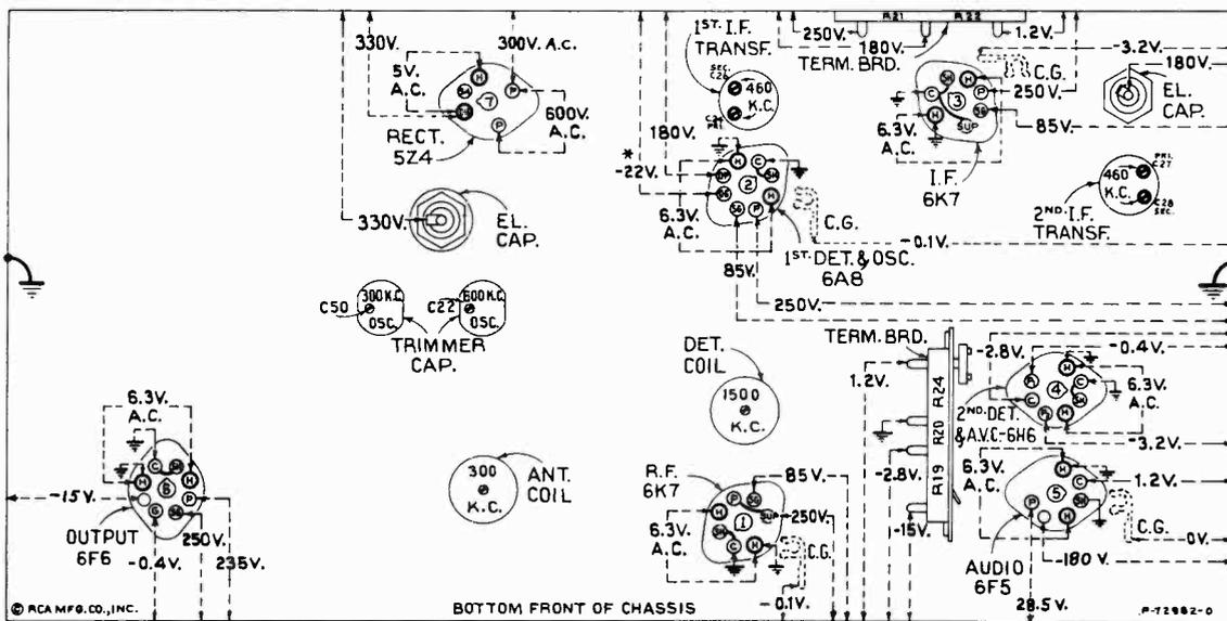
Figure 6—Radiotron Socket Voltages, Coil, and Trimmer Locations
