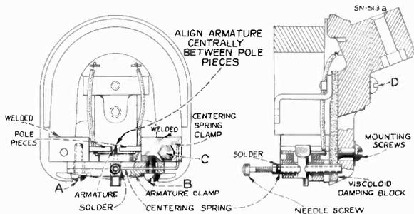
Figure 13—Details of Pickup
