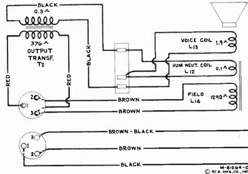
Figure 6—Loudspeaker Wiring
