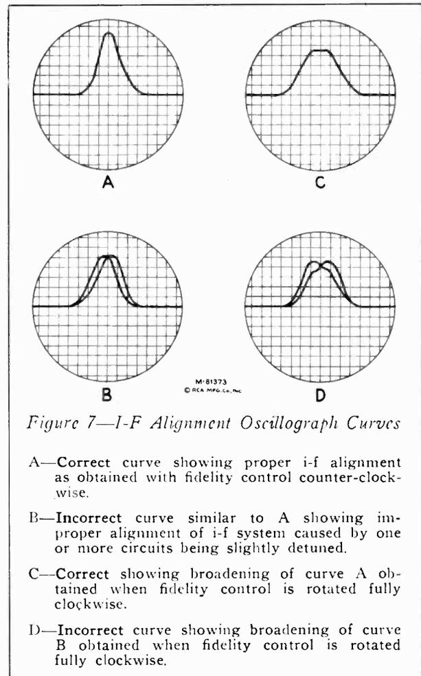
Figure 7—*I-F Alignment Oscillograph Curves*
