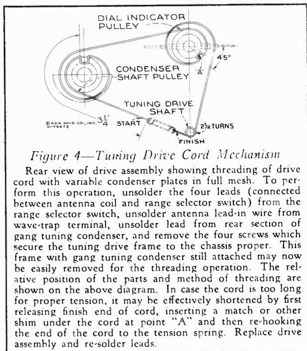
Figure 4—Tuning Drive Cord Mechanism
