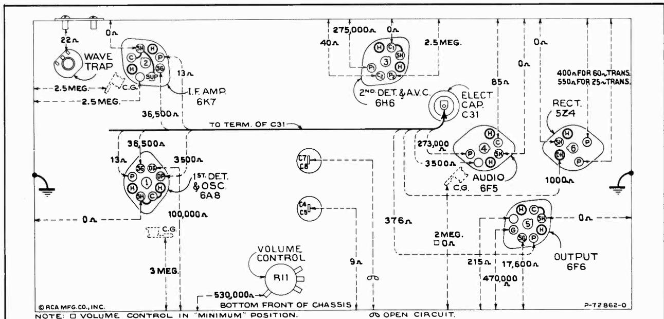
Figure 4—Resistance Diagram
