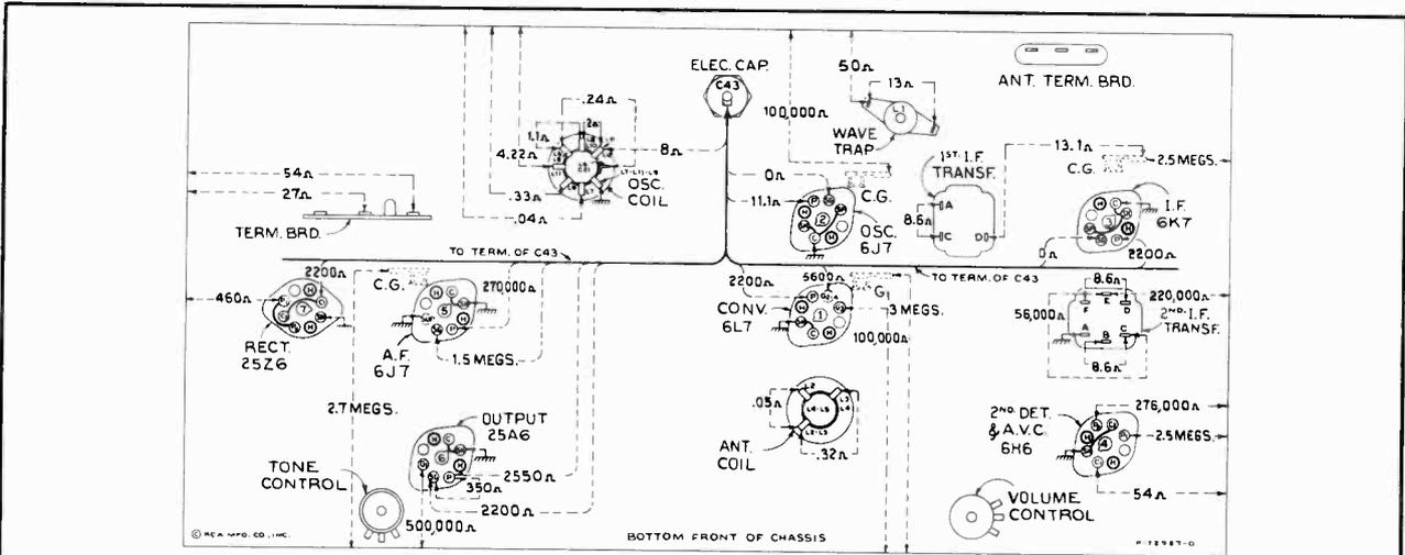
Figure 4—Resistance Diagram
