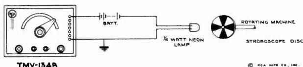
Figure 6—Stroboscopic Speed Measurements
