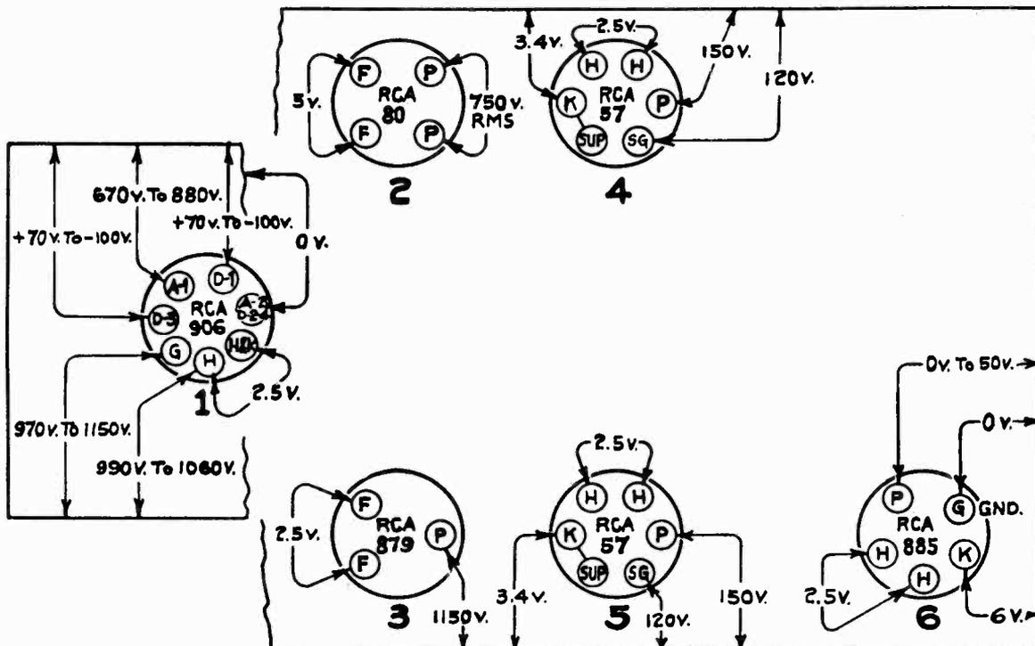
Figure 1—Radiotron Socket Voltages (Bottom View)
