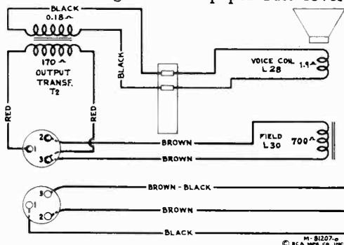
Figure 10—Loudspeaker Wiring
