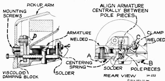
Figure 10—Details of Pickup
