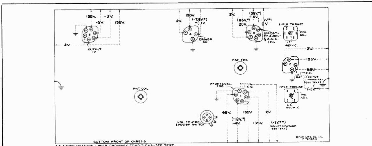
Figure 6—Radiotron Socket Voltages, Coil, and Trimmer Locations
