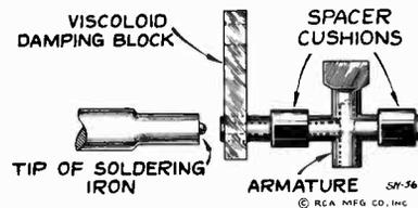
Figure 14—Special Soldering-Iron Tip
