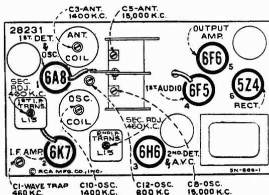
Figure 1—Radiotron, Coil, and Trimmer Locations
