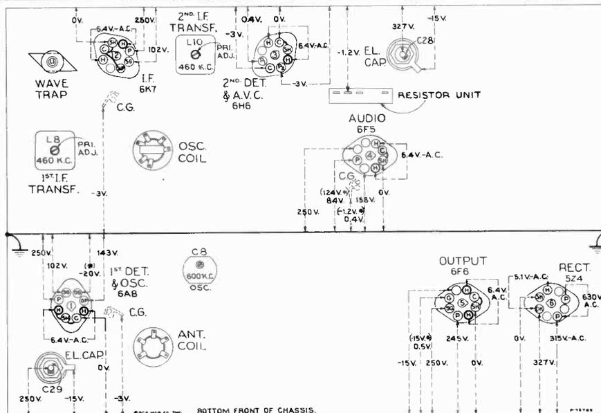
Figure 7—Radiotron Socket Voltages, Coil and Trimmer Locations
