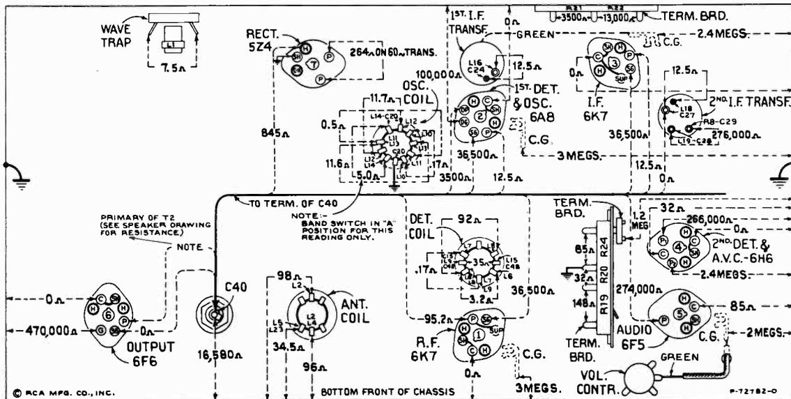
Figure 4—Resistance Diagram
