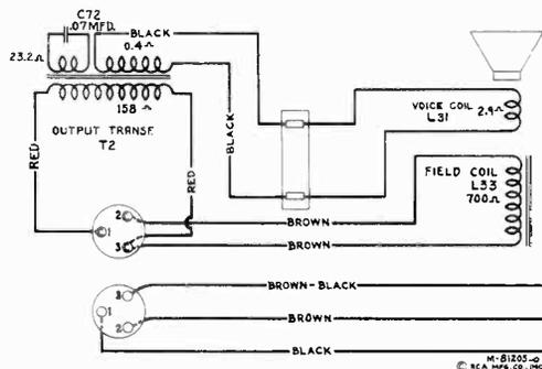
Figure 10—Loudspeaker Wiring
