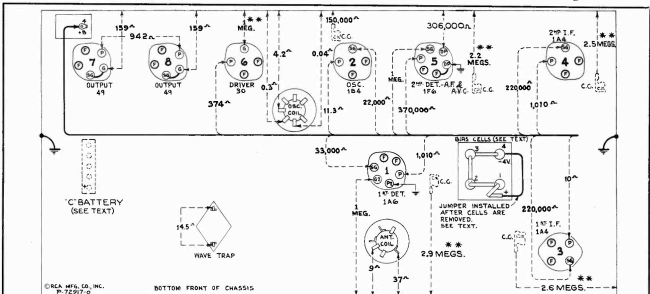
Figure 6—Resistance Diagram
