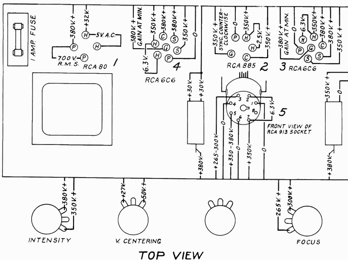
Figure 24—Radiotron Socket Voltage Diagram (Stock No. 151 and 151A)
