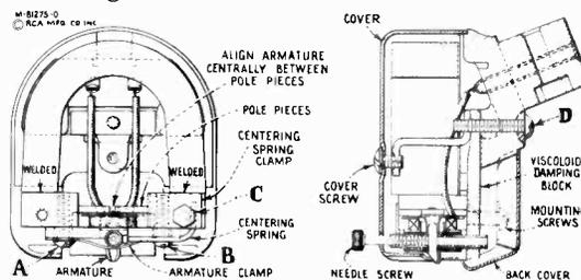
Figure 15—Details of Pickup
