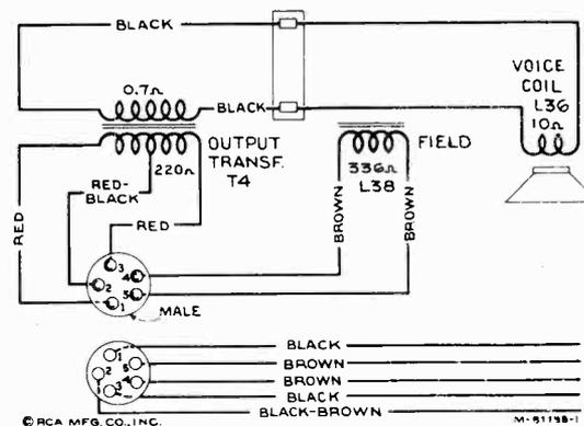
Figure 9—Loudspeaker Wiring
