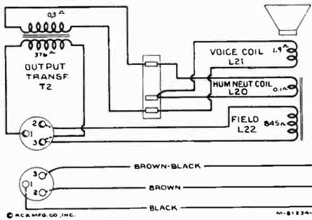
Figure 10—Loudspeaker Wiring
