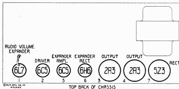
Figure 3—Radiotron Locations
