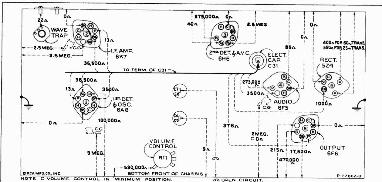
Figure 4—Resistance Diagram
