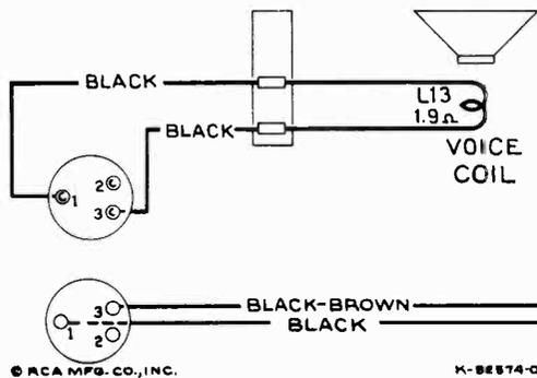
Figure 6—Loudspeaker Wiring
