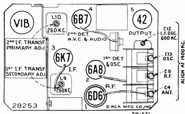
Figure 3—Radiotron, Coil, and Trimmer Locations
