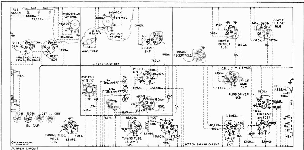
Figure 9—Resistance Diagram
