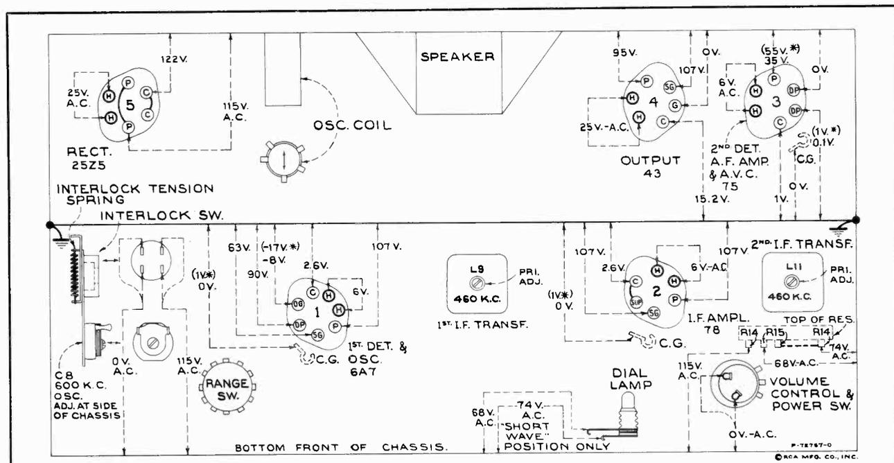
Figure 5—Radiotron Socket Voltages and Trimmer Locations
