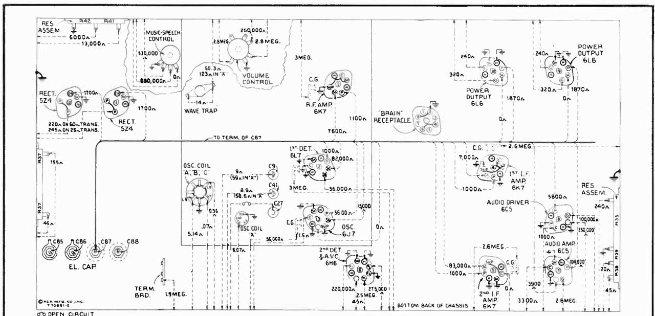
Figure 9—Resistance Diagram
