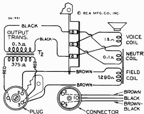
Figure 4—Loudspeaker Wiring
