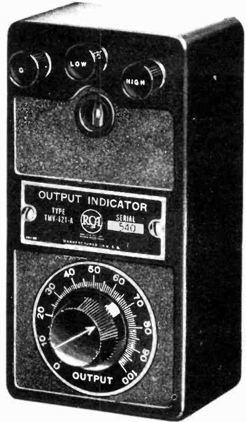
The RCA Output Indicator is a small, compact, visual output indicator designed for use with an oscillator when aligning radio receivers. The instrument consists of a tapped step-up transformer, a potentiometer, a glow tube and three binding posts for connecting the output of the receiver to the transformer. Three input impedances are available, namely, 0.6 ohm, 1.5 ohms and 4 ohms, which cover practically all receivers manufactured.
