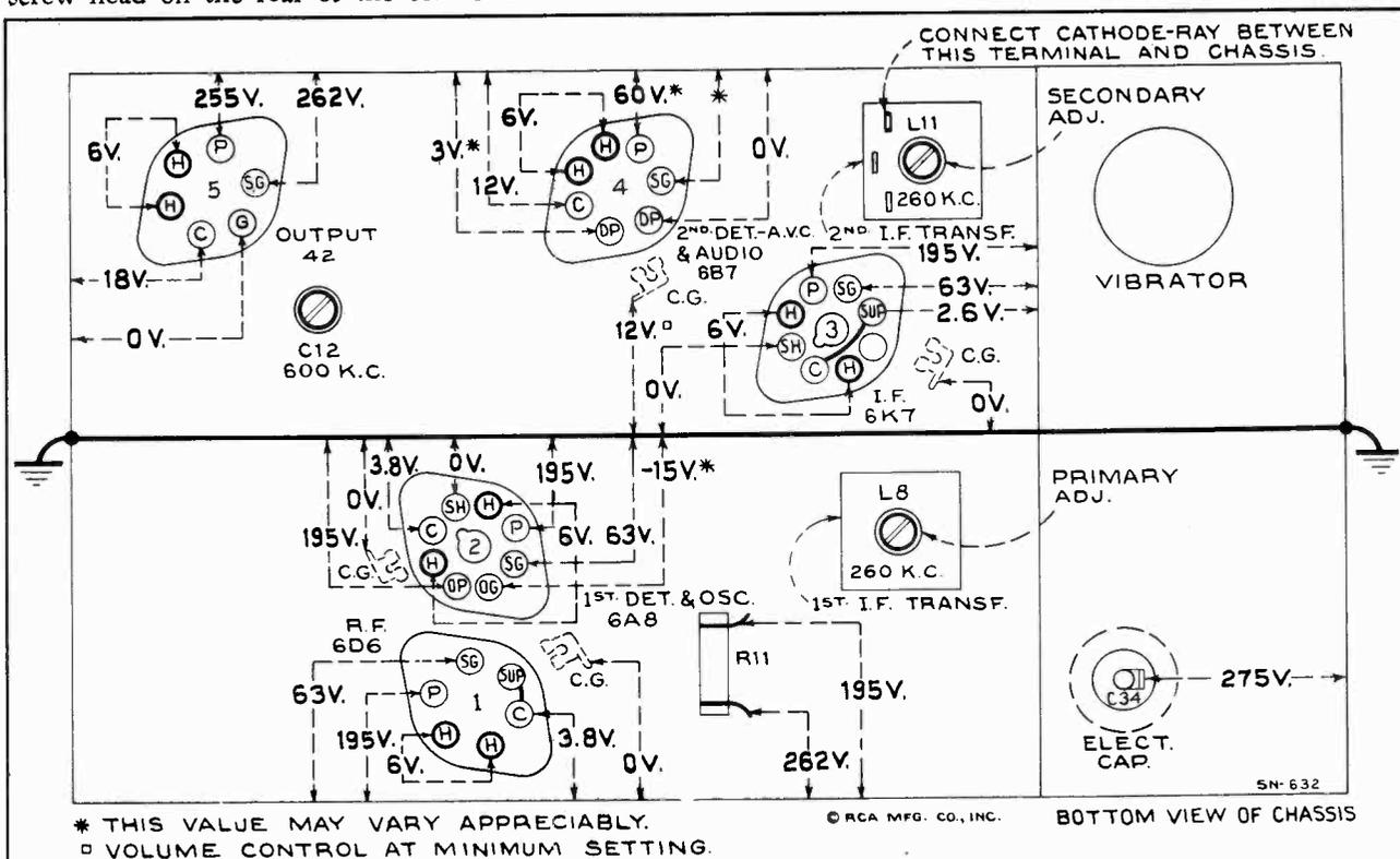
Figure 5—Radiotron Socket Voltages and Trimmer Locations
