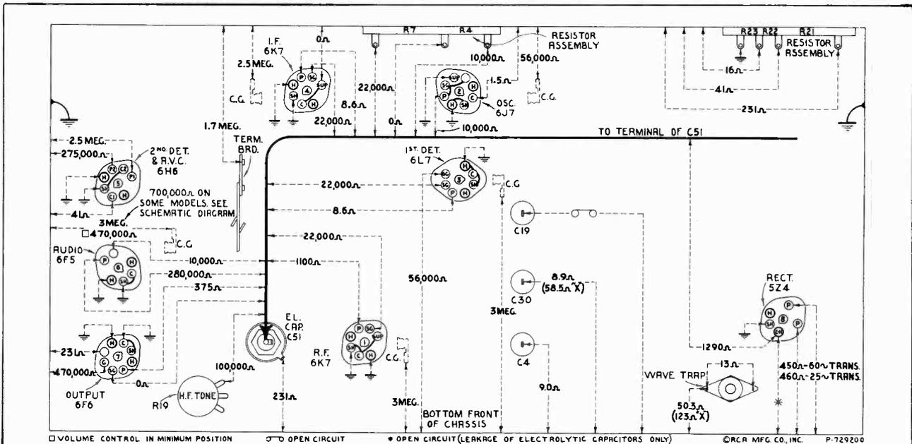
Figure 6—Resistance Diagram
