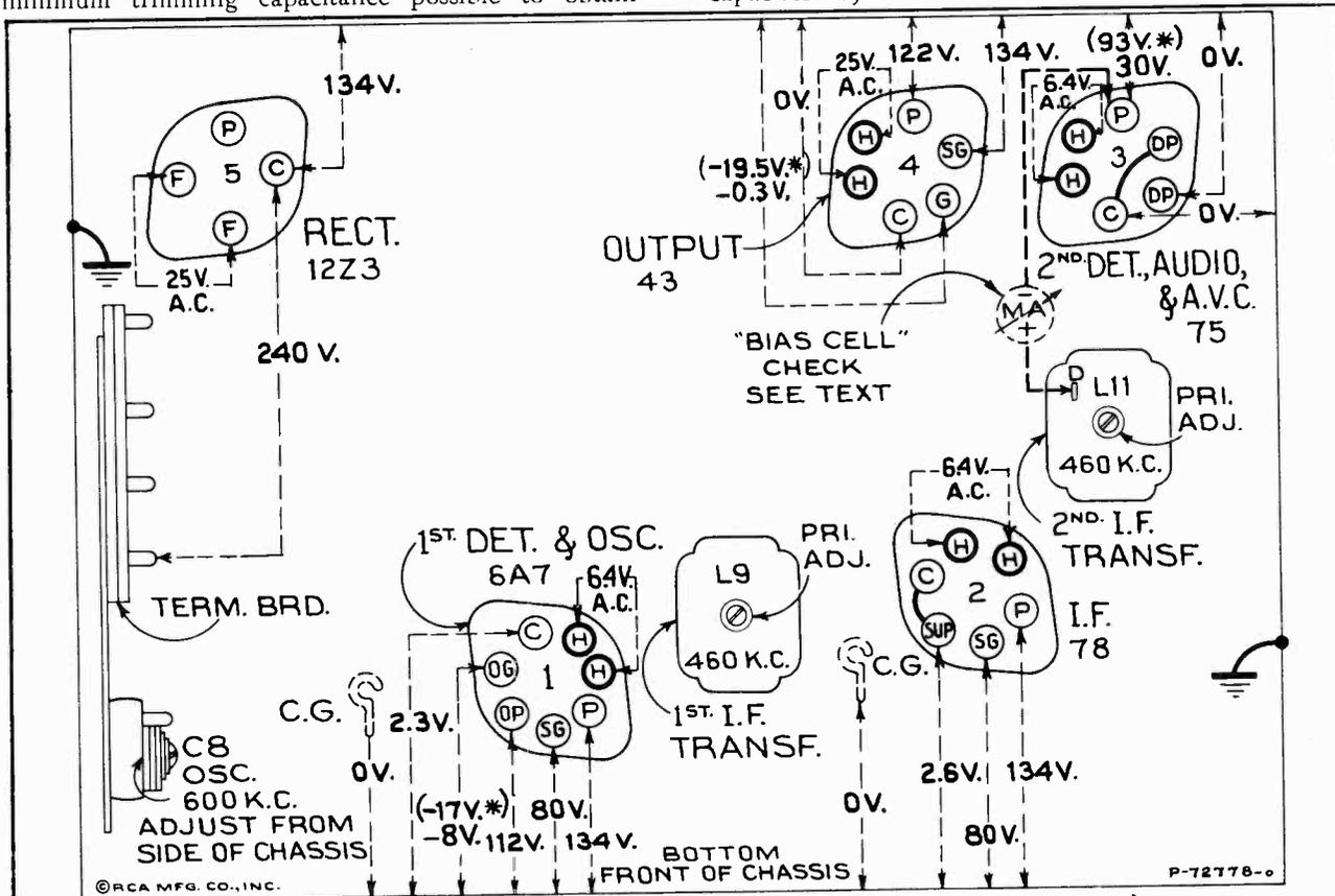
**CAUTION: NEVER CONNECT VOLTMETER TO CONTROL GRID OF TUBE NO. 3 (RCA-75)-SEE TEXT.**
