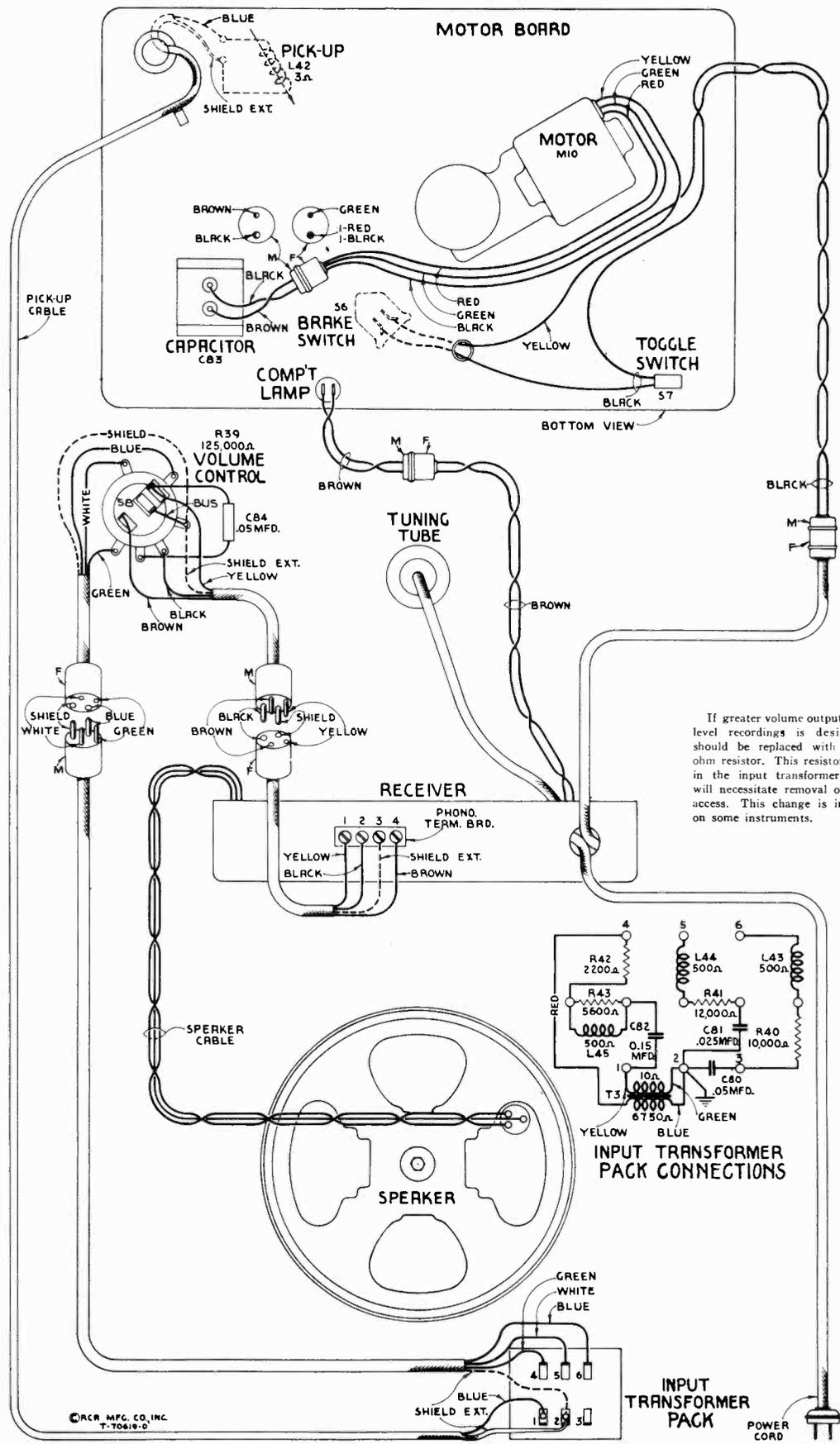
If greater volume output from low-level recordings is desired, R-42 should be replaced with a 10,000-ohm resistor. This resistor is located in the input transformer pack and will necessitate removal of cover for access. This change is incorporated on some instruments.
