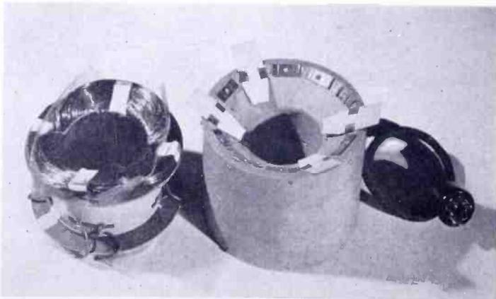
Fig. 11—At left is the unmounted 45-degree multibeam deflection yoke, adapted for machine winding and die forming. The completed yoke, in its case, is shown with four compensating tabs in their approximate operating arrangement, at right.
