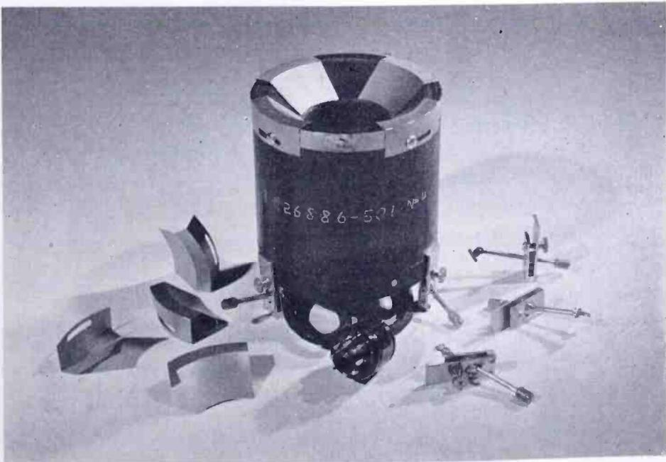
Fig. 5—Section-wound yoke for 45-degree deflection, complete with compensating trimming tabs and beam-alignment magnets.
