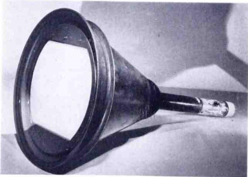
Fig. 1—External view of three-gun tri-color kinescope.
