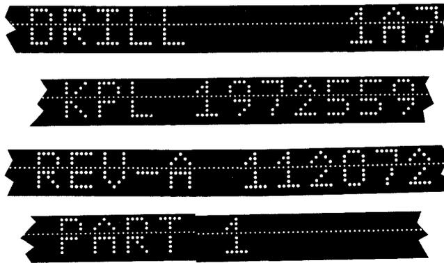
Fig. 9 — Sample of a paper tape identification. Data punched on the leader includes the type of N/C machine (drill, weld, test), the unit code of the board, the key pin list drawing number and revision letter, the same information from the wire net list, if applicable, the computer run date, and the reel number.
