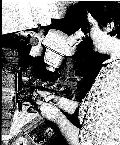
Fig. 4—Grid lineup performed by experienced operator.
