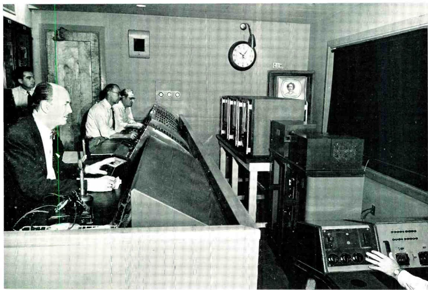
FIG. 9. WKY-TV's Control Room C as rearranged for color operation. Video engineers sit at camera control units at further end of raised platform: color monitors are on table in front of them. Program director sits at console in foreground. Audio position is at lower right corner. Slide camera is just in front of studio window. Color receiver in far corner functions as "on air" monitor.
