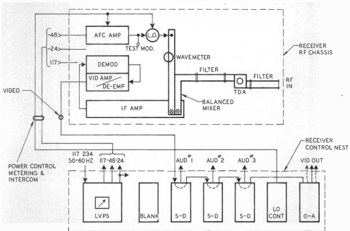
FIG. 10. TVM-6A receiver block diagram showing components in the RF chassis and control units.
