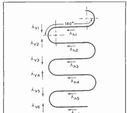
FIG. 4. Zig-zag element showing currents in segments.
