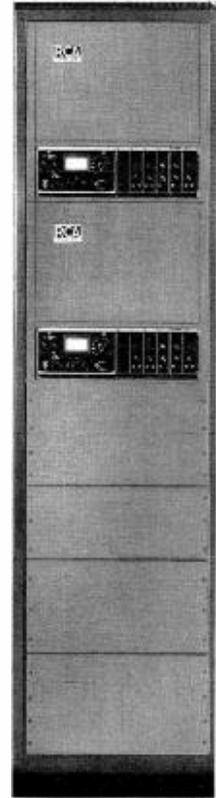
FIG. 1. TVM-6A Solid State TV Relay System packaged for both portable and rack-mounted use.
