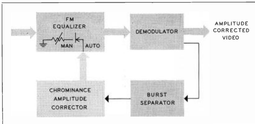
FIG. 11. Block diagram of chrominance amplitude corrector circuitry.
