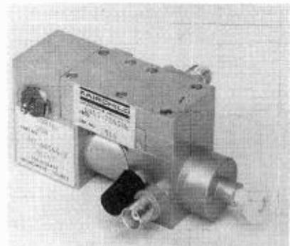
Two additional optional modules that may be used are the low power/low signal indicator that provides an indication of low received RF signal. The other is the video presence indicator, this unit senses the video signal at the receiver control nest.
