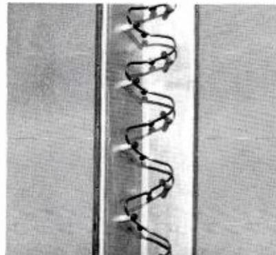
FIG. 8. Zee Panel bent into V-shape.
