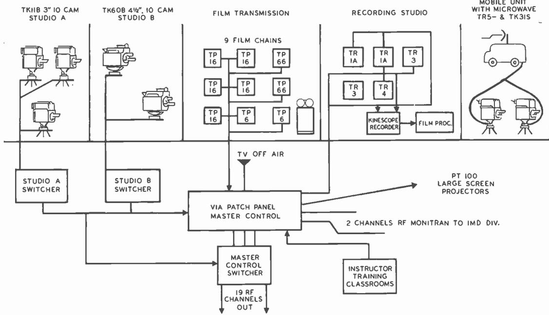
FIG. 27. Block diagram of WFM-TV technical facilities.
