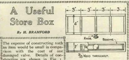
Fig. 3 shows the arrangement of the drawer.
