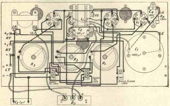
The wiring of the receiver may be followed from this drawing. The connections to the jacks are numbered in accordance with those given in the theoretical circuit diagram. Blueprint No. 102b.
