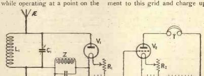
Fig. 5.—The equivalent of the Fig. 4 circuit, two valves being employed in this case to perform the separate functions required. Z, C2 are at the bottom of the anode circuit of V1 for the reasons stated in Fig. 3.
