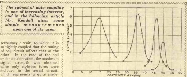
Fig. 3.—These curves express the results obtained by varying the aerial tapping point.
