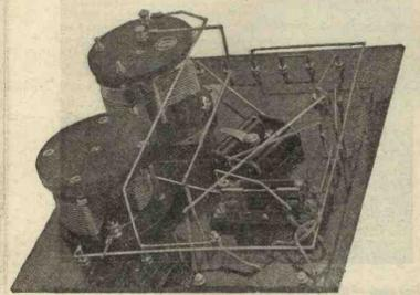
The well-spaced wiring and easy access to the components may be seen from this photograph.
