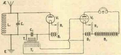
Fig. 6.—A step-up transformer T1 T2 has been substituted here for the choke Z in Fig. 5.
