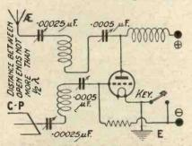
Fig. 3.—Final circuit which met requirements and will oscillate at less than 5 metres.
