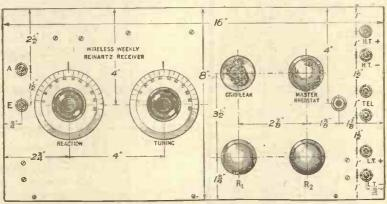
The layout of the panel showing dimensions. Blueprint No. 103a.
