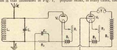
Fig. 3.—Showing a modification of Fig. 2 so that the H.F. component applied to the grid of V2 is eliminated.
