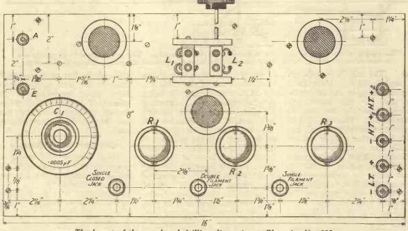
The layout of the panel and drilling dimensions. Blueprint No. 102a.
