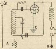
Fig. 4.—The short-wave receiving circuit. The manner in which coil A is connected increases selectivity. This coil in the improved Reinartz circuit was the aerial detuning coil, and in this case is used to couple the aerial coil to the tuner.
