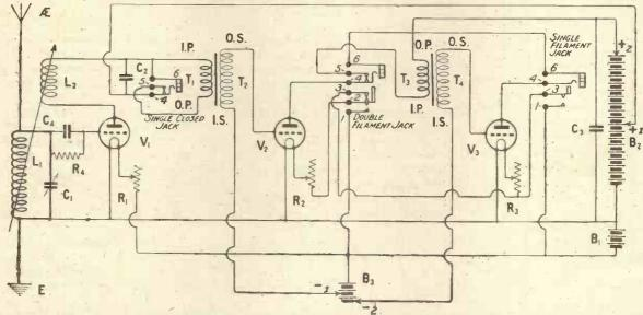
The theoretical circuit. The connections to the facks should be carefully noted, the numbers corresponding with those given in the wiring diagram.
