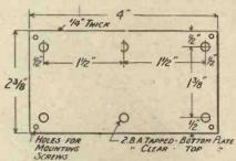
Each end plate is cut to the dimensions shown and afterwards drilled as indicated.
