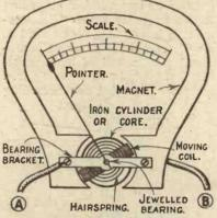
Fig. 1.—Principal working parts of a measuring instrument.
