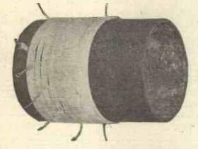
The coil used for theseries of simple tests described in this article was of the single layer variety with a number of tapping points.
