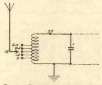
Fig. 2.— The actual connections of the coil.
