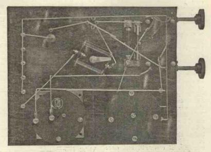
By comparing this photograph of the underside of the panel the actual wiring of the original receiver may be followed.
