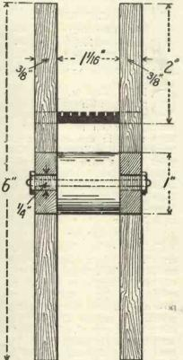
Fig. 5 shows the construction of the coil former.
