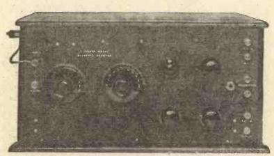
The valves of the receiver are enclosed, accessibility being given by the hinged lid.
