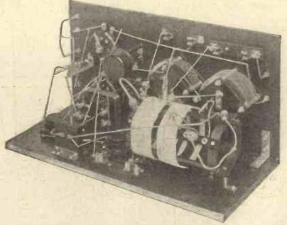
This photograph of the wiring of the receiver also shows the coil with its connections. Note the low-loss former.
