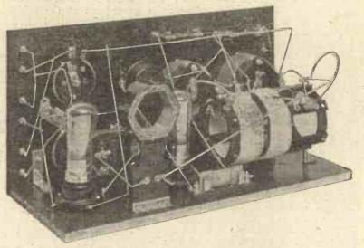
The wiring is well spaced, short and easily carried out.
