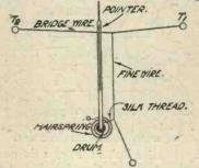
Fig. 3.-Showing principle of the hot wire ammeter.
