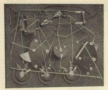
A helpful plan view of the wiring. If used in conjunction with the wiring diagram, all possibility of error is eliminated.
