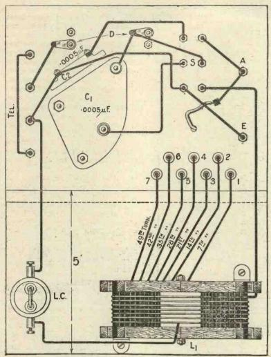
Fig. 8 clearly shows the wiring of the receiver.
