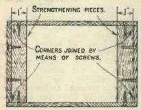
The constructional details of a homemade cabinet.
