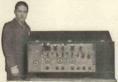
Mr. J. Elliott with the seven-valve T.A.T. he has built. An A.B C. wavetrap which he sometimes uses may be seen on the left.
