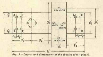
the H.F. transformer, or a readymade valve - holder may be mounted. The holes marked A, B, C, and D are intended for the terminals. The other four, E, F, G and H, are intended to take
