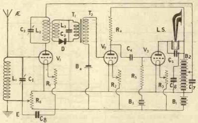
Fig. 1.—In the author's case, the replacing of the valve detector by a crystal results in the circuit shown above.
