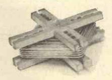
The coil laid upon its side to show how the turns are spaced. Ebonite strips wedged between layers separate these latter in such a way that both turns and layers are air-spaced.
