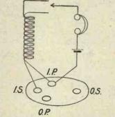
Fig. 2.-How to identify the ends of the windings.
