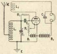
Fig. 1.—A simple auto-coupled circuit in which the aerial is not separately tuned.
