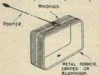
Fig. 2:- The windings and light metal former.
