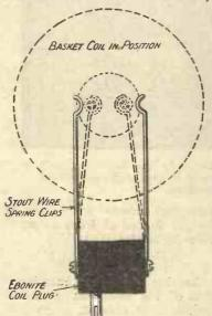
ebonite coil plug in which the connections are made to screws at the sides, two small pillar terminals, some stout copper wire of No. 16 gauge, and some ebonite,  $\frac{1}{8}$  or 3/16 in thick.
