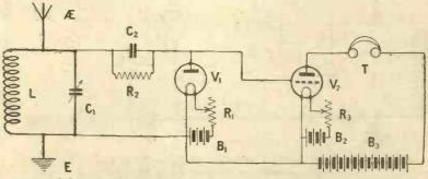
Fig. 2.- In this illustration the detector is a Fleming two-electrode value followed by a three-electrode palue acting purely as an amplifier and serves to explain the function of the Fig. 1 circuit.
