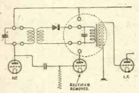
Fig. 6.—The resulting circuit when the crystal is used in place of the valve detector.
