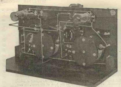
Fig. 4.—The panel is secured to a baseboard by means of two pieces of wood, and may therefore be removed from the box without the necessity of removing screws.
