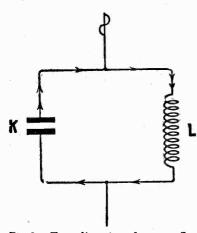
Fig.6.-True direction of current flow in an oscillatory circuit.
