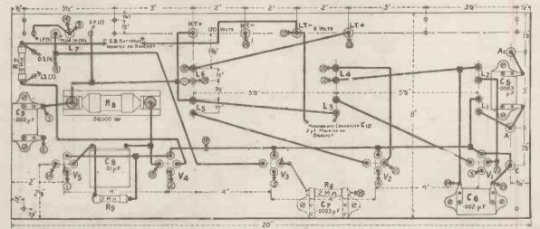
Fig. 3.—The wiring af the underside of the value panel, the lower edge being that which fits against the front panel. Blue print 94c.
