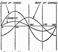
Fig. 2.-Illustrating the relation between magnetic field and its rate of change.
