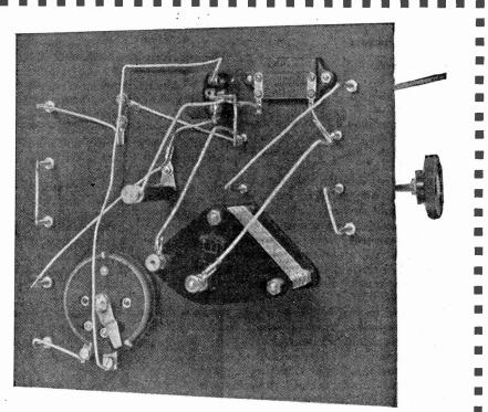
Fig. 3.—Back-of-panel wiring.
