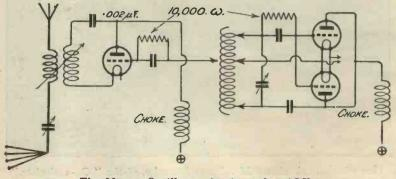
The Master Oscillator circuit used at 2DX.
