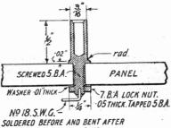
LEG HAS BEEN FIXED IN PANEL. LEADS ARE SOLDERED TO THIS WIRE.
