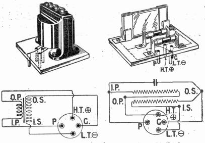
Figs. 5 and 6.—Illustrating how the interchangeable units are mounted and connected.
