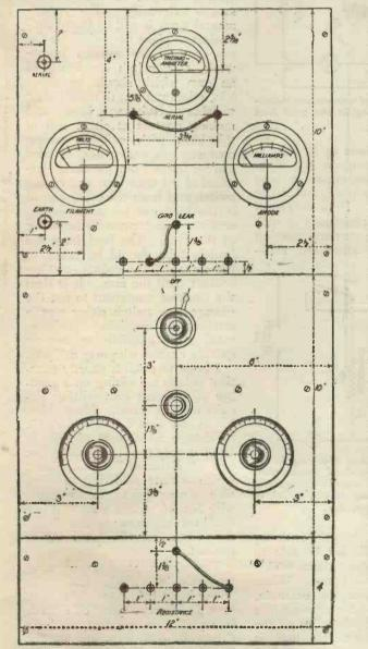
Fig. 1.-Dimensioned drawing of front of panel.
