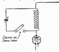
Fig. 4.—A suggested arrangement for cutting out the variable condenser in a tuned anode circuit.
