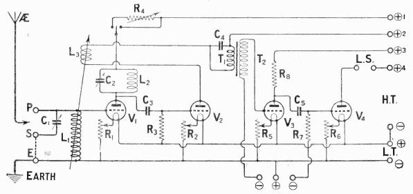
Fig. 4.—Showing the connections necessary when a two-valve amplifier is added, the last stage of L.F. being resistance coupled. 448
