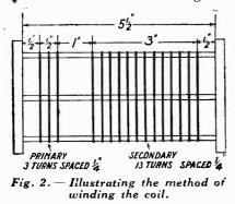
is seen the method of winding the primary and secondary coils, both of which are placed upon the same former. The primary consists of three turns of No. 18 s.w.g. wire with a spacing of  $\frac{1}{4}$  in. between turns. The secondary, which begins 1 in. away from the primary, has 13 turns of the same wire, also with  $\frac{1}{4}$  in. spacing between turns.
