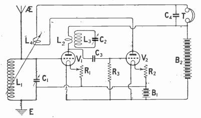
Fig. 4.- An even more selective circuit is obtained by the use of reaction.
