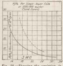
Fig. 10.—Showing the variation in R/Ro for single-layer coils at 1,000,000 cycles.
