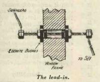
If the holes in the bushes are larger than 2 B.A. clearance, washers should be placed under each nut, the rod being arranged concentrically in the holes, and the nuts screwed up tightly. Two nuts are then placed on each end of the rod; the down-lead of the aerial is securely clamped between the two nuts on the outside, while the lead to the set is clamped between those on the inside.
