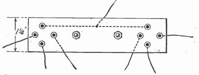
Fig. 2.—The ebonite strip showing how the flexible connections are made.
