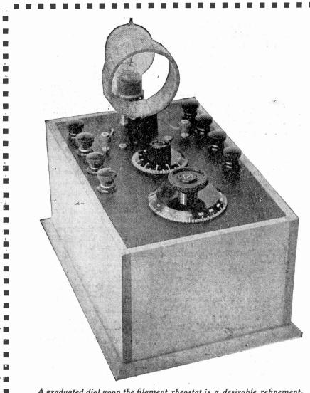
A graduated dial upon the filament rheostat is a desirable refinement.
