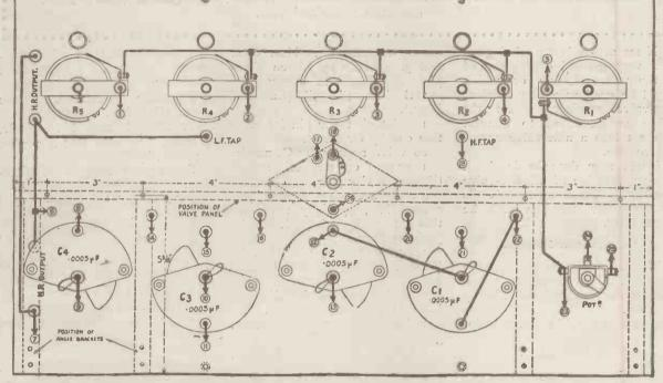
Fig. 2.—The wiring arrangements behind the main panel, which should be used in conjunction with the valve panel seen in Fig. 3. The numbers on this drawing indicate that these connections are continued to similar numbers on the valve panel. Blue print 94b.
