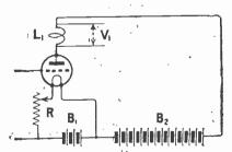
Fig. 2.—When H.F. potentials are applied to the grid the E.M.F.'s across L1 will be small.
