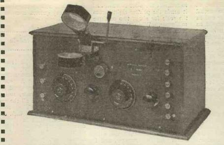
Fig. 1.—The handsome appearance of the receiver may be seen in this photograph. The novel form of crystal detector seen in the centre of the panel should be noted.
