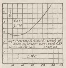
Fig. 7.—Curve produced when using a coil of 200 microhenries.
