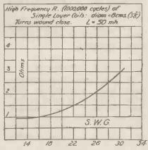
Fig. 5.—Showing the H.F. resistance of coils wound upon the same former with different gauges of wire to produce an inductance of 50 microhenries.
