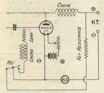
Fig. 3.—Method of connecting backload when keying in the grid leak lead.
