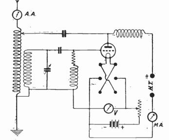
Fig. 3.—A typical transmitting circuit showing the positions of the meters.
