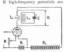
Fig. 3.—The impedance of L1 will rise when L2 C is tuned to the aerial circuit.
