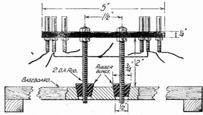
Fig. 1.-Constructional details of the value mounting.
