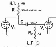
Fig. 2.—Details of the resistance coupling connections.
