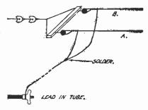
Fig. 3.—How the wire may be joined in a double wire aerial.
