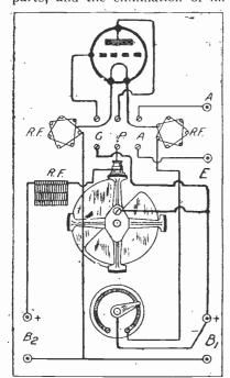
Fig. 1.—The back-of-panel layout of the 5-metre transmitter.
