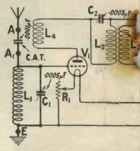
Fig. 2.- The theoretical circuit
