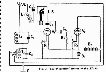
Fig. 1-The theoretical circuit of the ST150.
