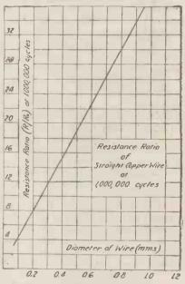
Fig. 3.—Curve of resistance ratios of straight copper wire plotted against diameter.
