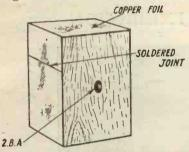
Fig. 1 shows details of the former on which the coil is wound.
