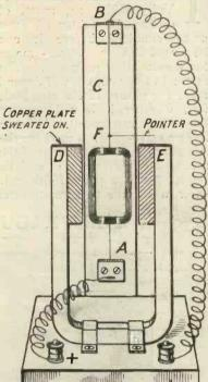
Fig. 2.—Illustrating how the component parts are arranged in the complete instrument.
