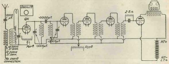
The essentials of the supersonic heterodyne receiver at 2DX. For simplicity the filament connections and L.T. batteries have been omitted.
