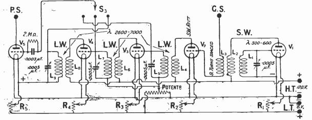
Fig. 6.—Theoretical circuit arrangement of the super-heterodyne unit.
