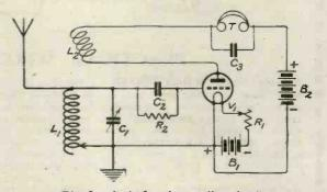
Fig. 2.—A single value reaction circuit.
