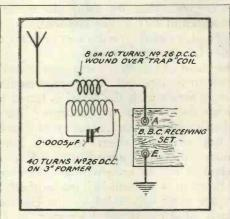
Fig. 2.—Type B filter. This consists of a similar oscillatory circuit coupled inductively to a coil placed in series with the aerial lead. In the case of a B.B.C. receiver this coil should consist of a very few turns tightly coupled to the trap coil.
