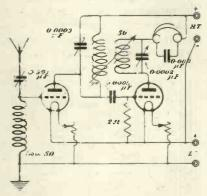
Fig 2.—Method of controlling reaction by a variable condenser shunted across the reaction coil. Numbers indicate suitable sizes of Igranic coils for broadcast reception.
