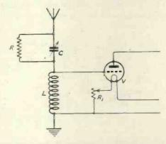
Fig. 4.—Illustrating the position of the static leak in relation to the aerial circuit.
