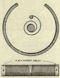
Fig. 13.—Illustrating arrangement of the resistance element.
