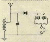
It is regretted that last week's diagram illustrating "A Home-made Potentiometer" contained an error, in that the aerial circuit was not tunable. We reproduce a corrected circuit diagram herewith.
