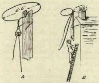
Fig. 19.—Method of lifting loop over chimney.
