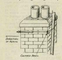
Fig. 16.—Method of fixing pole.
