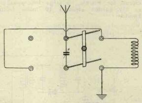
J. G. (WATFORD) asks for the correct connections of a series-parallel switch.
