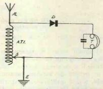
Fig. 5.—A simple crystal receiver circuit.
