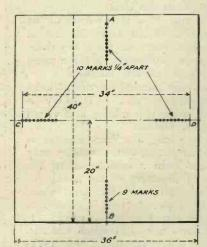
Fig. 1.—Dimensions of the holland foundation.
