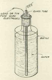
Fig. 8 .- The completed resistance.
