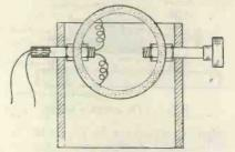
Fig. 6.—Suggestion for inner coil connections of a vario-coupler.
