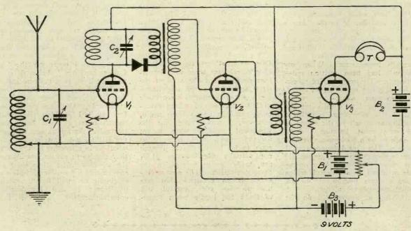
Fig. 1.—A method of obtaining exact adjustment of grid potential.
