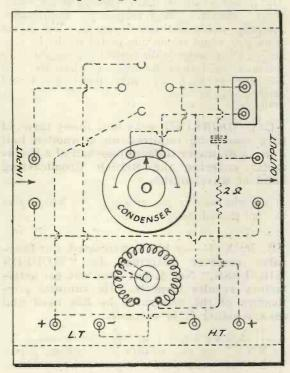
We give herewith a sketch showing how a suitable amplifier may be assembled. You will require the following :-
