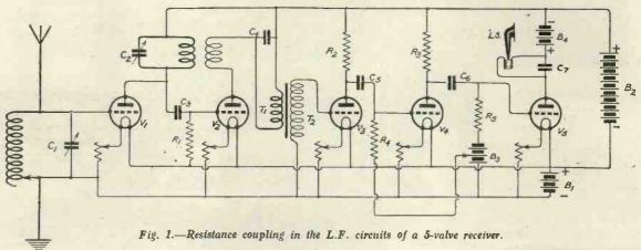
quency side of the circuit. The secondary  $T_2$  is connected across the grid and filament of the third valve, in the anode circuit of which is an anode resistance  $R_2$  having a value of about 50,000 to 70,000 ohms. The anode of the third valve is connected through the grid condenser  $C_3$  to the grid of the fourth valve, the condenser  $C_5$  having a capacity of about 0.005  $\mu F$ ; the gridleaks  $R_4$  and  $R_5$  have a value of about 2 megohms.
