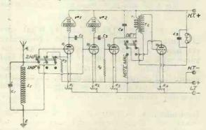
The arrangement you indicate should ensure satisfactory results, but the condensers coupling the anode coils are much too large. These should have a value not greater than 0.00025 µF, and be arranged as shown in diagram above.
