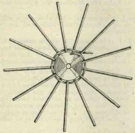
J. H. (SUNDERLAND) proposes to wind a set of 6 basket coils on cardboard formers having an internal diameter of lin. with No. 28 standard wire gauge double cotton covered wire. He asks how many turns will be necessary on the various coils to produce a set to cover a range of from 100 to 1,500 metres.
