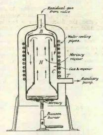
Fig. 4.—Principle of Langmuir pump, Mercury vapour "wind" blows residual gas before it, vapour afterwards condensing.
