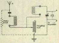
Fig. 3.—Diagram of the tuner showing one of the inductances in each circuit.
