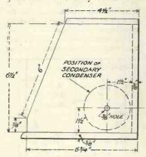
Fig. 3.—Dimensions of side of containing box
