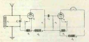
Fig. 3.—A theoretical circuit explain ng -esistance capacity coupling.
