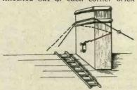
Fig. 18.—Using chimney ledge as anchorage for aerial.
