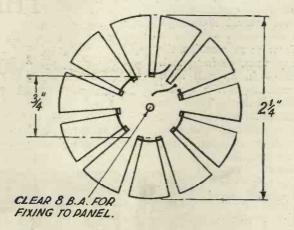
Fig. 3.-Former for the fixed basket coil.
