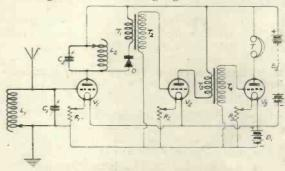
Fig. 2.—A three-valve tuned anode receiver employing a crystal detector.
