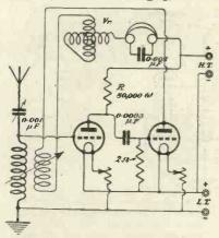
Fig. 4.—Another good ctrcuit for longwave telephony. Intervalve coupling is provided by resistance R, white the variometer Vr controls the reaction.
