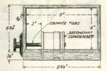
Fig. 4.—Arrangement for fitting the secondary condenser.
