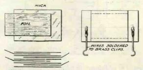
METHOD OF ASSEMBLING COMPLETE CONDENSER.
