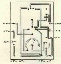
Fig. 3.-Wiring of Panel.
