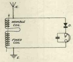
Fig. 15 .- Circuit diagram of receiver with variometer.
