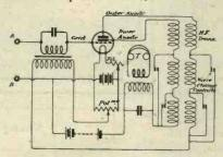
Fig. 2.—Diagram of the circuit arrangements of the amplifier.
