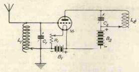
Fig. 3 .- A simple amplifier circuit without reaction.
