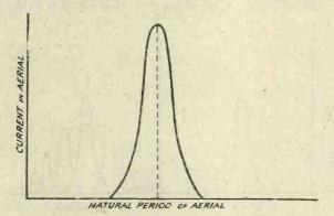
Fig. 1.—Showing the effect of aerial resistance on an imposed H.F. current.
