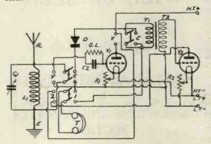
A valve and crystal circuit with alternative switching arrangements.
