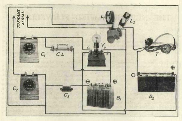
Fig. 2 .- A pictorial wiring diagram of the new circuit.
