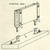
Fig. 12.—An interchangeable mounting for the condensers.
