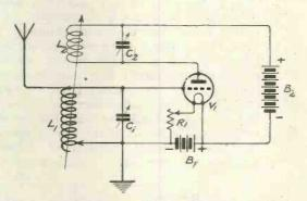
Fig. 4.—Showing how reaction is obtained by coupling anode and grid coils.
