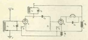
Fig. 1 .- "Tuned anode" H.F. coupling.
