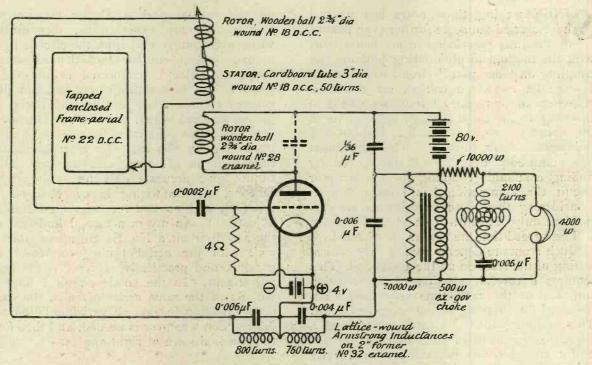
Fig. 2.-Circuit diagram of the portable receiver.
