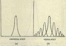
Fig. 3.—The form of emitted H.F. waves when speech is applied.
