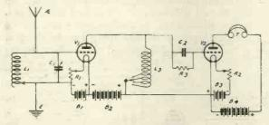
Fig. 1.—Theoretical circuit illustrating reactance-capacity coupling.
