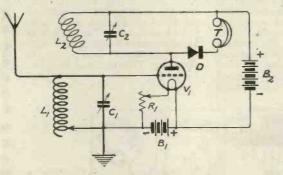
Fig. 1.-A simple valve-crystal receiver with reaction.
