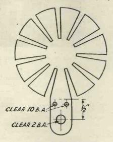
Fig. 4.—Former for the moving coils.
