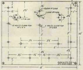
Fig. 2.—Plan of the panel.
