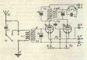
We give herewith a suitable circuit diagram for your purpose, showing how a two-valve receiver may be arranged in the most efficient manner. The values
