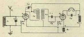
Fig. 3:-A tuned transformer coupling.
