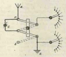
Fig. 10.—Switch to enable one condenser to be used in series or parallel.
