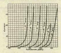
Fig. 2.—Showing the rapid increase in the emission from sodium with rise of temperature (Richardson).
