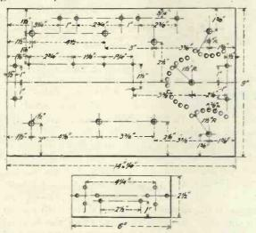
Fig. 4.—Showing dimensions and drill sizes of main and valve panels.
