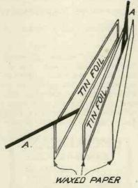
Fig. 9.—The assembly of the foils.
