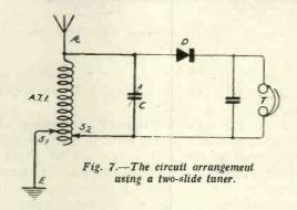
A simple form of tubular condenser may readily be made from a cylindrical lamp glass or test tube coated with tinfoil on the outer side, whilst a metal tube or a tinfoil-coated wooden rod is arranged to slide inside it.
