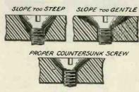
Fig. 7.—Illustrating correct and incorrect countersinks.
