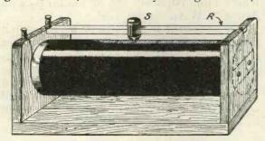
Fig. 1.—A "single slide" tuning inductance.
