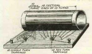
Fig. 8.—A tuning inductance with multiple and submultiple tappings.
