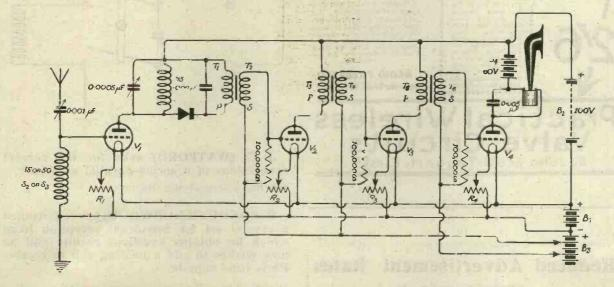
for Igranic and Burndept coils are shown in the figure, together with condenser, battery, and resistance values. The battery  $B_a$  may be variable up to 9 volts.
