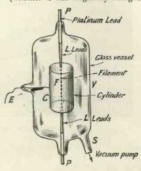
Fig. 2.—Simple arrangement for studying emission from a wire under various conditions.
