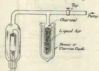
Fig. 3 .- Illustrating the method of employing charcoal cooled by liquid air, for absorbing the residual gas which cannot be removed by pump.
