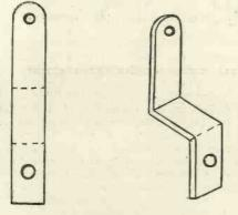
Fig. 5.—Showing how to bend the clips.
