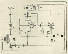
Fig. 1.—The ST75 circuit showing the position of the extra resistance  $R_4$ .
