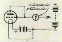
Fig. 2.—Simple method of determining characteristic curve of valve
