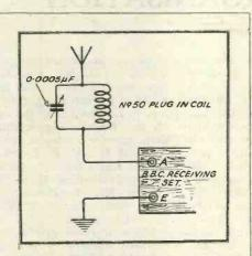
Fig. 1.—Type A wave-filter—a simple oscillatory circuit connected in series with the aerial lead. When this circuit is tuned to the interfering wave, it will act as a trap for this wave and will very largely reduce the jamming.
