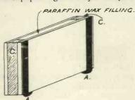
Fig. 10.-Finished condenser.
