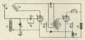
Fig. 3.—The addition of low-frequency amplification to the circuit of fig. 2.
