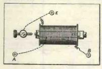
Fig. 2.—Showing connections of buzzer.
