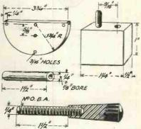
Fig. 5.- Components for coil mounting.
