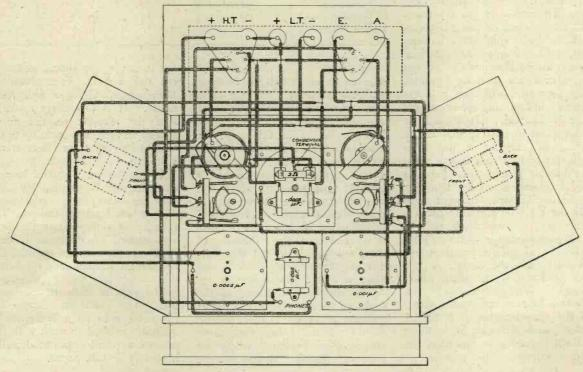
Wiring diagram of the cabinet set For clearness the sides and top of the cabinet have been drawn as if they were opened out. The letters "B" and "F" by the tabs of the anti-capacity switches indicate "back" and "front" respectively. One terminal of the central variable condenser happens to come immediately beneath the gridleak. Where wires join, the tubing is cut away to allow soldering.
