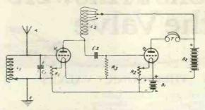
Fig. 2.—A practical application of reactance-capacity coupling.
