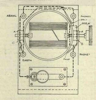
Fig. 1.—Underside of baseboard showing wiring.
