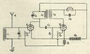
Fig. 4.—A circuit employing the approved type of reaction.
