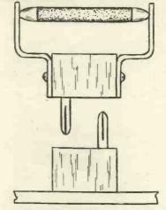
Fig. 4.-Method of mounting anode resistances.
