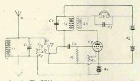
Fig. 1.—The ST34 circuit with the first valve removed.
