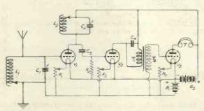
Fig. 1.—A three-valve tuned anode receiving circuit.
