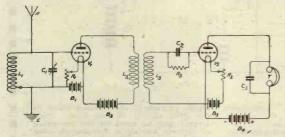
Fig. 1.—Two valves coupled by an aperiodic transformer.
