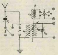
Fig. 6.—Circuit diagram of the tuner.
