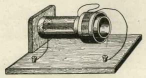
Fig. 14 .- An easily constructed but efficient variometer.
