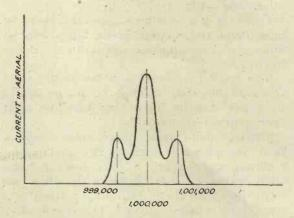
Fig. 2.—What happens when a steady low frequency is imposed on a H.F. current.
