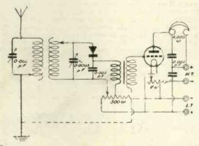
Coil L<sub>1</sub> might have 35 turns of No. 20 s.w.g. wire wound on a 3 in. tube. Coil  $L_2$  should have 50 turns of similar wire. The value of C1 might be 0.0015  $\mu$ F and C2 0.002  $\mu$ F. High resistance telephones may, of course, be used in place of a telephone transformer, as shown above.
