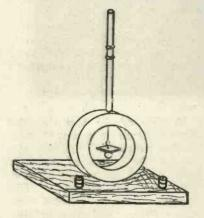
Fig. 1.—Illustrating principle of electromagnetic ammeters and vollmeters.
