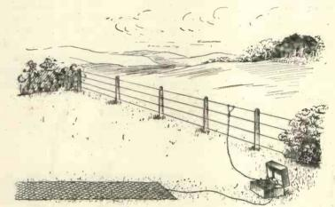
Fig: 2.-Using a fence as an aerfal.
