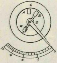
Fig. 2.—Principle of "moving-iron" instrument, "gravity control."
