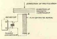
Fig. 2.—Illustrating phase-effect in a frame edge-on to advancing waves.
