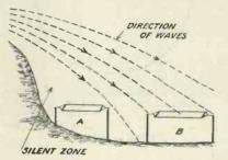
Fig. 3.—Shielding effect of high ground. Aerial A is in silent zone. Position B should be at distance from A equal to about 5 times the height of the mountain or hill.
