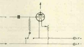
Your reaction coil appears to be much too large. The coupling with the anode coil should be just sufficient to raise signal strength to the maximum, and no more. Instead of connecting your gridleak as shown, one end of it should be attached to the positive filament leg. This will still further decrease any tendency to oscillate.
