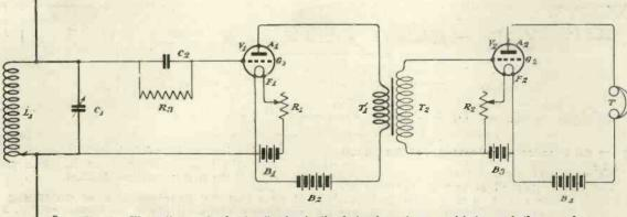
Fig. 1.—Illustrating a simple circuit wherein the first valve acts as a detector and the second as a low-frequency amplifier.
