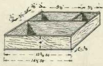
Fig. 11.—Delails of the containing box.
