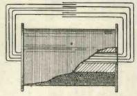
Fig. 2.—Showing the core and bobbin of the transformer.
