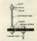
Fig. 5.—Details of vertical clip.
