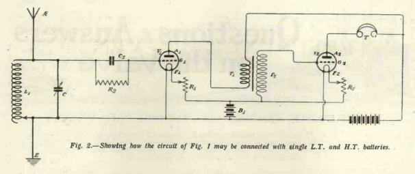
duce low-frequency current variations through  $T_1$ . These current variations are stepped-up by the transformer  $T_1$   $T_2$ , and variations of higher voltage are impressed on the grid of the second valve, which amplifies them, the magnified current flowing through the telephones T.
