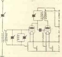
Fig. 8.—Circuit with rejector arrangement.
