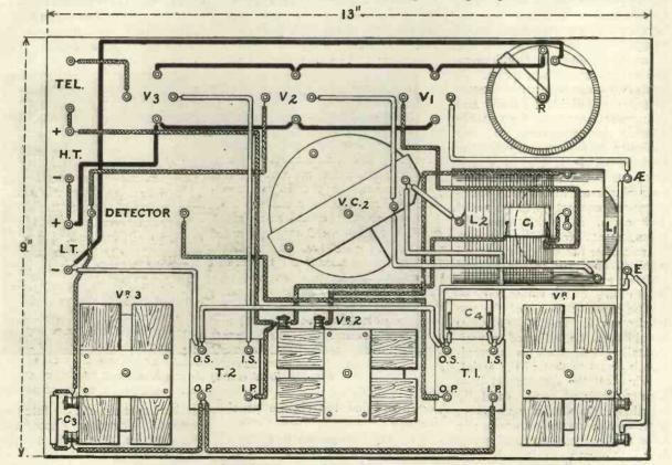
Fig. 12 .- A complete back-of-panel wiring diagram.
