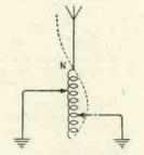
Fig. 1.—Potential nodes in aerial system.
