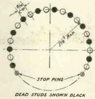
Fig. 11.—Suggested method for fitting studs.
