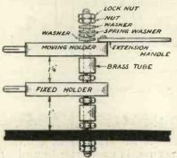
Fig. 9.—The arrangement of spindle.
