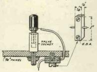
Fig. 5.-Selector plug and socket.
