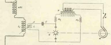
Fig. 1.—Theoretical circuit diagram of damped-wave or "spark" transmitter.
