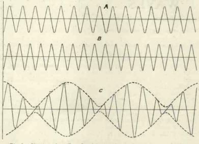
Fig. 2.—Showing "beals" produced by interference between waves of slightly different frequencies.
