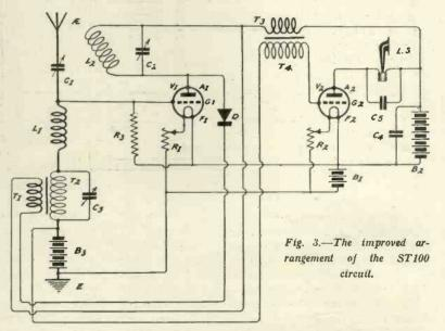
was found to be Galena, with a fine metal point resting on it. The importance of the detector not only lies in its actual rectifying properties, but also on its impedance.  $R_1$  and  $R_2$  are of standard pattern. The inductance  $L_1$  may be a coil of 70 turns of No. 24 double cotton-covered wire, wound on a (Continued on page 772.)
