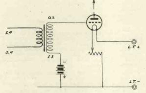
high-frequency current is allowed to pass through it, and for this reason a large condenser will provide a more ready by-path. There is no reason for a condenser across the second transformer, as all the high-frequency current (if any) will have passed through the first. It is, however, an advantage to shunt the telephone with a large fixed condenser, as this sometimes controls reaction effects and increases signal strength.
