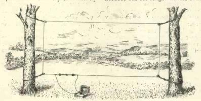
Fig. 7.-Using a large loop aerial.
