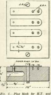
Fig. 6.—Plug block for H.T. and L.T. connections.
