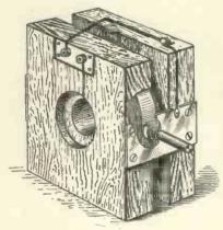
Fig. 6.—A completed variometer.
