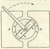
Fig. 4.—Showing the moving coil.
