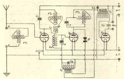
Fig. 4.-The circuit of the receiver.
