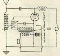
Fig. 2.-Illustrating grid control.
