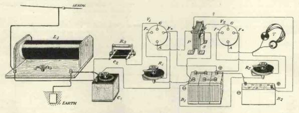
Fig. 3.-A pictorial arrangement of the circuit in Fig. 2.
