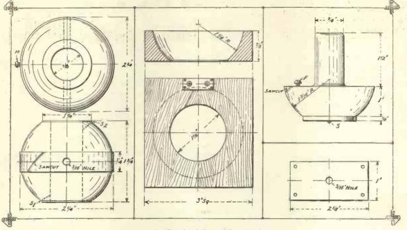
Fig. 5.-Details of the aerial variometer.
