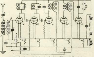
Fig. 2.-One method of using the three-slider potentiometer.
