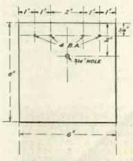
Fig. 7.-The layout of the panel.
