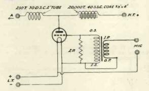
Microphone transformer: core §in. diameter × 4in. tron wire.
