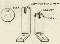
Fig. 6.—The parts of the detector ready for mounting.
