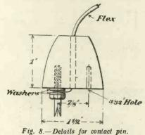
used with great advantage to see that nothing is wrong with the battery connections. Plug its pins into the filament legs of the valve holder. If a mistake has been made—and it is easy to do so in an absent-minded moment—it is better to sacrifice a sixpenny flashlamp bulb than a fifteen-shilling valve. R. W. II.
