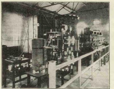
Continuous wave transmitter, showing, from left to right: (1) high-speed signalling relays; (2) independent drive; (3) rectifier and oscillator valve panel.
