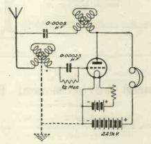
We give above a novel circuit for which good results are claimed in America. If an earth connection is used with the aerial it should be connected as indi-
