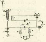
Fig. 1.—Circuit diagram of typical CW transmitter.
