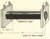
Fig. 1.—The bobbin and core of the transformer.
