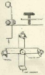
Fig. 9.—A suggestion for crystalcrystal combination.
