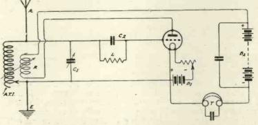
Fig. 4.-Circuit diagram of modern self-oscillating valve receiver.
