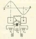
Fig. 4.—Principle of the Weagant arrangement.
