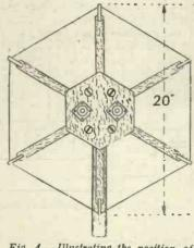
Fig. 4.—Illustrating the position of the arms.
