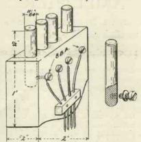
Fig. 11.—Details of the 4-pin plug.
