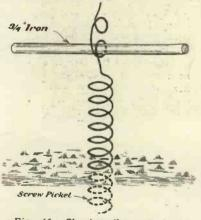
Fig. 11.—Showing the method of using a screw picket
