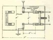
Fig. 6.—A double-pole earthing switch.
