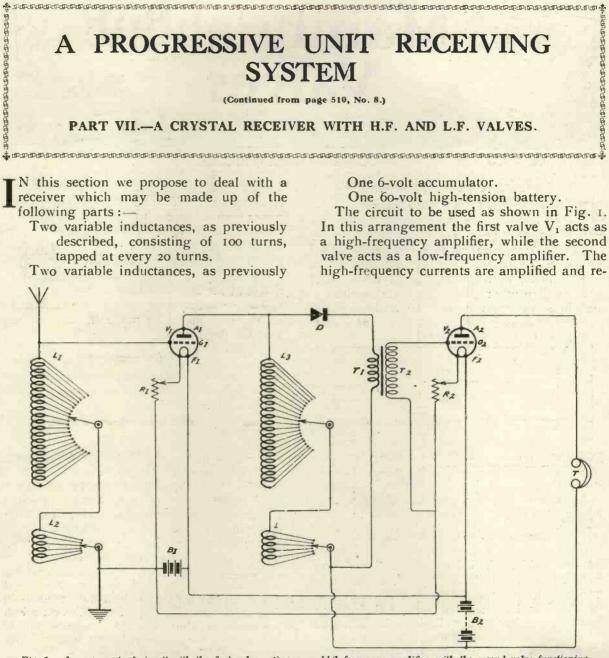
Fig. 1.—Arrangement of circuit with the first valve acting as a high-frequency amplifier, with the second valve functioning as a low-frequency amplifier.
