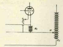
Fig. 2.—Method showing how the H.T. ballery may be used for providing negative potential to the grid.
