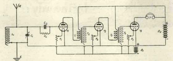
Fig 2 .- A valve detector followed by two stages of L.F. amplification.
