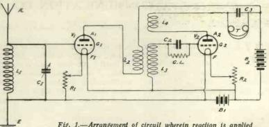
Fig. 1.—Arrangement of circuil wherein reaction is applied to the secondary of an untuned H.F. transformer.
