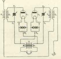
Fig. 2.—Circuit arranged to eliminate interference.
