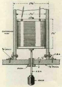
Fig. 4.—Illustrating the sliding reaction coil.
