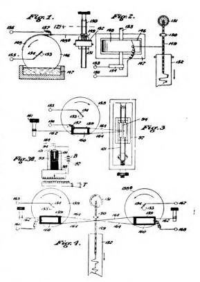
gram of an amplifier or relay. Fig. 4 is a similar view of a modified form in which pressure effects are balanced and operate differentially to produce **a** more sensitive instrument.
