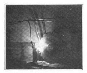
Siasconset's spark. This photograph was made with a 5 sec. exposure while the disc was running at 1800 R. P. M. Although traveling at a speed of more than 100 miles an hour, the studs appear to be standing still, due to the fact that the disc was illuminated only at the instant when the moving stud came opposite the stationary stud, causing the spark to disclarge
