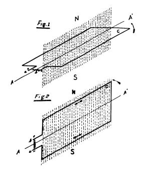
maximum speed. In this case b will be *plus* (Positive) and a *minus* (Negative). If a and b are connected together so a current can flow, it will flow from b to a indicated by the arrow along side the loop. The E. M. F. has passed through all values from zero to its maximum, that is, the E. M. F. has had a different value for every change in position of the loop. These values are called instantaneous values, and will be discussed later.
