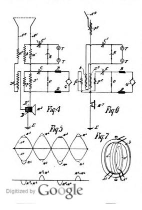
conductors, which, as is common in the art, may consist of one or several wires. These may be independent of each other, or, and as indicated by the dotted line  $3^3$ , they may be different legs of the same loop antenna. These conductors are both grounded, as, for instance, at E.
