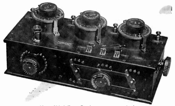
Marconi Multiple Tuner. For adjusting to partous wave lengths.
