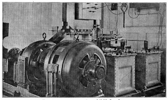
Transmitting Apparatus at Suva-5-K.W. Disc Set.
