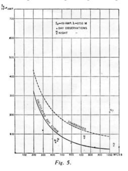
for very distant stations. It is seen that for good communication at a distance of 2,500 miles not less than 240 ampères must be used at a wave length of 6,000 metres, though onefourth of this would be audible.
