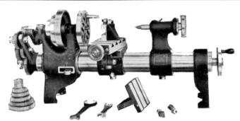
4 in. S S. Boring and Milling Lathe.
