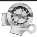
GARDNER BALL-BEARING JOINT OF L. C. SMITH & BROS.' TYPEWRITER.
