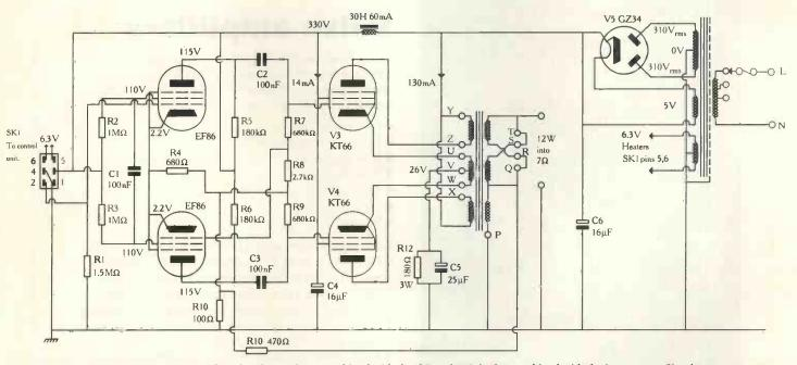
Fig. 4. The Quad II is different. Not only is the phase splitter combined with the driver, but it is also combined with the input stage. Circuit courtesy Quad Electroacoustics.
