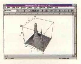
Fig. 11. In a three-dimensional plot such as this, peaks in the surface correspond to poles and depression to zero level corresponds to a zero. Plots of this type are useful for visualising the poles and zeros of a circuit.
