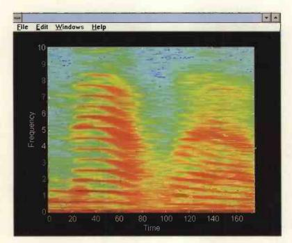
Fig. 6. Spectrogram of the word matlab. The function specgram can be used with great effect to analyse speech signals.
