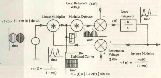
Fig. 1. Amplitude-locked loop consists of a linear multiplier, modulus detector and a high gain integrator. When the loop is closed, envelope variations of the carrier are reduced to insignificant proportions due to servo action and an error signal called the inverse modulus is produced.
