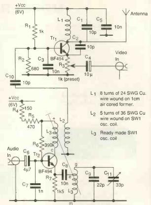
Using a short-wave coil for the 5.5MHz oscillator greatly simplifies the transmitter's design.
