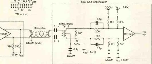
Circuits to isolate or break the path between instruments and host computer to avoid ground currents interfering with analogue equipment.
