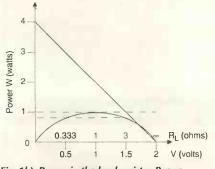
Fig. 1 b). Power in the load resistor  $R_l$  as a function of its value, when  $R_s$  equals the design system impedance of  $1\Omega$  (curve) and total power supplied by the generator (sloping line).
