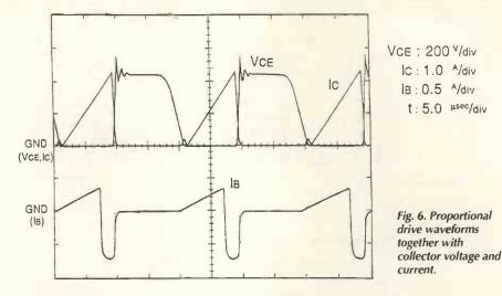
conventional pwm flyback converters - leakage inductance causes overvoltage, and primary capacitance causes overcurrent.
