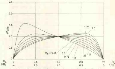
Fig. 3. Power in the load resistor R<sub>1</sub> as a function of its value, showing curves for several different values of Rs. Source emf ESOURCE adjusted to give 1W into a 1 $\Omega$  load resistor R<sub>L</sub> for each value of R<sub>s</sub>.
