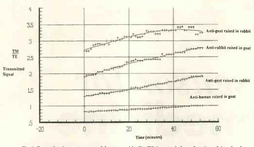
Fig. 2. Transmitted output power of the waveguide (TM/TE) is recorded as a function of time for the following sequence of antibodies bound to the waveguide – a) anti-human raised in goat, b) anti-goat raised in rabbit, c) anti-rabbit raised in goat and d) anti-goat raised in rabbit. As each subsequent layer binds to the preceding layer the transmitted output power is observed to rise in each case.
