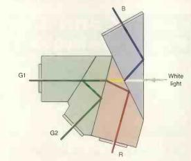
ccds are assigned to green light, with other two being used for red and blue as normal. Putting more emphasis on the resolution of the green signal improves efficiency and makes the system compatible with the human eye which has a much greater sensitivity to luminance signals than chroma signals: 70% of hdtv luminance signals come from the green component.
