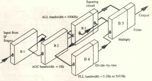
Fig. 2. ALL-PLL amplitude demodulator. The amplitude-locked loop alternates between in-lock and out-of-lock for strong and weak carrier signals. The PLL captures the carrier phase quickly but releases it slowly. A highly stable carrier is generated.
