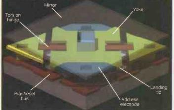
Details of the digital micromirror device. 500,000 mirrors – each hinged and capable of rotating independently under digital control – make up a display measuring just 1.5 by 1cm. Pictures courtesy TI.
