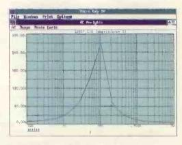
Fig. 5. Output noise analysis of the filter of Fig 1 shows a strong peak at 10kHz.
