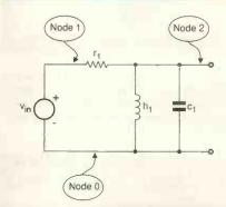
Fig. 9. Poles and zeros of this band-pass filter are analysed by a Nodal routine in Fig. 10.
