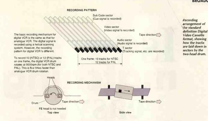
DVCPRO differs in using more robust metal particle tape, which is run at double speed to increase track pitch to 18 $\mu$ m, and the addition of a control track and cue channel. The HD version uses metal-evaporated ME tape run at double speed to record twenty 10 $\mu$ m tracks per frame. Horizontal resolution is about 500 lines for SD – 25% greater than Hi8/S-VHS – and 600 lines for HD, with double the vertical resolution.
