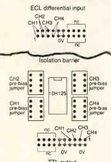
used here having low capacitive inter-winding coupling with good inductive coupling at the frequencies of interest. Since the transformer cannot couple signals of less than 100kHz, with pulse widths of more than a few microseconds, a pre-biasing circuit is needed to define the output during steadystate periods by means of jumper settings.
