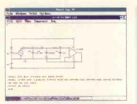
Fig. 1. Typical schematic drawn with Micro-Cap IV includes definitions of models and optional command statements for the analysis.
