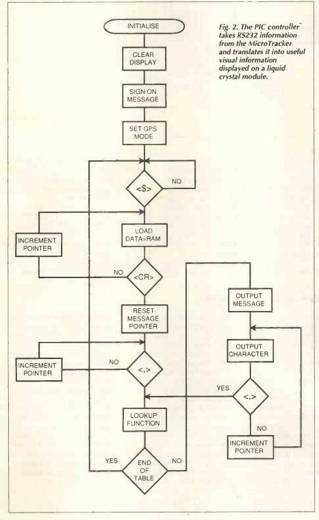
$2C_{16}$  is identified – field delimiter, the message type is then determined from a lookup table and sent to the liquid-crystal display. Additional text messages are sent prior to the received information to clarify to the user what is being displayed.
