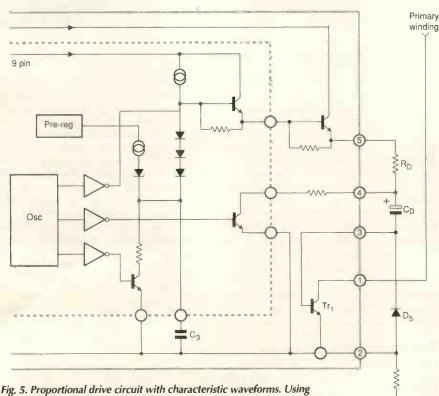
proportional drive helps the power supply cater for a wide load range. In the upper waveform diagram, IB1(peak)=(V9pin-3)/RD
