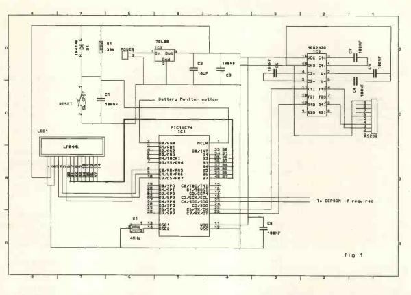
characters respectively and are interfaced in the 8-bit mode with full handshaking. This method of interfacing provides the fastest display update times but uses eleven i/o lines. If this design is transported to a 28-pin 16C73 then the 4bit write only approach can be taken with the display using only six i/o lines.
