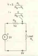
Fig. 1a). Normalised source and load, illustrating the maximum power theorem.
