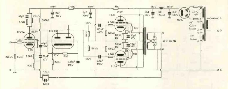
Fig. 2. Mullard's 5-20 was an ultra-linear design with high sensitivity but poor noise performance due to the input being pentode, rather than triode, based. Circuit courtesy Philips Components Ltd.
