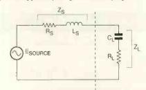
Fig. 1c). In the ac case, source and load reactance must be taken into account. Source to the left of the dotted line, load to the right.
