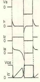
Fig. 7. Conventional ringing-choke convertor drive circuit with waveforms.
