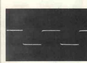
Response of the preamplifier subjected to a 5kHz squarewave at 6V pk-pk amplitude. Output loading was the quasi-standard of  $50k\Omega$ .
