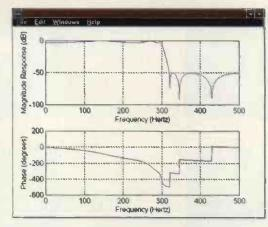
Fig. 2. Transfer function generated graphically in the digital z domain.
