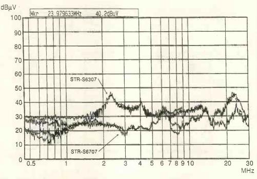
Fig. 10. Comparison of conducted EMI - ringing choke versus quasi-resonant techniques.
