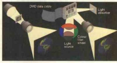
Conventional projector, left, and a projection system incorporating the digital micromirror device, right. In the DMD system, light from the source passes through a colour wheel and is reflected to both the projection lens and to the light absorber on the right. Picture courtesy Texas Instruments.
