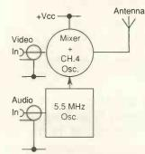
Only two transistors are needed to transmit both audio and video on vhf channel 4.
