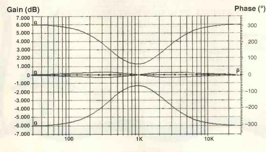
Simulation of boost and cut curves with the preamplifier's tone controls set flat and at maximum and minimum. Centre curves show phase shift. Measured results tally.
