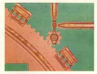
Close up of the output gear of Sandia's microengine.
