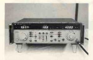
Solid State Microwave Signal Generators 2.3-13 GHz Freq' Range Wideband FM for satellite AM/FM & pulse modulation Built in pulse generator Options 001/003 fitted
