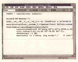
Fig. 10. This Mathematica-based sensitivity analysis of the filter in Fig 11 is adaptable to a wide range of circuits.
